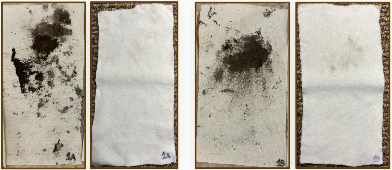
FIG 2. TEXTILE SAMPLE SOILED WITH DIRT BEFORE (LEFT IN EACH PAIR) AND AFTER (RIGHT IN EACH PAIR) CLEANING. THE PAIR ON THE LEFT WAS CLEANED USING THE FULLONICA METHOD; THE PAIR ON THE RIGHT WAS CLEANED USING CASTILE SOAP. PHOTOS BY KAIRA SHLIPAK
