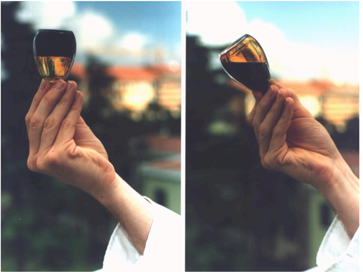
FIG 5. REPRODUCTION OF THE 'BLOOD' OF ST. JANUARIUS (THIXOTROPIC MIXTURE). PHOTO BY LUIGI GARLASCHELLI
