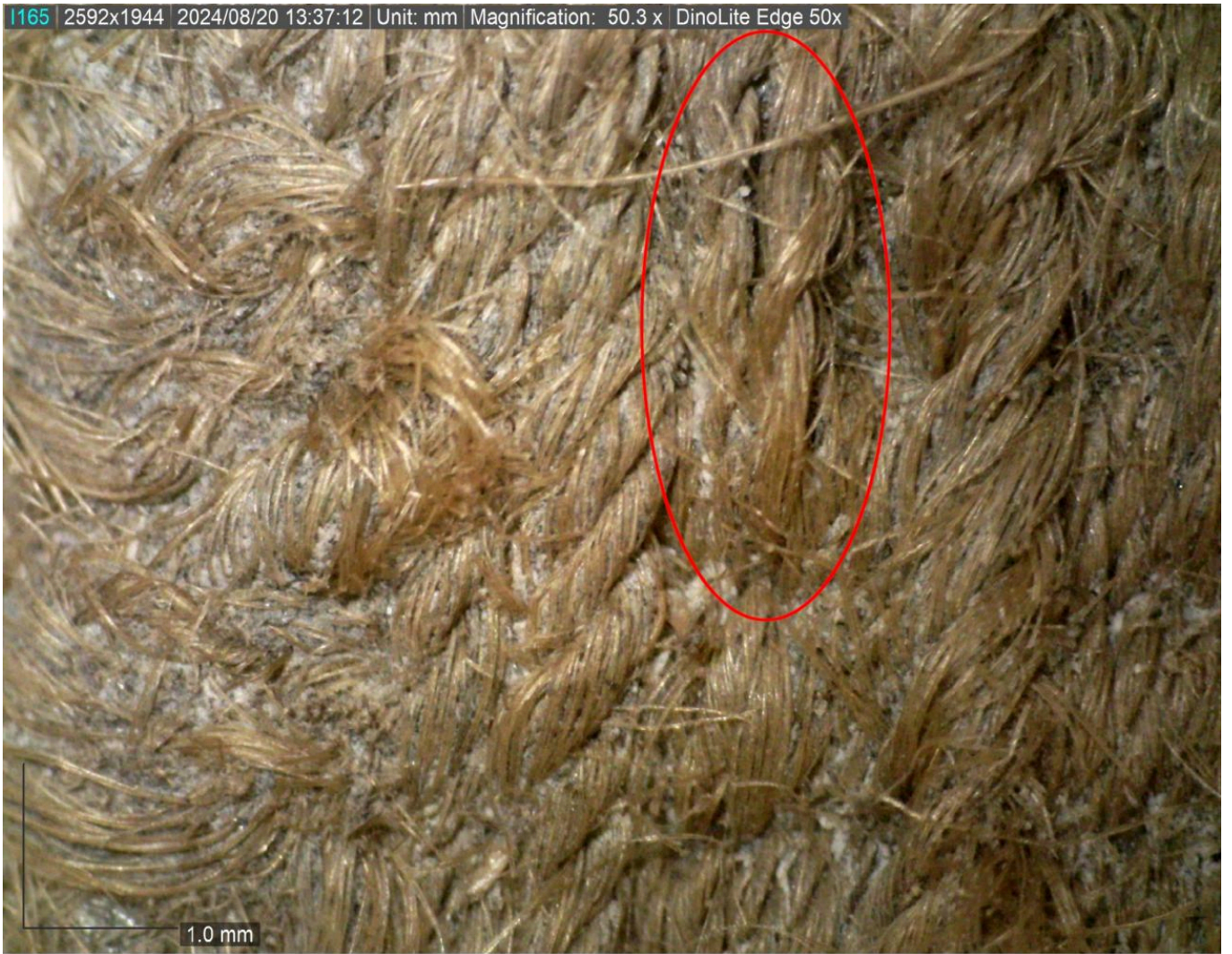
FIG 4. MISTAKENLY FLOATING THREADS IN HALLTEX 390B CIRCLED IN RED. PHOTO BY KAYLEIGH SAUNDERSON, DINOLITE DIGITAL MICROSCOPE
