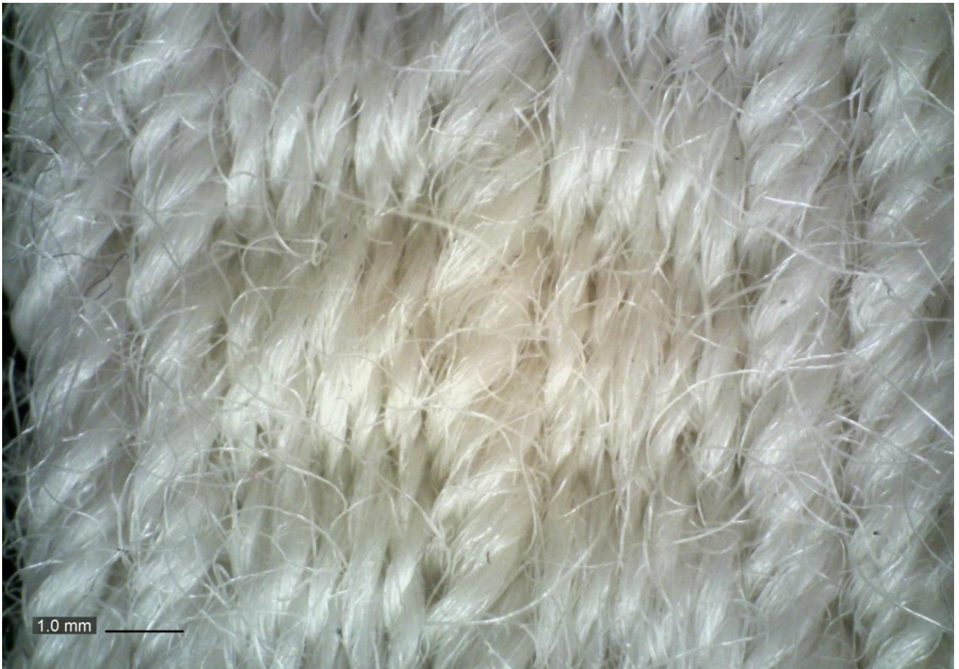
FIG 10. DETAIL OF THE RESULT COMBINING HEDDLE AND TABLET WEAVING (DINOLITE DIGITAL MICROSCOPE, 30X MAGNIFICATION, PHOTO BY KAYLEIGH SAUNDERSON)
