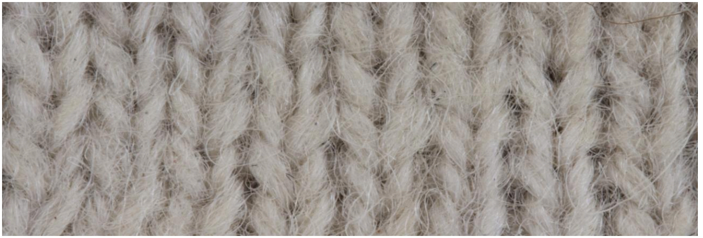
FIG 6. THIS SAMPLE IS KNITTED WITH MODERN KNITTING WOOL; THE YARN IS 2-PLY, BUT IT IS LOOSELY PLYED, AND THE DIVISION BETWEEN THE PLYED STRANDS IS HARD TO SEE. THE YARN FOR THE SAMPLES, WITH APPROXIMATELY THE SAME DIAMETER (THICKNESS), WAS SPUN AND PLYED WITH A STRONGER TWIST FOR A BETTER APPROXIMATION OF WHAT IS SEEN IN THE ARCHAEOLOGICAL MATERIAL. ALL SAMPLES WERE SPUN AND KNITTED BY THE AUTHOR AND PHOTOGRAPHED BY LETJA FEIS
