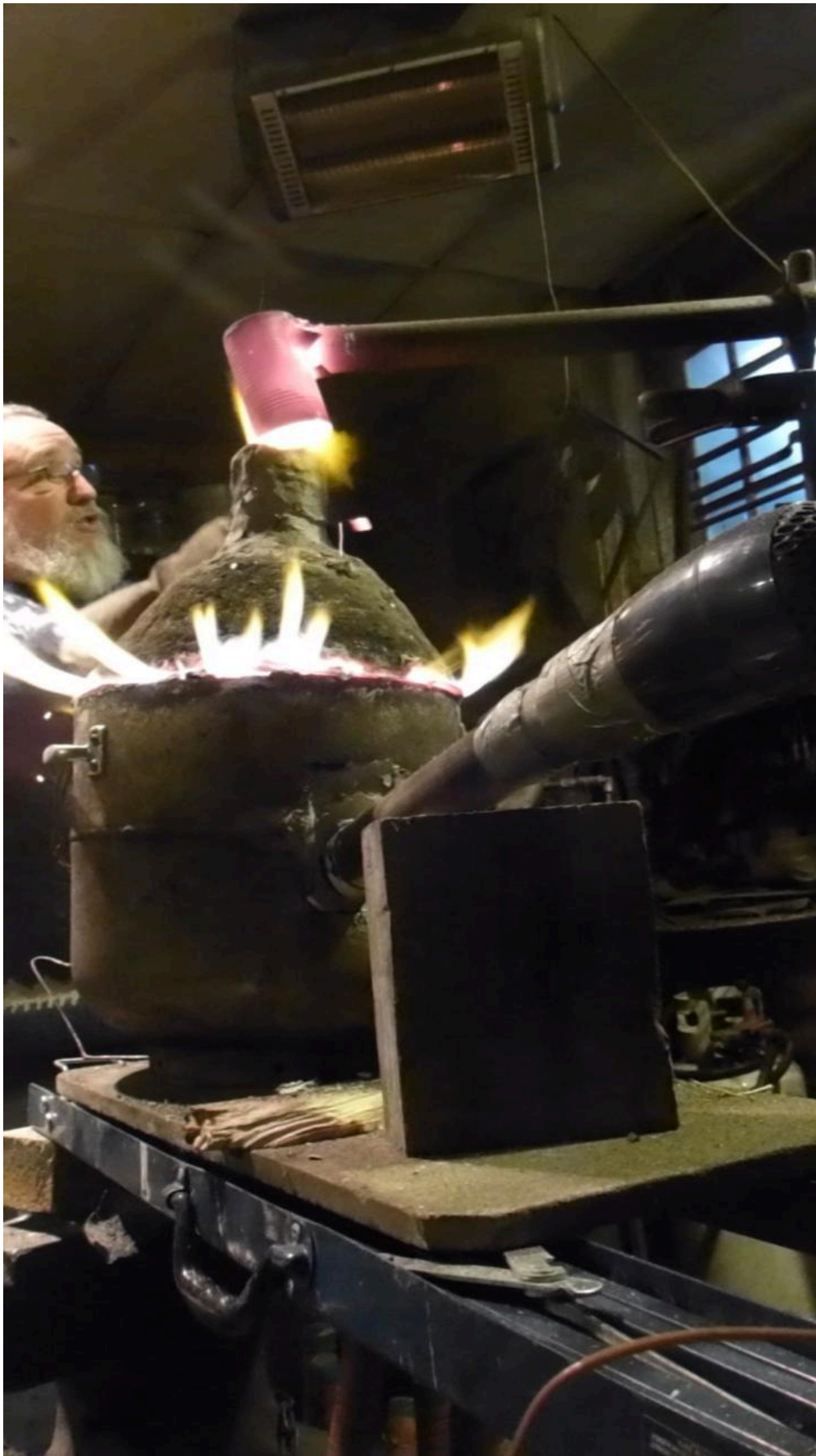
FIG 8. ADDING A CHIMNEY TO CAPTURE ASH
