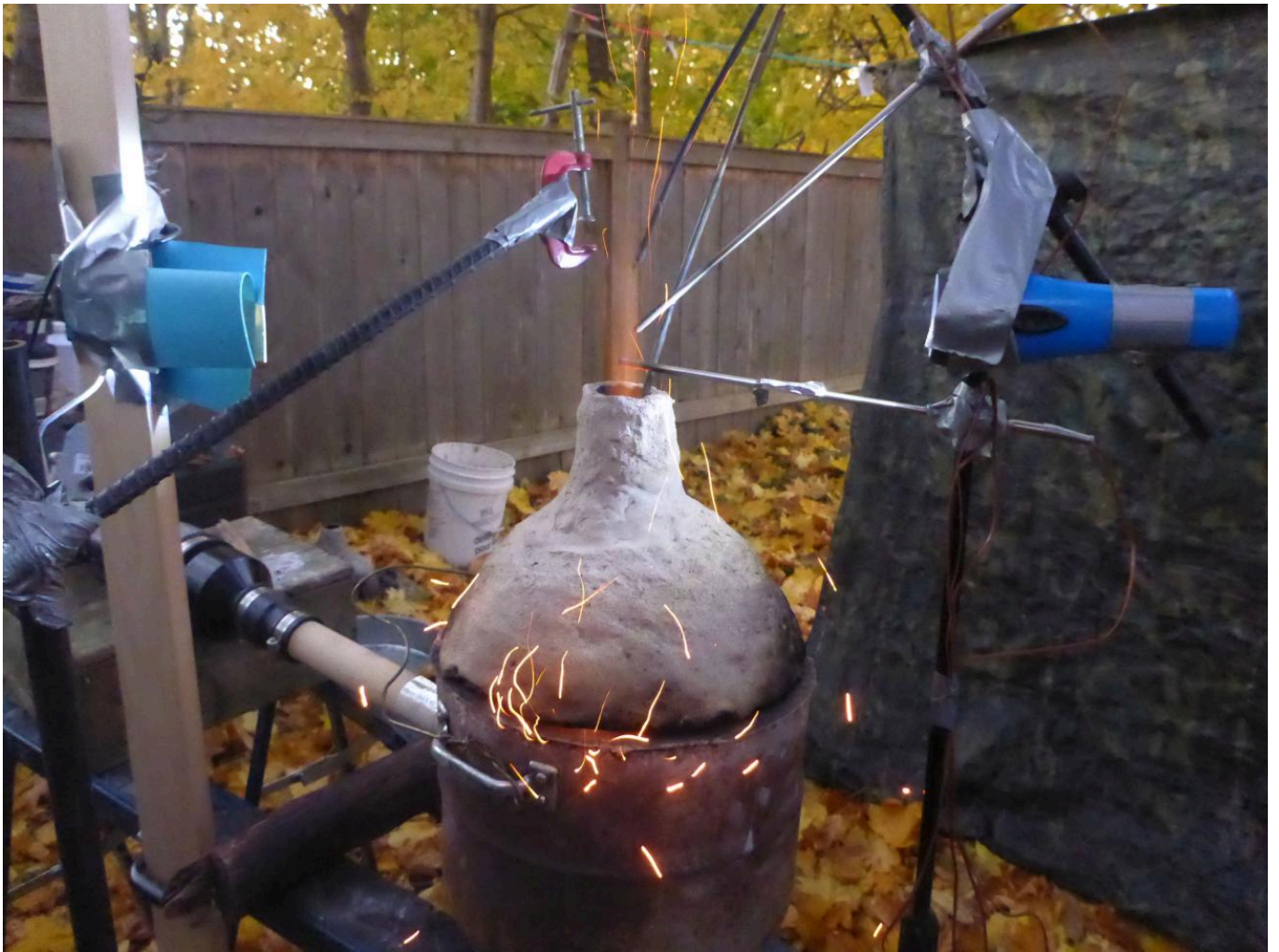
FIG 2. PILOT EXPERIMENT SETUP. LIGHT SOURCE AND THERMOCOUPLES ON THE RIGHT, LIGHT SENSORS ON THE LEFT. IN THE FOREGROUND IS THE CLAMP FOR THE CERAMIC PLATES.
