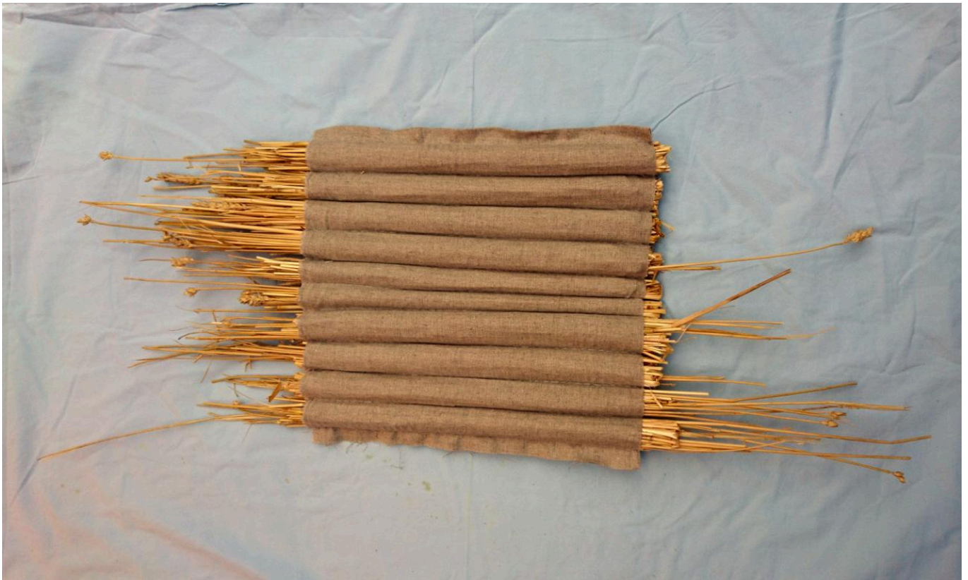
FIG 3. THE THATCHING STRAW IS STUFFED INTO THE LINEN AS SEEN IN VAQUERO SADDLES. PHOTO BY MOIRA WATSON
