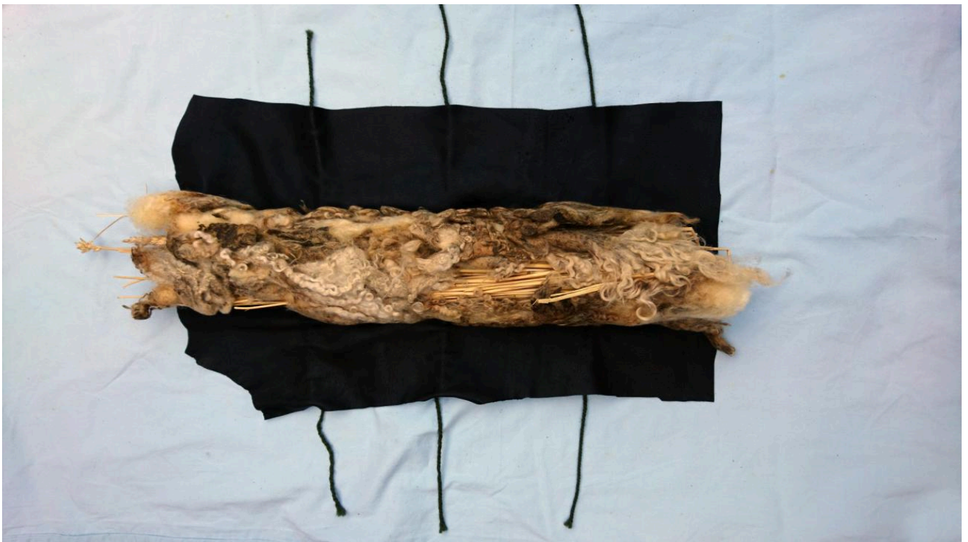
FIG 4. THE THATCHING STRAW WRAPPED IN UNWASHED FLEECE, TIED INSIDE (DYED) DEERSKIN TO TEST THE EFFECTS OF LANOLIN ON THE STRAW. AFTER THREE WEEKS, THE STRAW HAD NOT BEEN SOFTENED BY BEING WRAPPED IN THE FLEECE. PHOTO BY MOIRA WATSON
