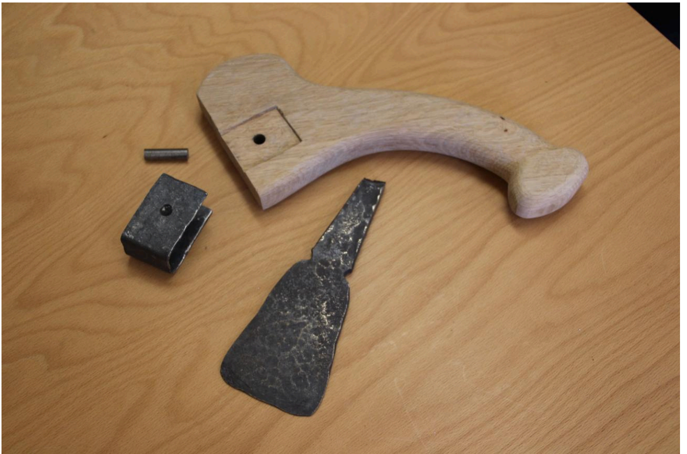
FIG 9. COMPONENTS OF THE SINGLE-HANDLED ADZE BEFORE MOUNTING. PHOTO: RÜDIGER SCHWARZ
