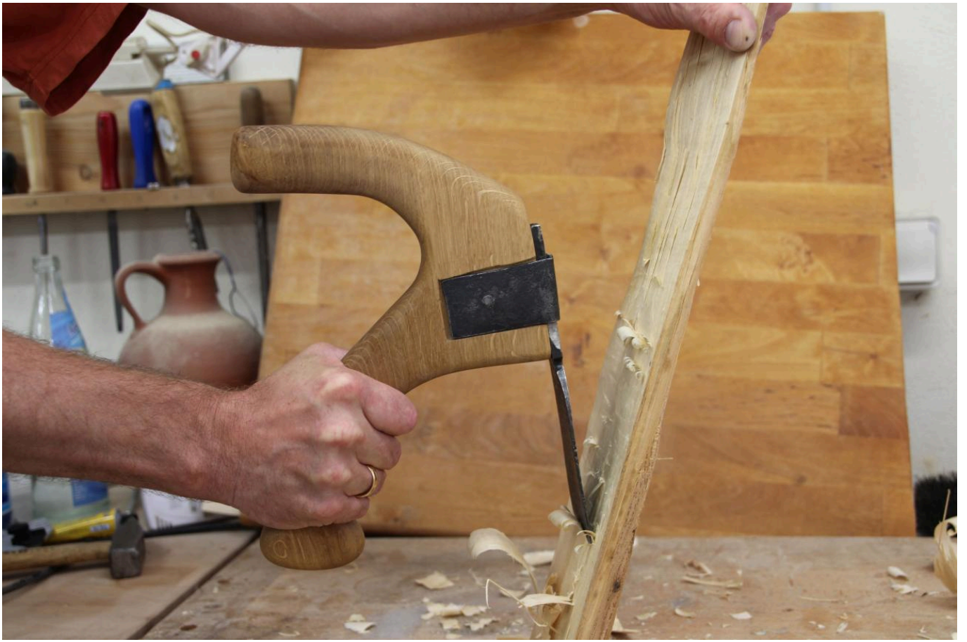
FIG 8. THE TWO-HANDLED ADZE IN USE FOR CHOPPING. PHOTO: RÜDIGER SCHWARZ
