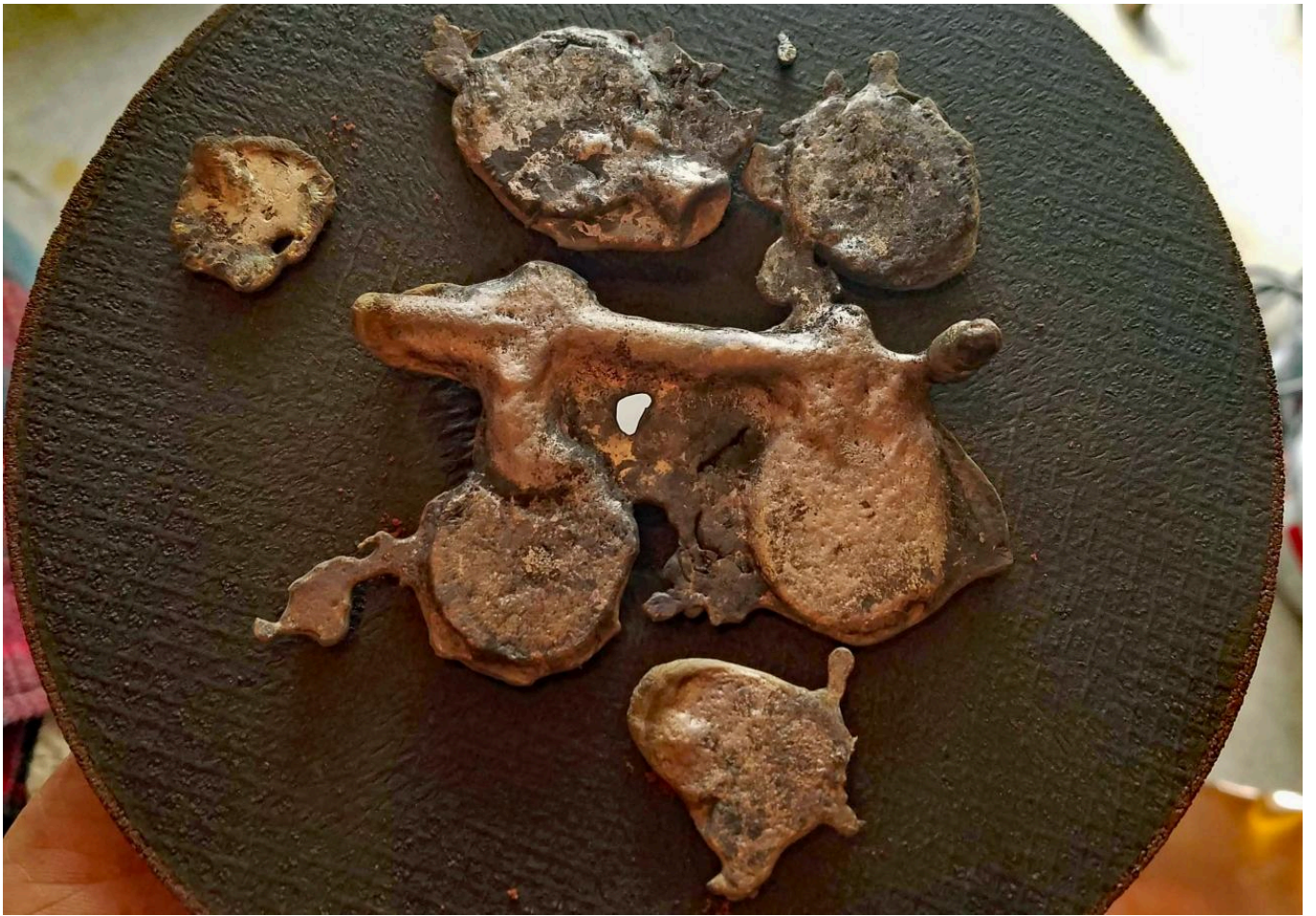
FIG 10. BRONZE DISKS CAST IN OPEN MOULD. NOTE UNEVEN SURFACE, EXCESSIVE OVERFLOW, DEEP OXIDES. PHOTO BY CHELSEA KAUFMAN
