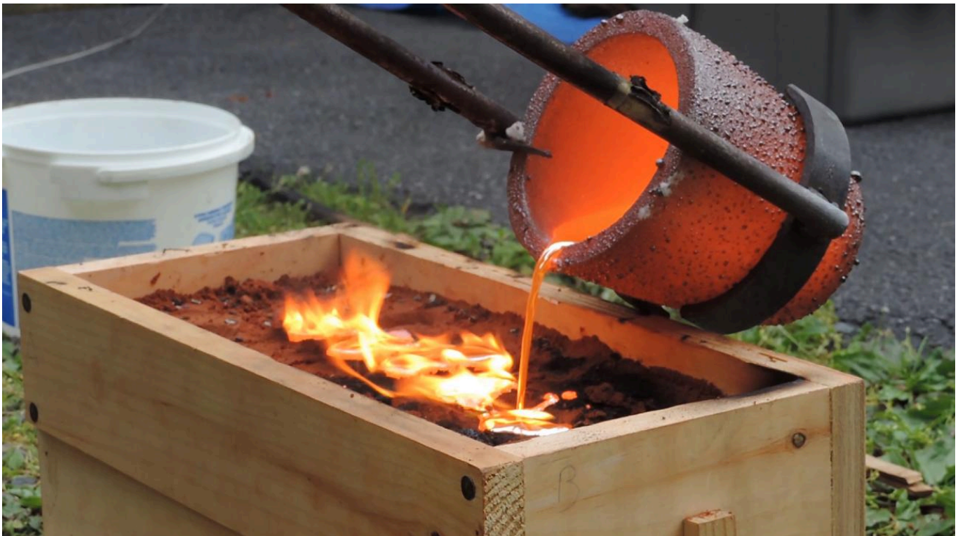
FIG 11. POURING MOLTEN COPPER-ALLOY INTO AN OPEN SAND MOULD. PHOTO BY CHELSEA KAUFMAN
