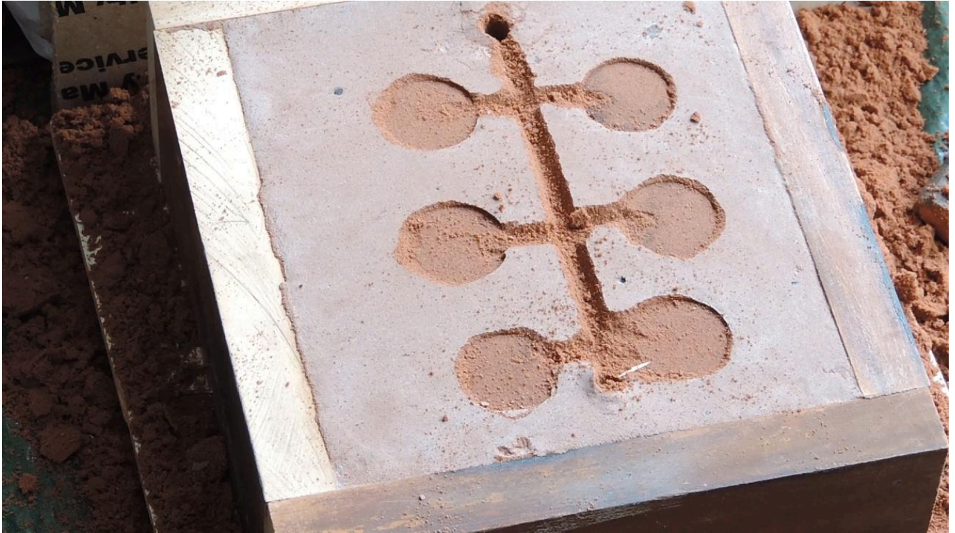
FIG 9A. : COPE & DRAG SAND MOULD LOWER HALF AFTER PACKING SHOWING DISK PATTERNS AND ADDED RUNNERS. PHOTO BY CHELSEA KAUFMAN
