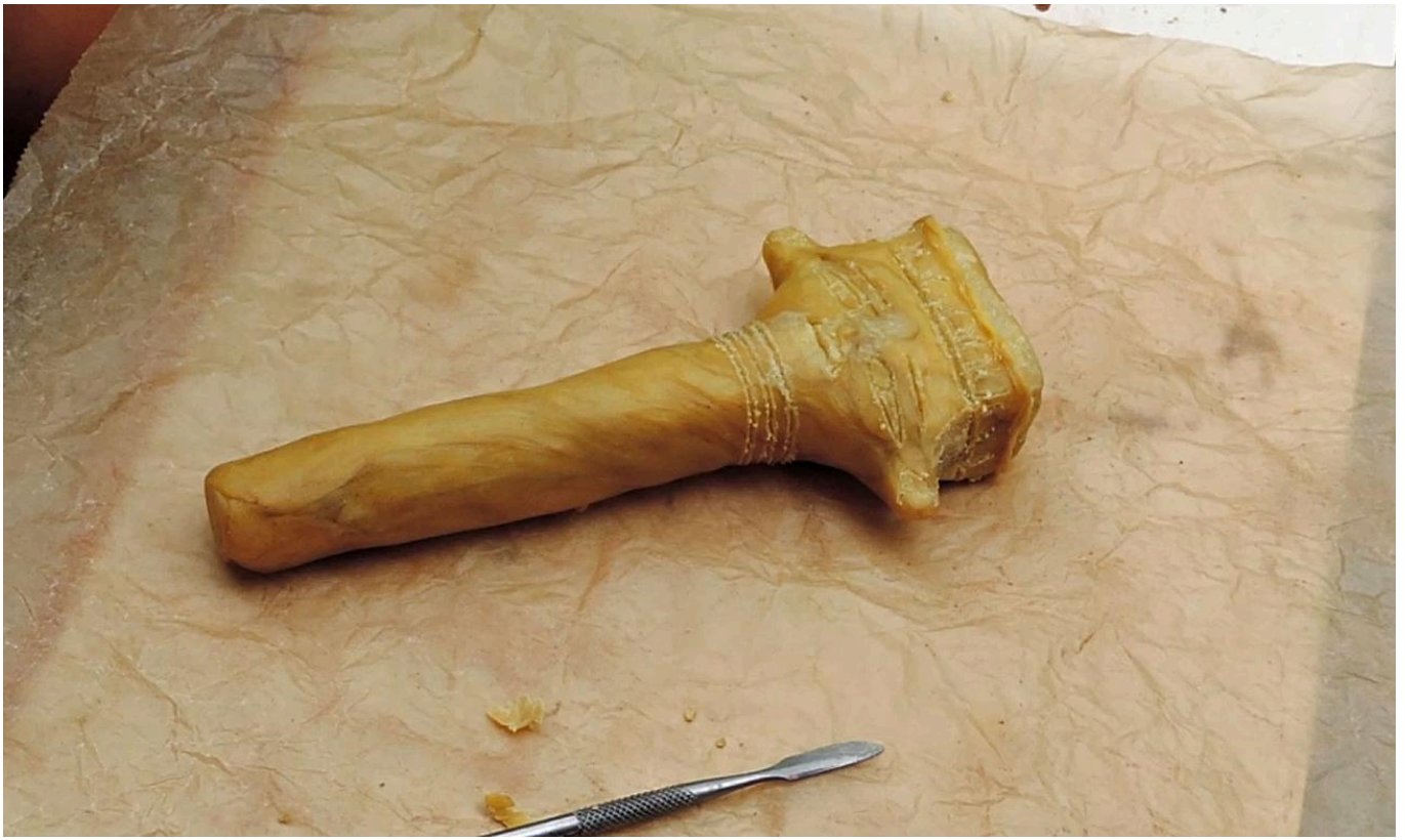
FIG 4. WAX SISTRUM HANDLE WHICH WAS USED AS THE LOST WAX PATTERN FOR OUR SISTRUM. CARVING DONE BY CHELSEA KAUFMAN. PHOTO BY CHELSEA KAUFMAN
