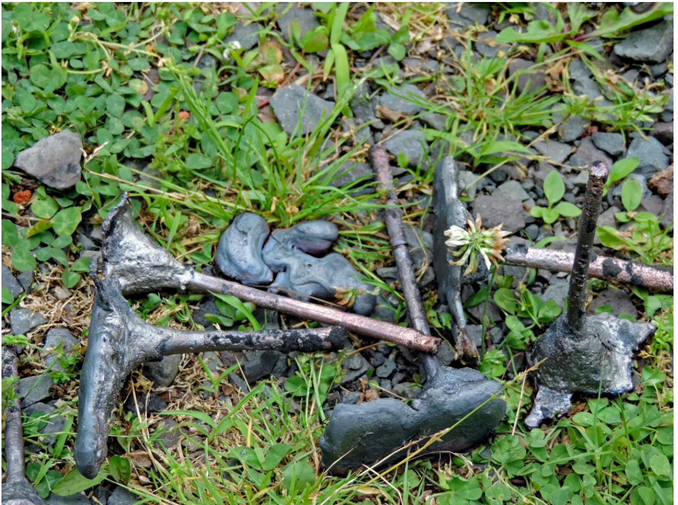
FIG 12. CAST COPPER CROSS PINS. THE CASTINGS WERE OUTWARDLY ACCEPTABLE; HOWEVER ONCE COLD WORKING BEGAN THEY WERE FOUND TO BE RIDDLED WITH POROSITY AND DID NOT SURVIVE. PHOTO BY CHELSEA KAUFMAN
