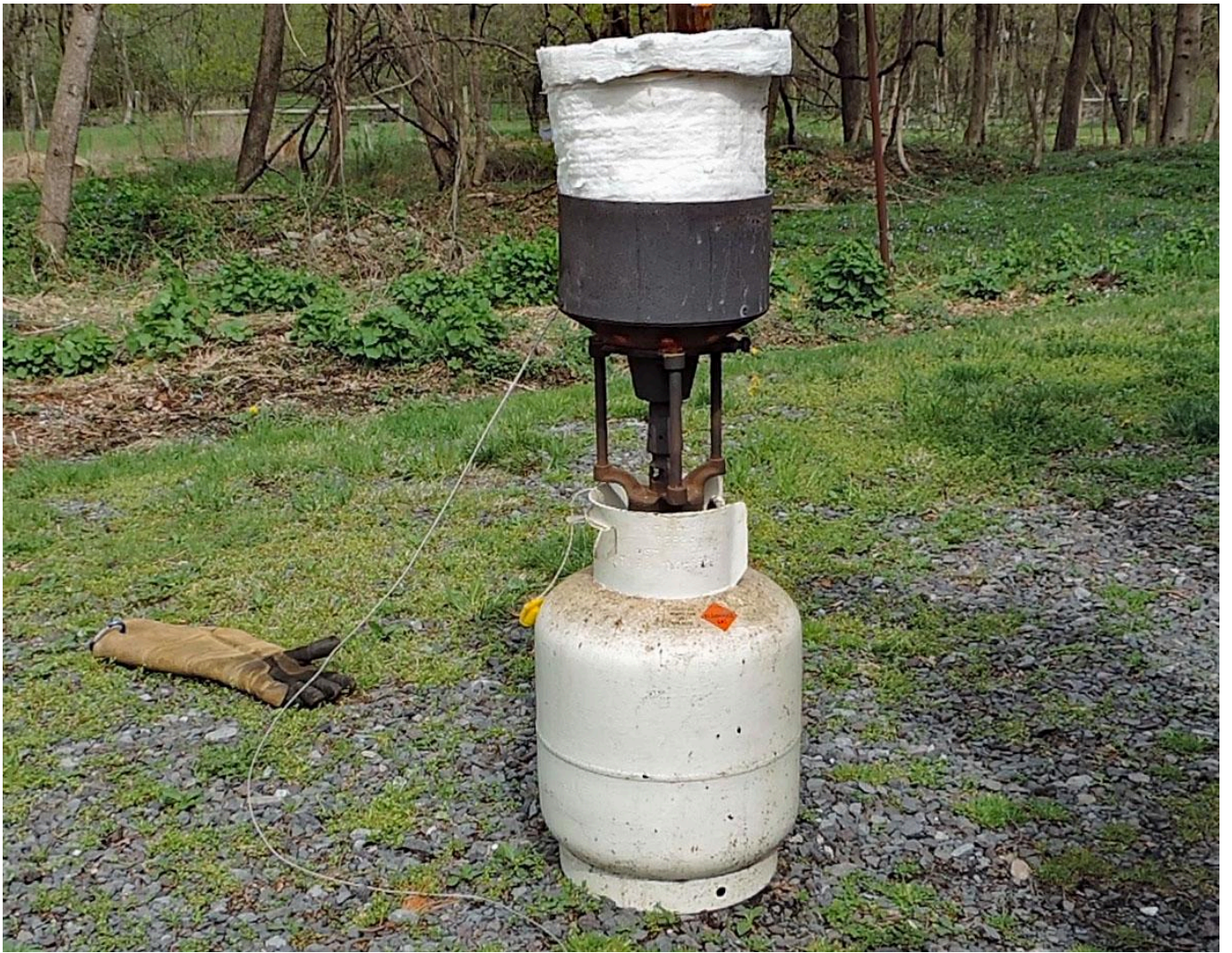
FIG 6. ANTIQUE PLUMBERS LEAD MELTER, POWERED BY PROPANE, OUTFITTED WITH REFRACTORY WOOL IN THE MELTING PAN TO CREATE AN ENCLOSED "PIT FURNACE" SPACE. PHOTO BY CHELSEA KAUFMAN
