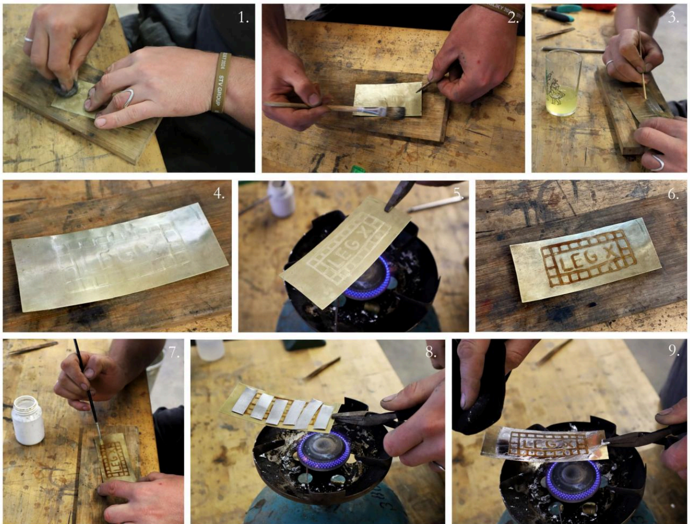
FIG 16. CHAÎNE OPÉRATOIRE OF PARTIAL TINNING USING EGG GLAIRE: 1. MECHANICAL CLEANING OF BRASS SHEET WITH STEEL WOOL. 2. ADDITIONAL CLEANING WITH SULPHURIC ACID WITH SUBSEQUENT CLEANING WITH WATER. 3. APPLICATION OF EGG GLAIRE USING A WOODEN STICK. 4. THE EGG GLAIRE APPEARS TRANSPARENT WHEN FIRST APPLIED. 5. HEATING OF THE EGG GLAIRE. 6. ACTIVATION OF THE EGG GLAIRE. 7. APPLICATION OF FLUX TO THE AREAS TO BE TINNED. 8. REHEATING THE BRASS SHEET WITH TIN PLACED ON TOP. 9. ONCE MELTED, THE TIN IS SPREAD USING A SOFT CLOTH. PHOTOS BY M.A. WIJNHOFEN AND M. KMOŠEK.
