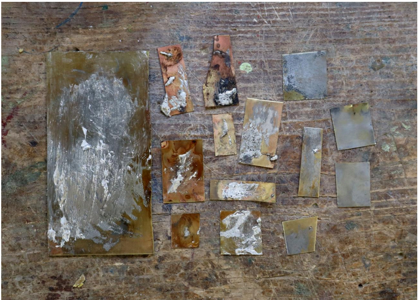
FIG 12. THE ABILITY TO TIN A BRASS OBJECT IS NOT EASY AND REQUIRED A STEEP LEARNING CURVE, AS EVIDENCED BY THESE FAILED ATTEMPTS (TIMELINE FROM LEFT TO RIGHT). PHOTO BY M.A. WIJNHOFEN AND M. KMOŠEK.
