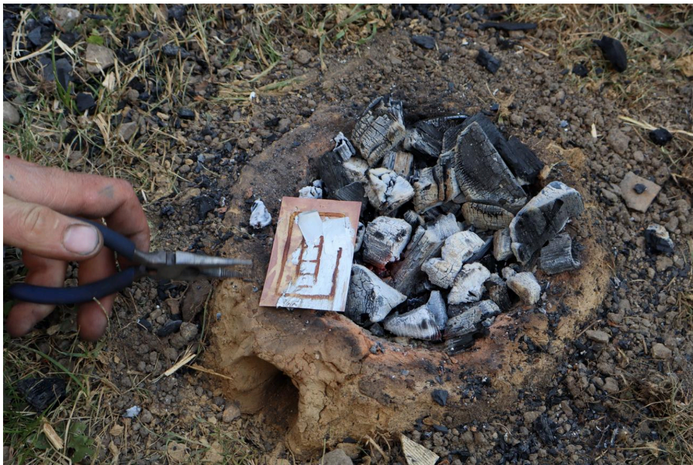
FIG 11. EXPERIMENTATION TO REPLICATE PARTIAL TINNING CONDUCTED ON A SMALL OPEN-PIT CHARCOAL HEARTH. PHOTO BY M.A. WIJNHOFEN AND M. KMOŠEK.
