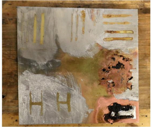
FIG 14. VARIOUS MECHANICAL MASKING MATERIALS WERE TESTED DURING TINNING, INCLUDING CARBON, HEMATITE, CLAY, HONEY, SUGAR WATER, MILK, AND EGG. MOST PROVED INEFFECTIVE, EITHER WIPING AWAY EASILY OR SPREADING UNCONTROLLABLY WHEN HEATED. MILK, EGG YOLK, AND EGG WHITE PERFORMED BETTER, ESPECIALLY AFTER BEING BAKED ONTO THE SURFACE BEFORE TINNING. PHOTOS BY M.A. WIJNHOFEN AND M. KMOŠEK.
