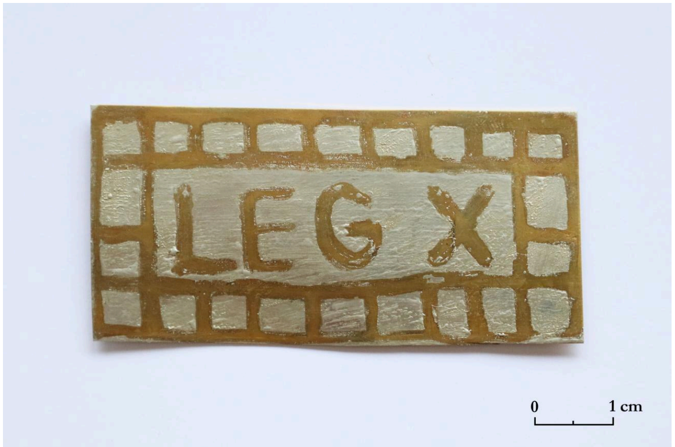
FIG 18. OF ALL TESTED METHODS, EGG GLAIRE BEST REPLICATED THE PARTIAL TINNING SEEN ON ROMAN ARTEFACTS. WITH MORE EXPERIENCE AND PRACTICE, EVEN CLOSER RESULTS SEEM ACHIEVABLE. PHOTO BY M.A. WIJNHOFEN AND M. KMOŠEK.
