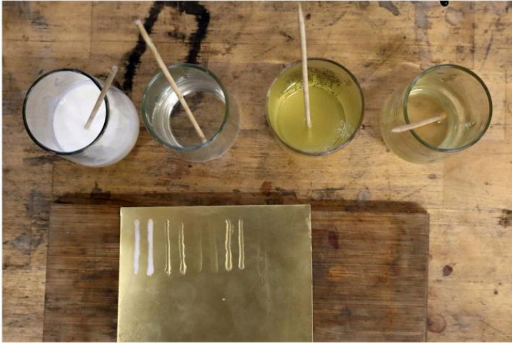
FIG 14. VARIOUS MECHANICAL MASKING MATERIALS WERE TESTED DURING TINNING, INCLUDING CARBON, HEMATITE, CLAY, HONEY, SUGAR WATER, MILK, AND EGG. MOST PROVED INEFFECTIVE, EITHER WIPING AWAY EASILY OR SPREADING UNCONTROLLABLY WHEN HEATED. MILK, EGG YOLK, AND EGG WHITE PERFORMED BETTER, ESPECIALLY AFTER BEING BAKED ONTO THE SURFACE BEFORE TINNING. PHOTOS BY M.A. WIJNHOFEN AND M. KMOŠEK.
