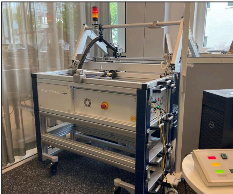
FIG 5. MICRO-XRF ANALYSIS OF THE MUŠOV CHEST PLATE BEING CONDUCTED AT BRUKER NANO ANALYTICS, USING AN M6 JETSTREAM SPECTROMETER. PHOTOS BY M. KMOŠEK AND M.A. WIJNHOFEN.
