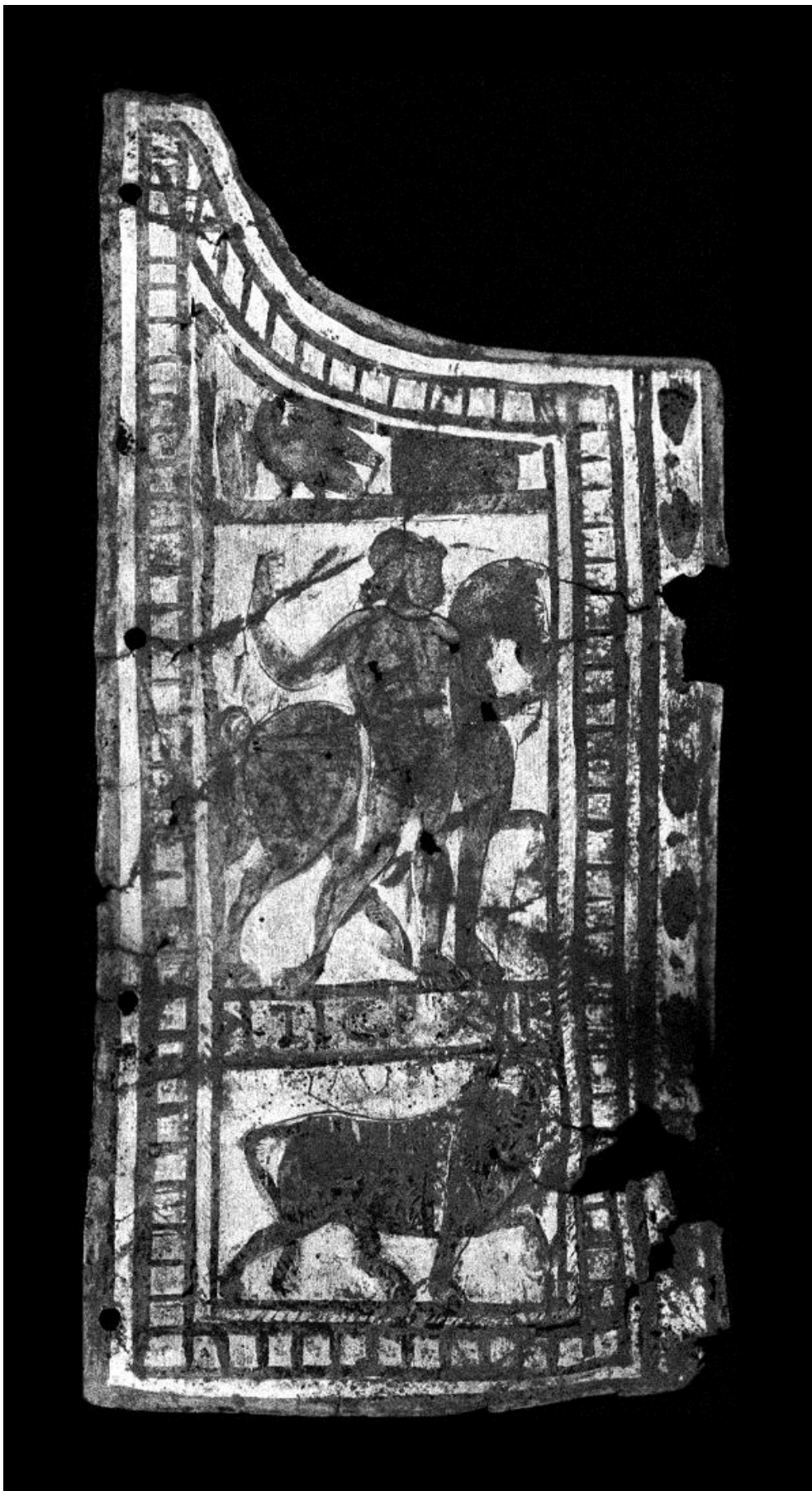
FIG 6. RESULTS OF THE MICRO-XRF ANALYSIS SET TO DETECT TIN (SN LA LINES) ON THE SURFACE OF THE MUŠOV CHEST PLATE. THE IMAGE CLEARLY INDICATES WHICH AREAS WERE ORIGINALLY TINNED AND WHICH WERE LEFT UNTREATED. IMAGE BY BRUKER NANO ANALYTICS.
