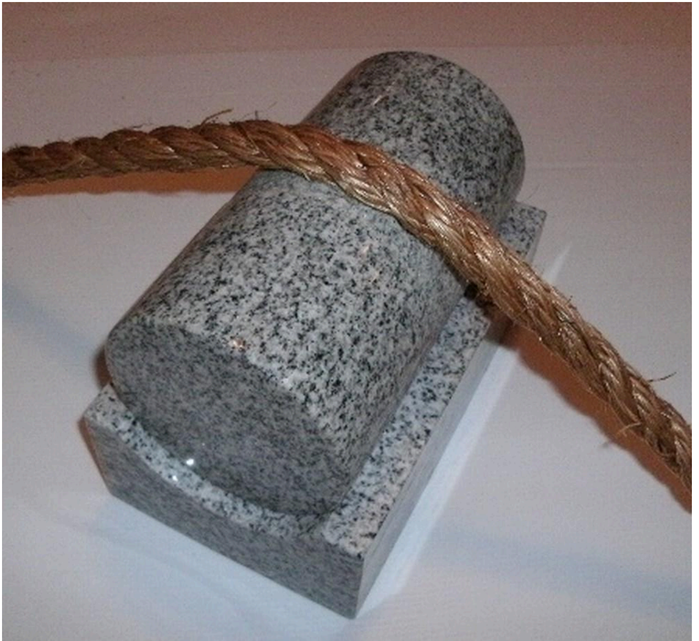
FIG 4. PROTOTYPE GRANITE EGYPTIAN PULLEY, WITH 10.2 CM DIAMETER CYLINDER PHOTO BY STEPHEN BLAKELY
