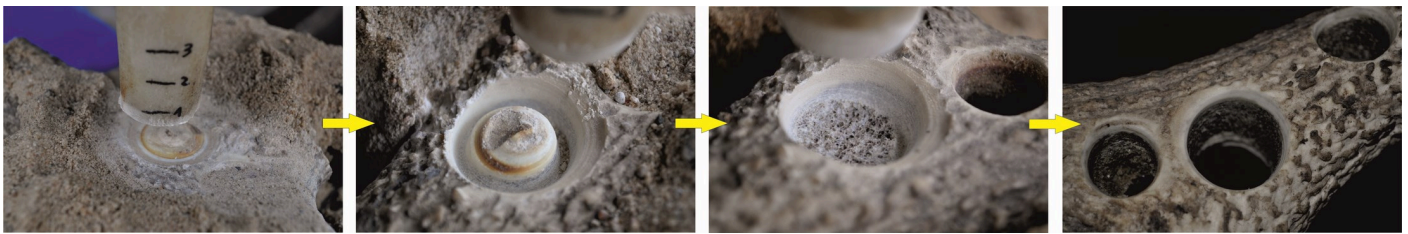
FIG 5. EXPERIMENTAL DRILLING IN ANTLER WITH THE USE OF BONE DRILL BITS – SELECTED PHOTOS (FOT. J. ORLOWSKA).
