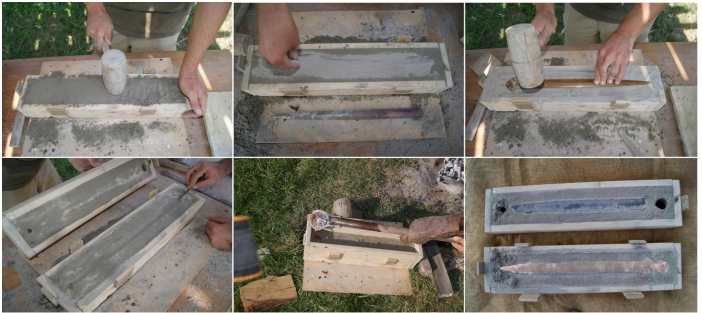
FIG 4. THE MANUFACTURING PHASES OF SWORD PRODUCTION.
