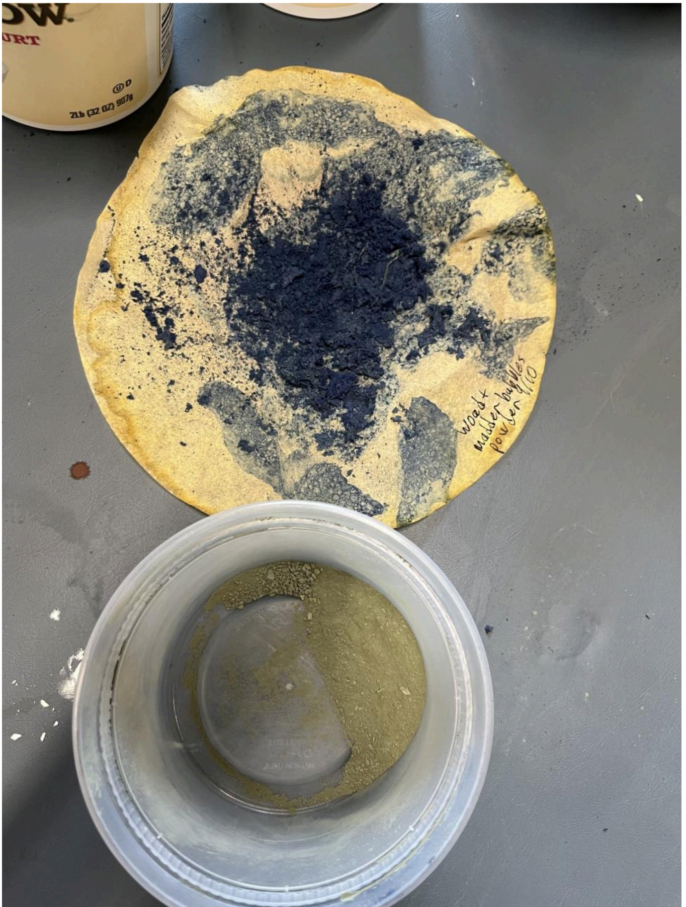
FIG 22. TWO BATCHES OF WOAD POWDER. TOP POWDER IS FROM DRYING OUT THE BUBBLES FROM THE TOP OF A MODERN WOAD VAT, BOTTOM POWDER IS FROM STRAINING FERMENTED WOAD LIQUID. PHOTO BY BECKER AND BANTA.
