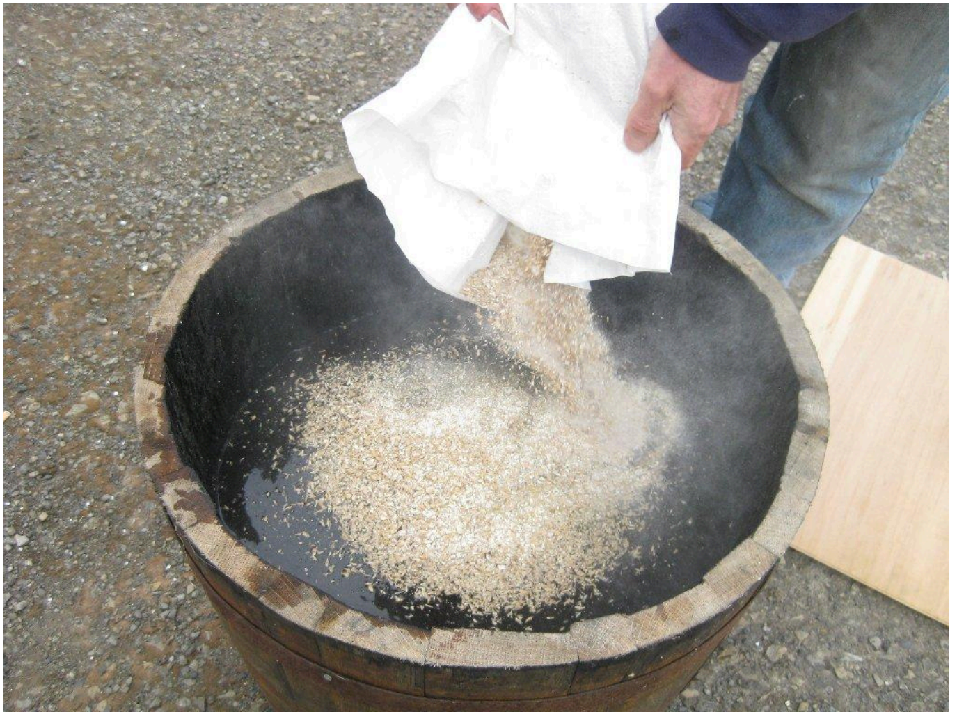
FIG 7. ADDING CRUSHED MALT TO HOT WATER IN THE MASH TUN. THIS IS CALLED THE 'STRIKE'.
