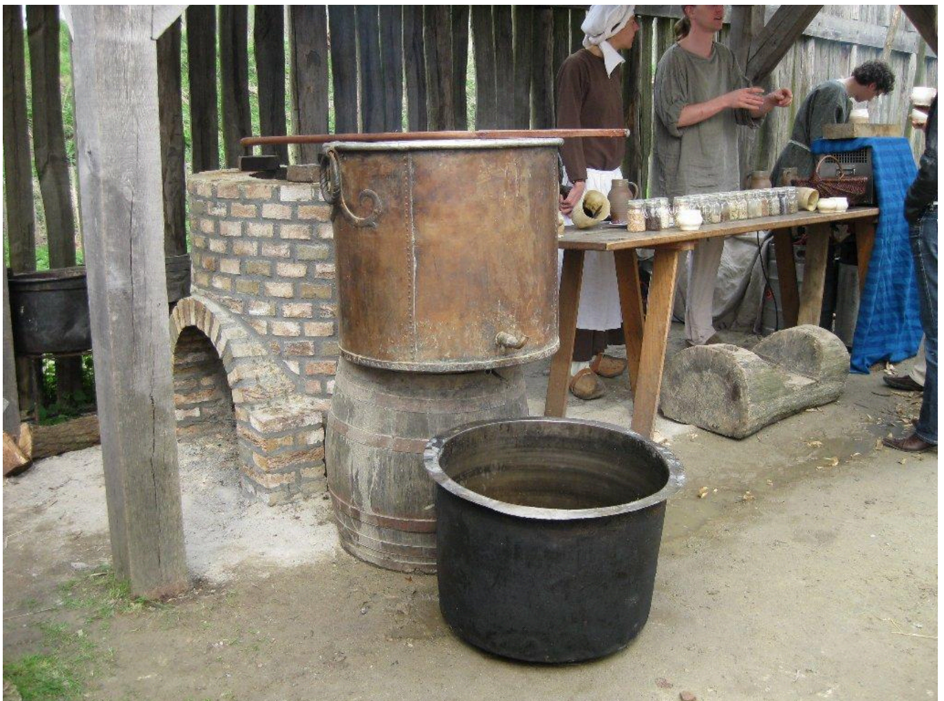
FIG 2. BREWING EQUIPMENT AT EINDHOVEN MUSEUM (NL). BRICK BUILT MASH OVEN, MASH TUN AND LAUTER TUN.
