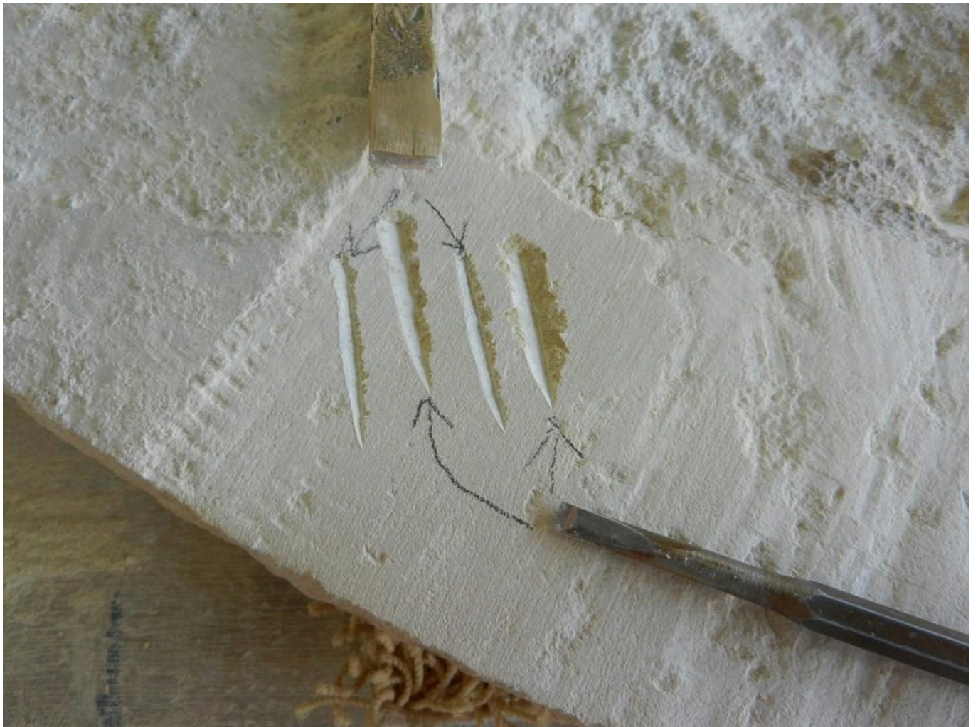
FIG 11. THE DIFFERENCE OF THE CUTTING DEPTH OF A BRONZE CHISEL AND A MODERN CHISEL WITH A CUTTING EDGE MADE OF SYNTHETIC DIAMOND. PHOTO: M. LOWE FRI.
