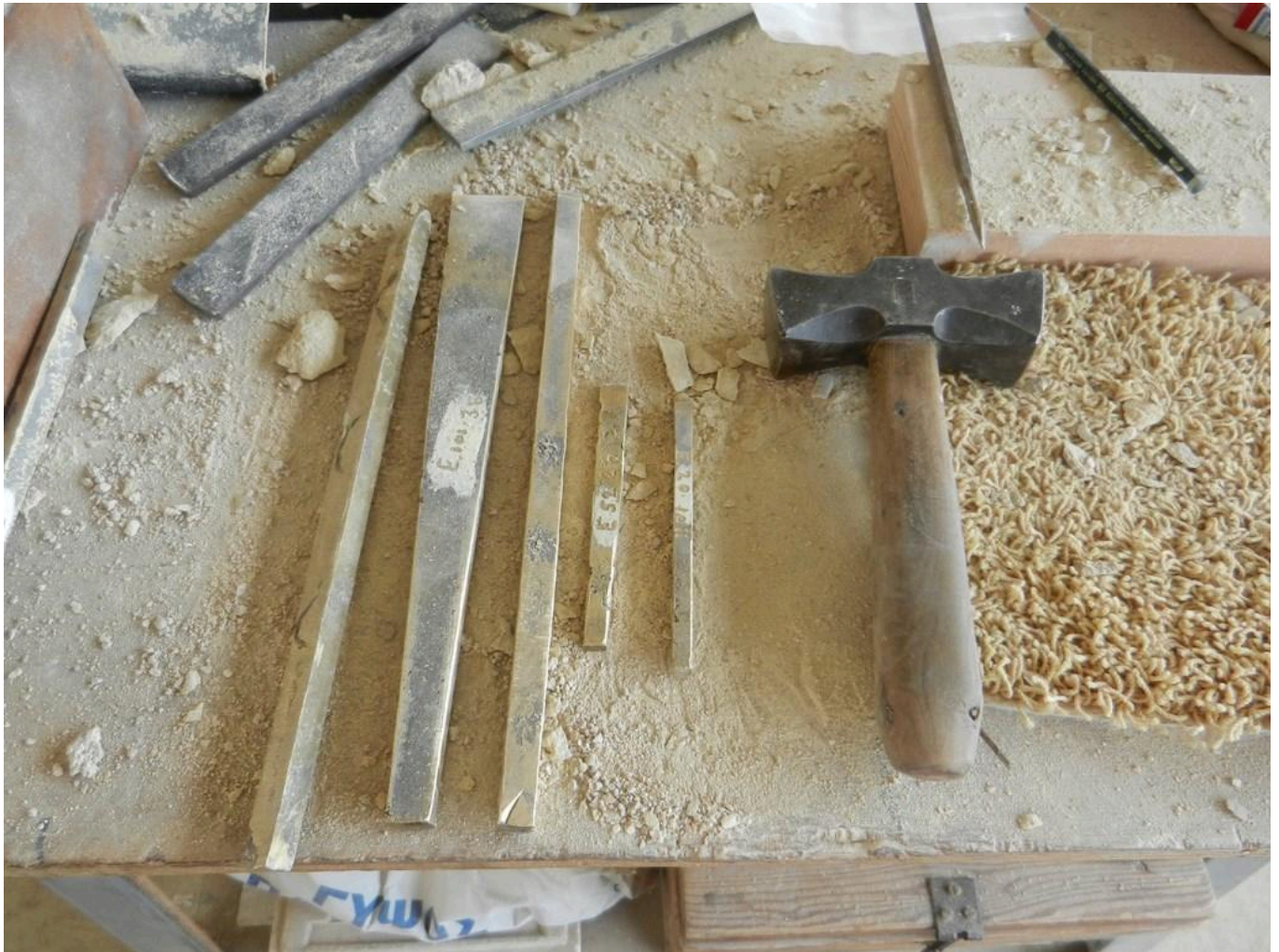
FIG 7. THE CHISELS USED IN THE RELIEF-CARVING EXPERIMENT. THE HAMMER IS NOT A MINOAN REPLICA, BUT BELONGS TO PETROS GEORGOPOULOS. A MINOAN ONE WOULD HAVE BEEN OF EITHER STONE OR WOOD. PHOTO: M. LOWE FRI
