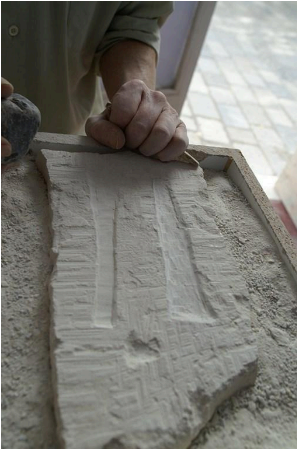
FIG 4. ONE INTERESTING RESULT, WHEN CARVING THE MOULD, WAS THAT DIFFERENT MARKS WERE CREATED BY THE CHISEL DEPENDING ON IF A WOODEN MALLET OR A STONE WAS USED AS A HAMMER. THE SMOOTHER RIDGES IN THE STONE (TO THE LEFT) WERE CREATED BY THE WOODEN MALLET AND THE SMALLER AND MORE DISTINCT MARKS (TO THE RIGHT) WERE CREATED BY USING THE STONE AS A HAMMER. PHOTO: M. LOWE FRI.
