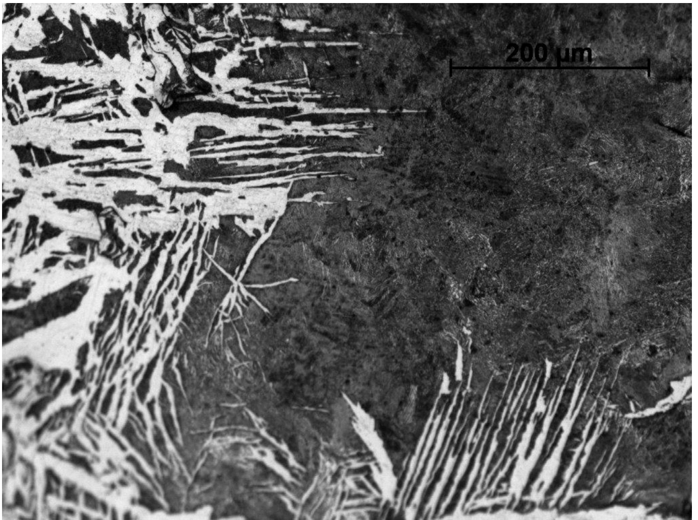
FIG 6. MICRO-PHOTOGRAPH OF INGOT NR 2. TRANSITION BETWEEN PEARLITE-FERRITIC STRUCTURE AND MORE CARBURIZED PEARLITIC ZONE.
