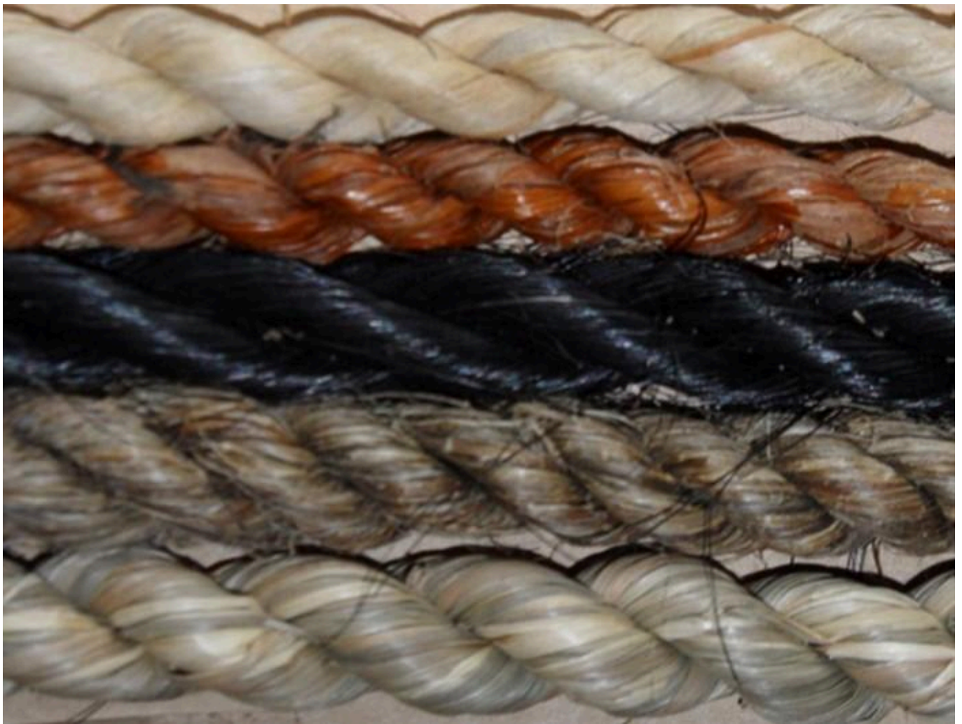
FIG 20. ROPE FROM TOP DOWN: LIME BARK, WILLOW, HORSEHAIR ,STINGING NETTLE AND GRASS, PHOTO EVA IJSVELD
