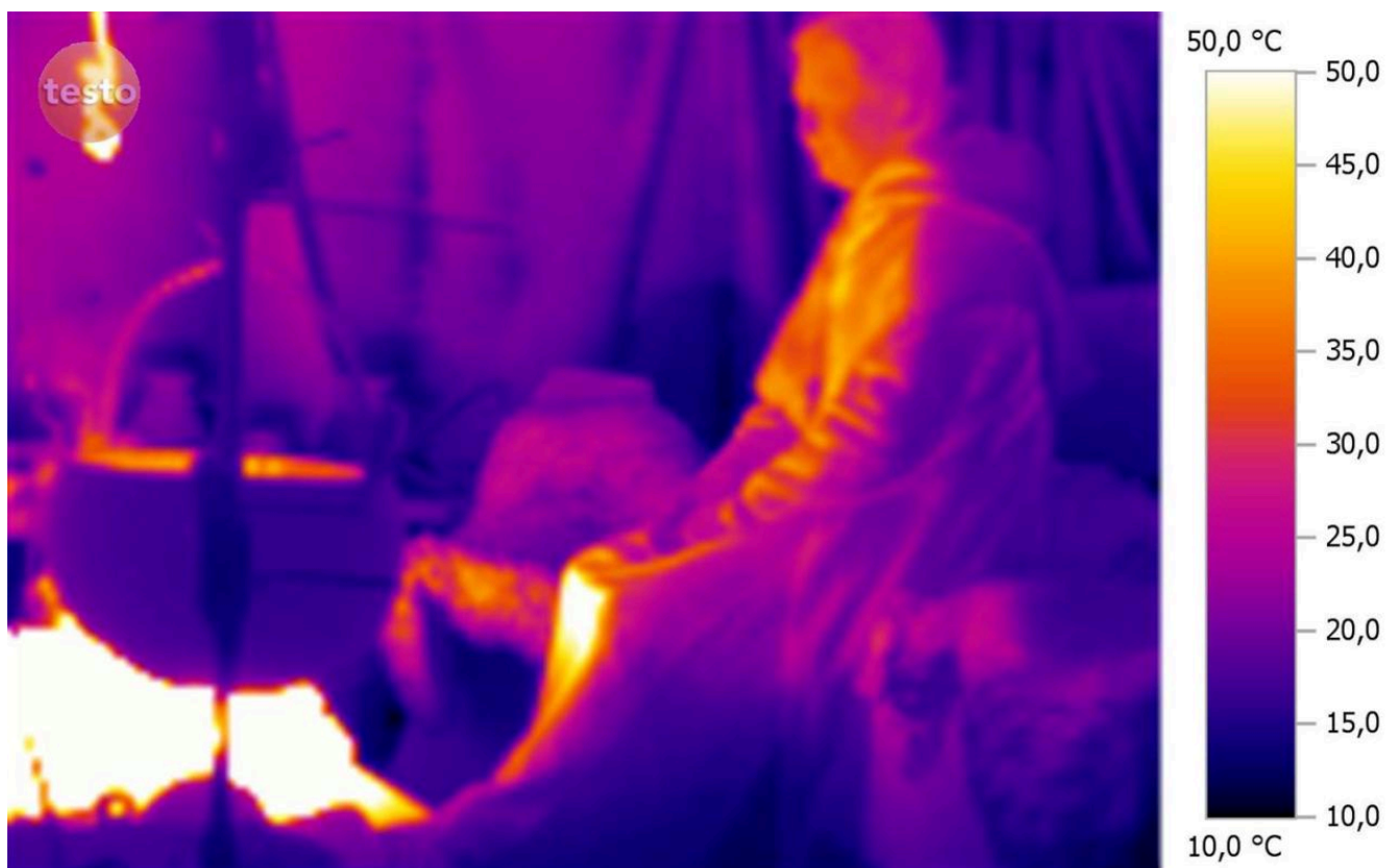
FIG 4. THERMAL IMAGE SHOWING THE ASYMMETRIC SURFACE TEMPERATURE ON A PERSON'S CLOTHES (APPROXIMATELY 15-50 °C) AND ON THE INTERIOR (DOWN TO 10-25 °C).
