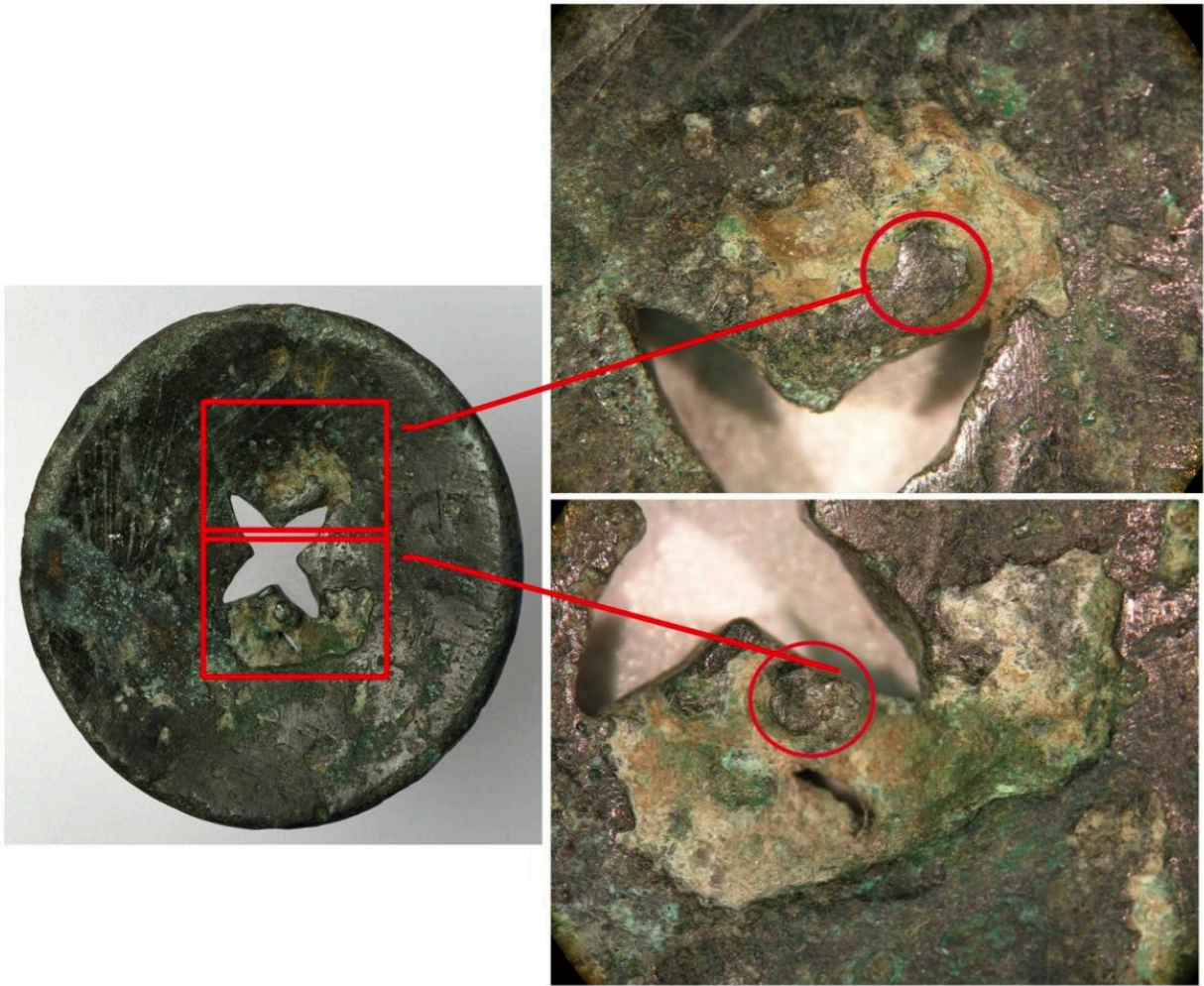
FIG 5. REAR VIEW OF THE PIECE WITH SIGNS OF SPRUES AMPLIFIED.
