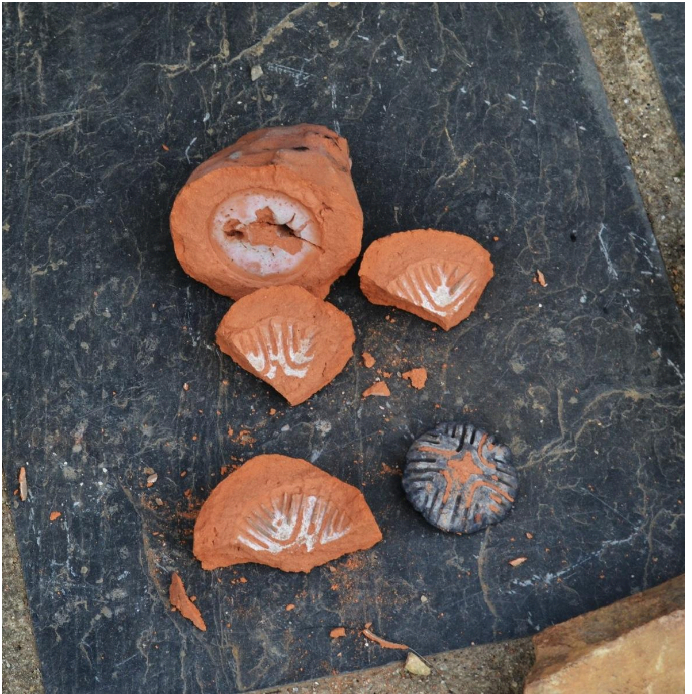
FIG 10. EXTRACTION OF THE PIECE FROM THE MOULD
