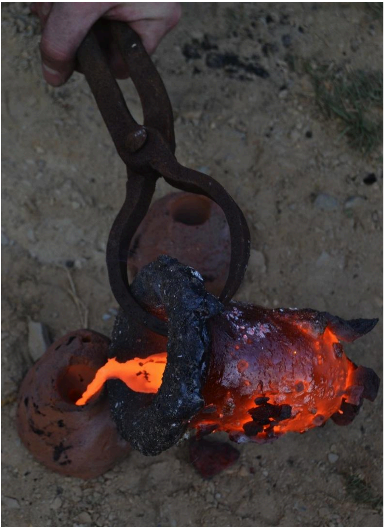
FIG 9. POURING OF BRONZE INTO THE MOULD.
