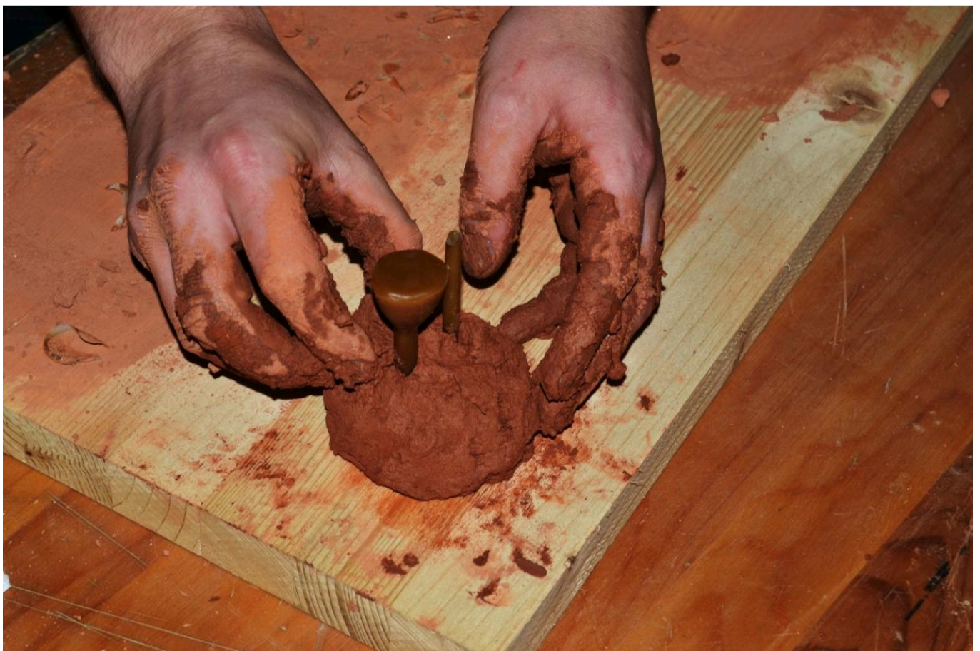
FIG 7. MANUFACTURE OF CLAY MOULD.
