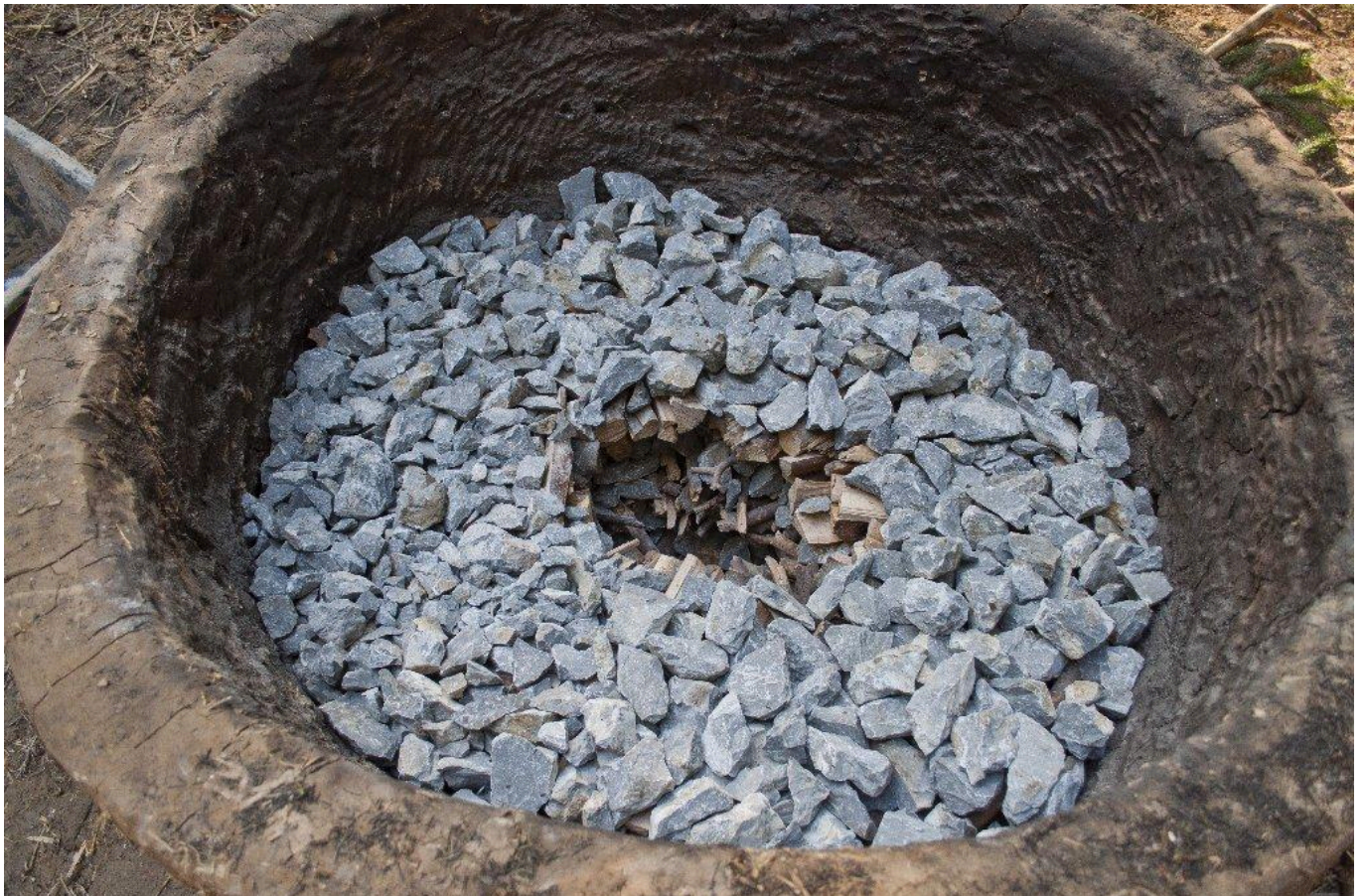
FIG 2. LAYER OF WOOD IN A ONE-CHAMBER BURNING.
