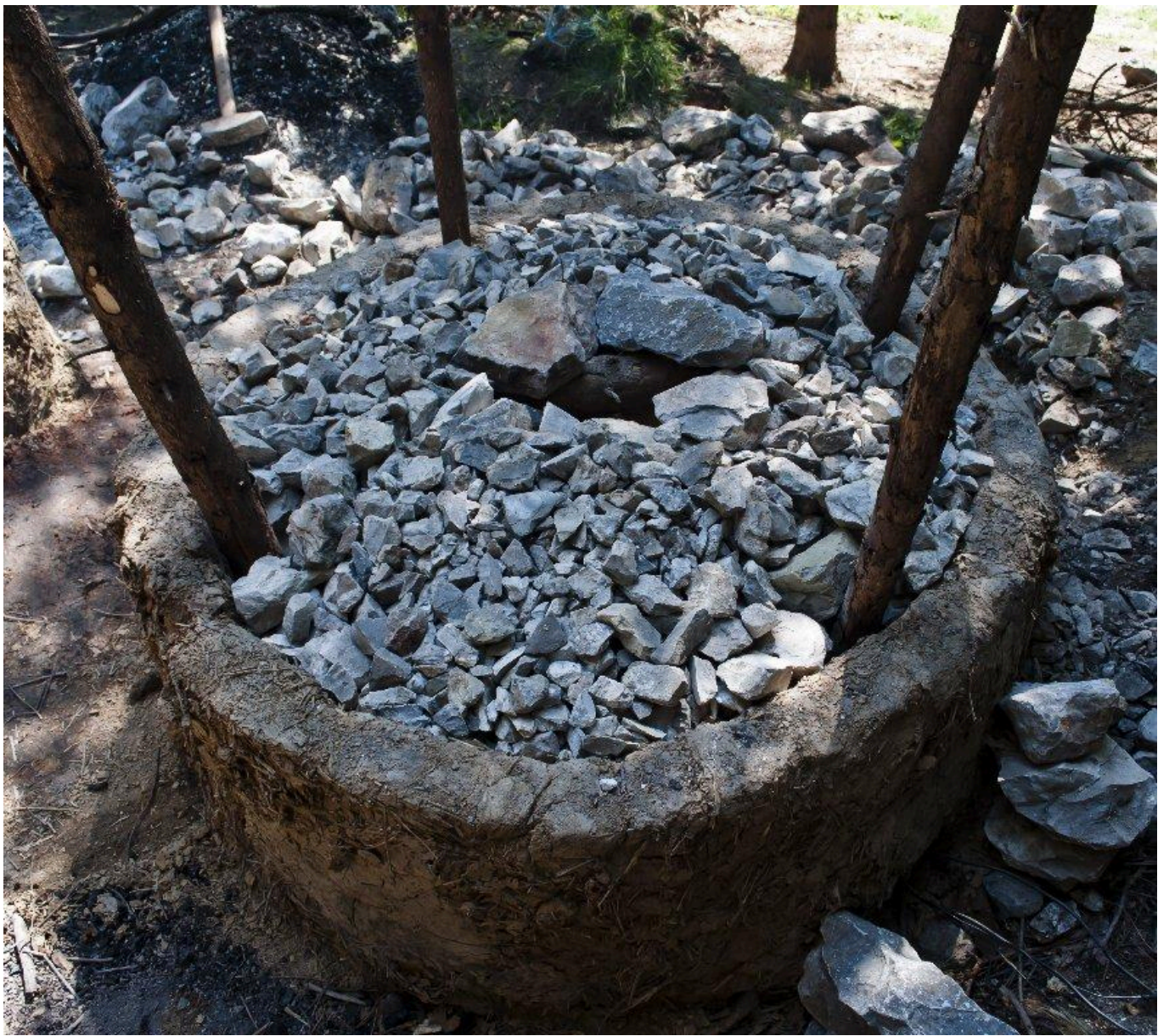
FIG 6. LOADING OF THE SECOND ONE-CHAMBER BURNING.
