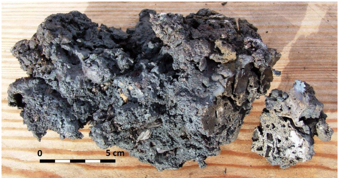
FIG 7. THE MAIN IRON BLOOM TAKEN FROM THE FIRST FURNACE IN STARACHOWICE. PHOTO – ADRIAN WRONA.
