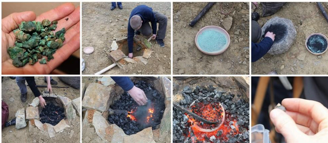
FIG 3. PARTS OF THE EXPERIMENT, FROM LEFT TO RIGHT: COPPER, SMELTING STRUCTURE, GROUND MALACHITE AND CASSITERITE, MINERALS MIXED WITH CARBON, INTRODUCTION OF THE SMELTING VESSEL, ADDITION OF MINERAL AND CARBON, VESSEL IN THE MOMENT OF EXTRACTION, DRIP OF METAL: RESULT OF THE PROCESS.
