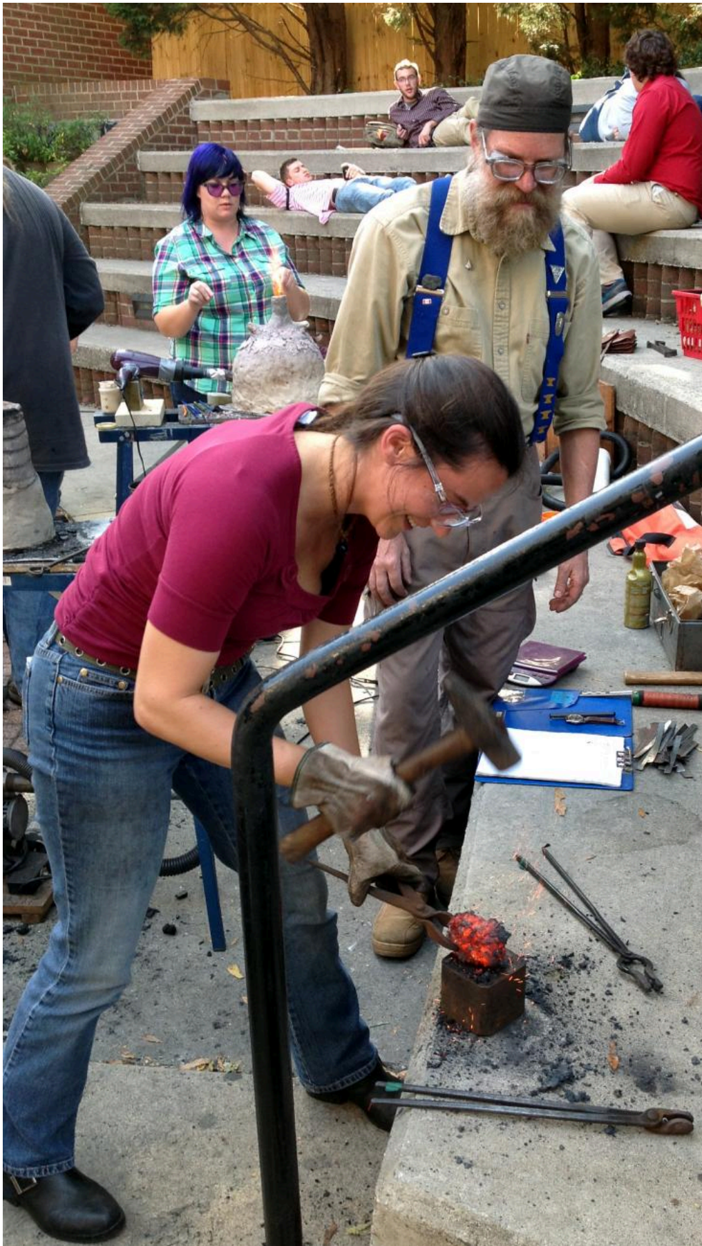
FIG. 2. FORGING A BLOOM WITH KAT MUELLER AND DARELL MARKEWITZ. PHOTO: BILL SCHINDLER
