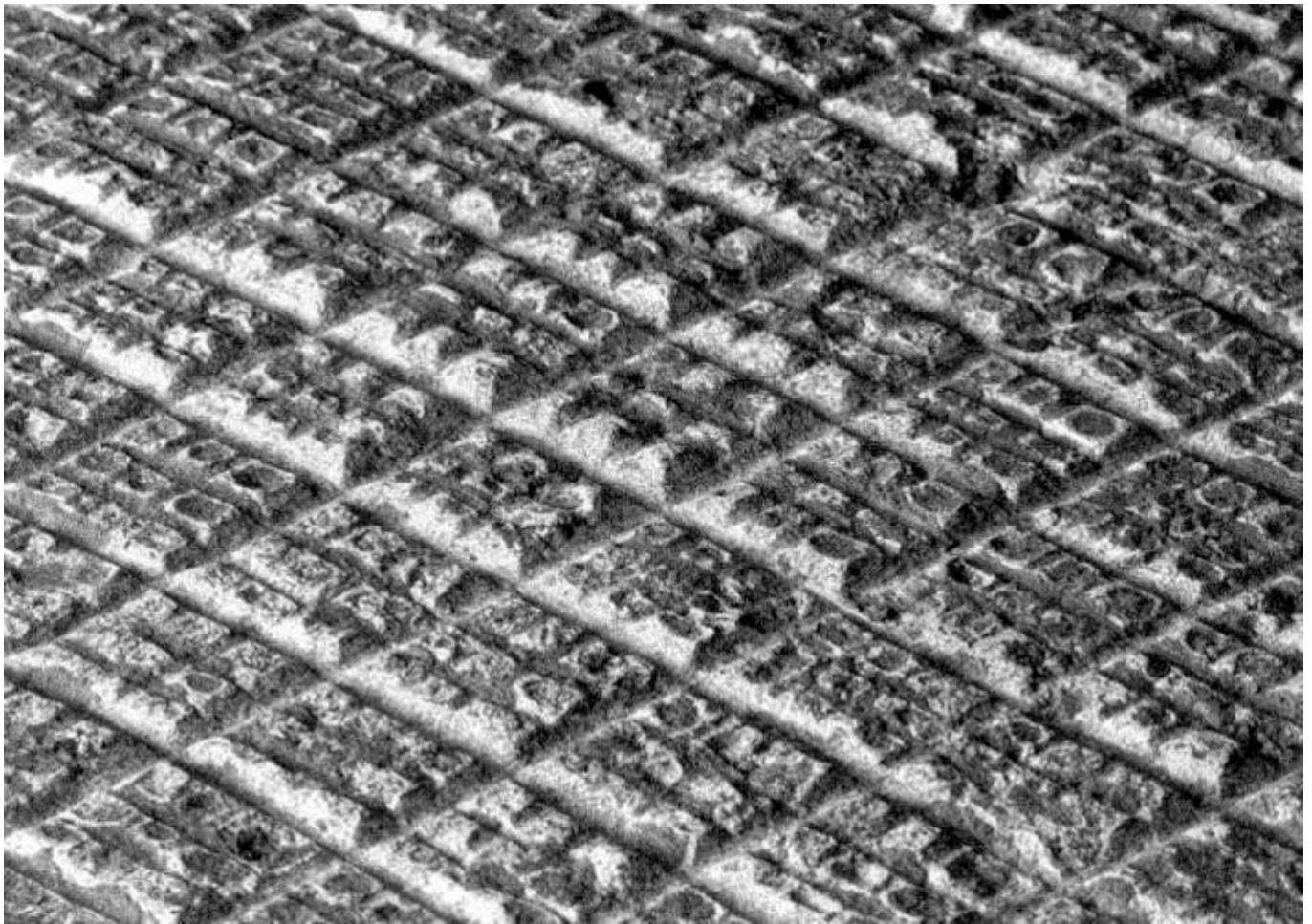
FIG 16. SEM IMAGE OF THE 'BOXED' PATTERN CASTING (X20). THE WHOLE PATTERN IS REPRODUCED, BUT THE SMALL DEPRESSIONS ON PYRAMIDS ARE FROM TRAPPED AIR (DURING WAX MOULDING OF THE SILICONE MODEL). WIDTH OF IMAGE 5.8 MM.
