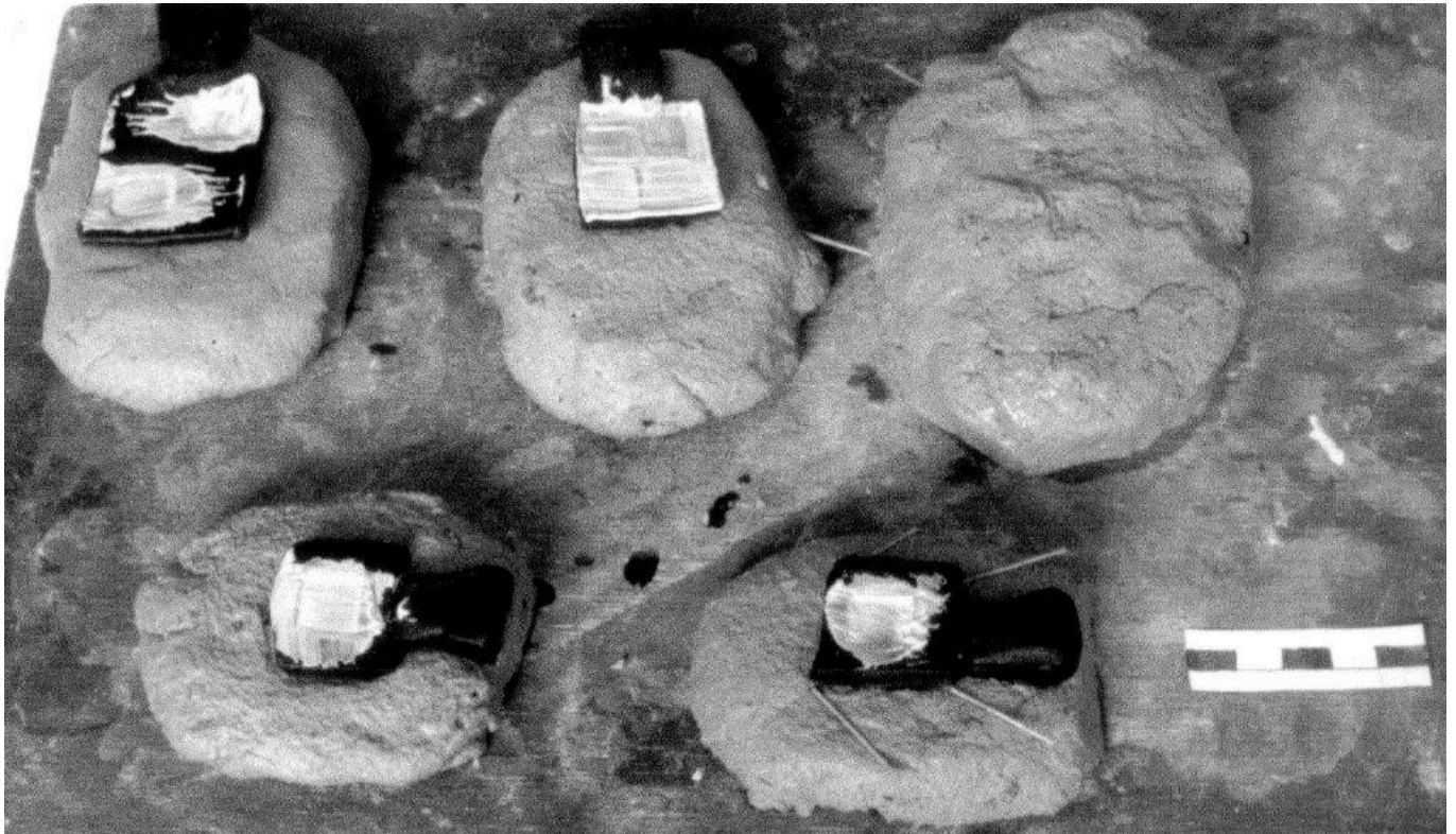
FIG 8. WAX IMPRESSIONS OF THE MODEL SUTTON HOO DIES BEING INVESTED IN CLAY, WITH STRAW RISERS.
