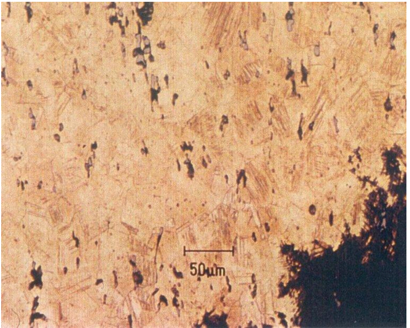
FIG 5D. THE DECORATED TORC. MICROGRAPHY OF A WIDTHWISE SECTION IN A BENT ZONE AFTER CHEMICAL ETCHING. IN THE RECRYSTALLIZED STRUCTURE, IT CAN BE NOTICED THAT THE ANNEALING TWINS ARE SLIGHTLY BENT AND SULPHIDE INCLUSIONS ARE BROKEN.
