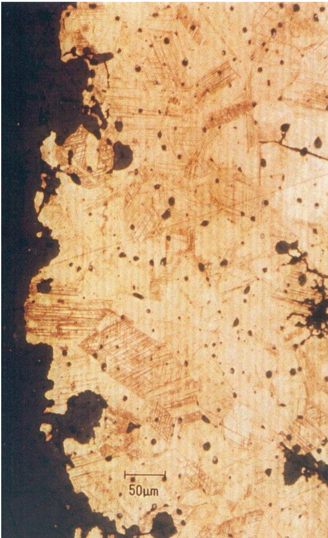
FIG 6C. VAUDREVANGE TYPE BRACELETS. MICROGRAPHY OF A WIDTHWISE SECTION AFTER CHEMICAL ETCHING. THE MICROSTRUCTURE IS NOT COMPLETELY RECRYSTALLIZED. MECHANICAL AND ANNEALING TWINS CAN BE SEEN; THE SULPHIDE INCLUSIONS (MEDIUM GREY) REMAIN WITH A GLOBULAR SHAPE (BRACELET NO 19.5).
