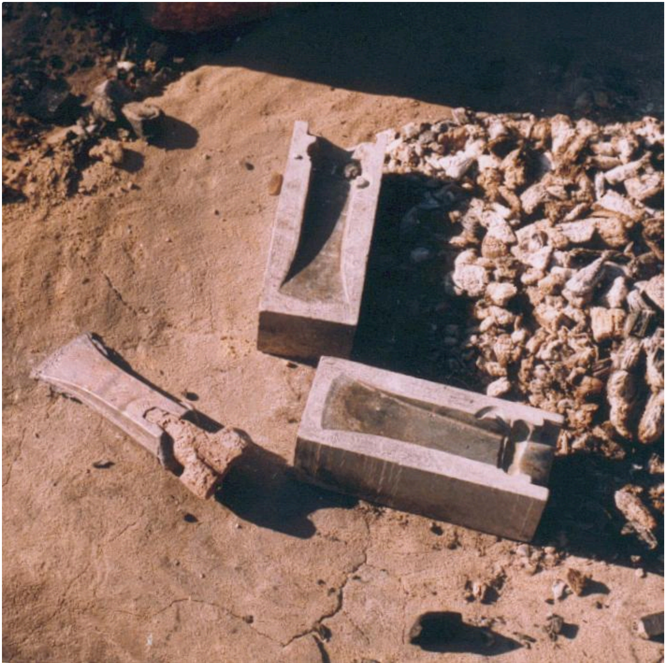
FIG 4. PROBLEMS WITH THE PRECISE POSITIONING OF THE CLAY CORE FOR THE SOCKET.
