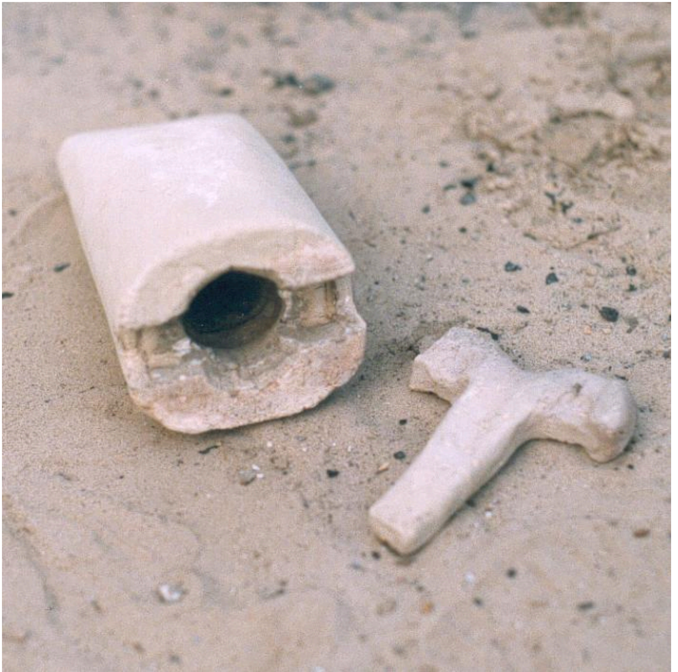
FIG 3. PROBLEMS WITH THE PRECISE POSITIONING OF THE CLAY CORE FOR THE SOCKET.
