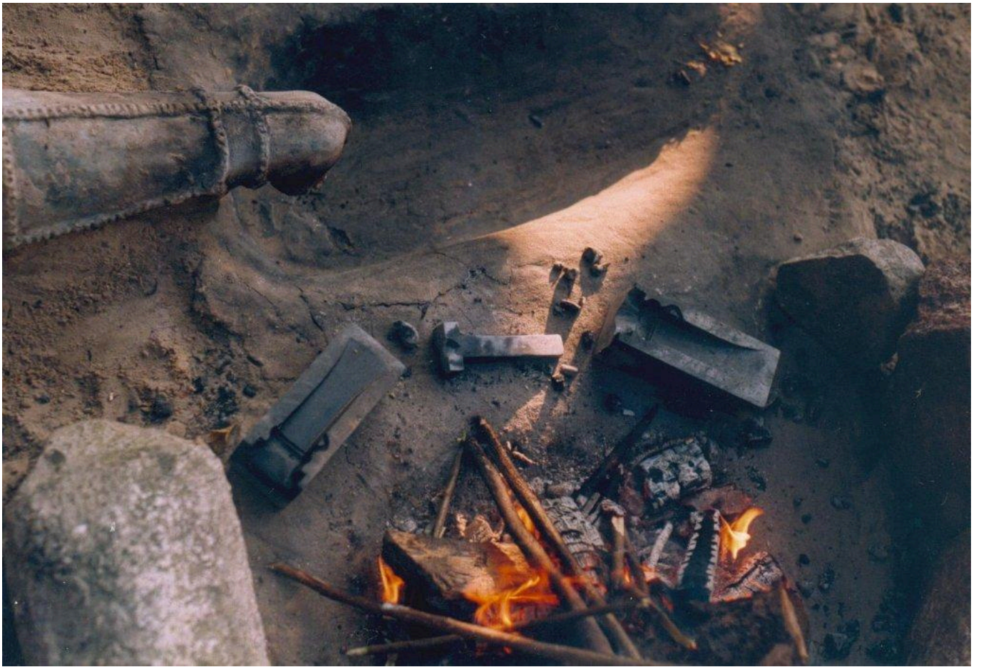
FIG 2. THE CAREFULLY TREATED SOAPSTONE MOULD BENEATH THE HEAT OF THE FURNACE.
