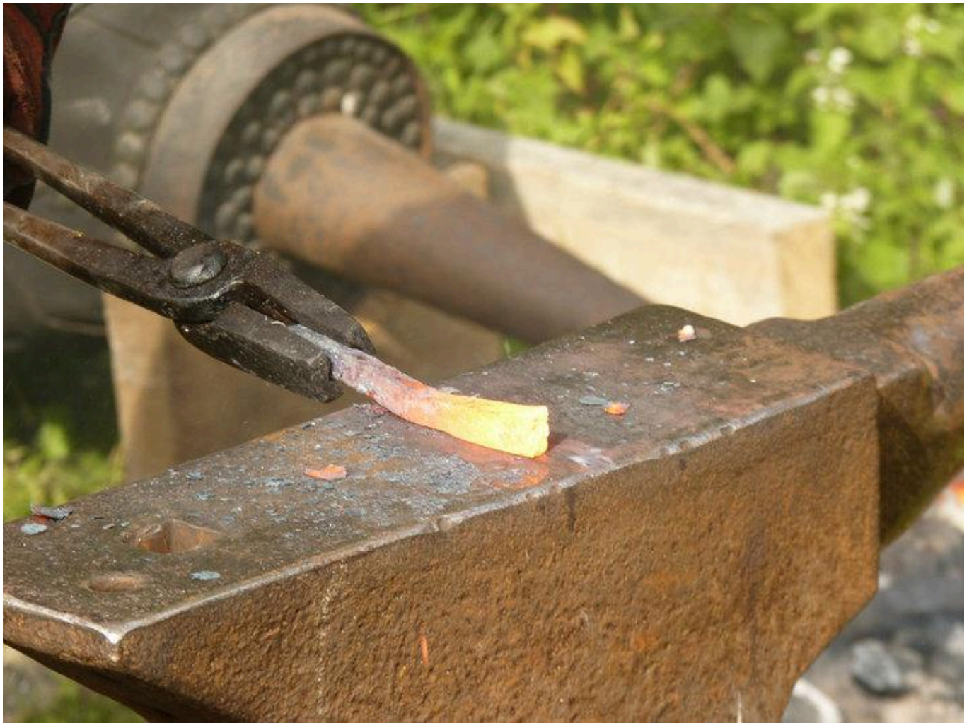
FIG 6. SMITHING A BLOOM DOWN INTO BARS.
