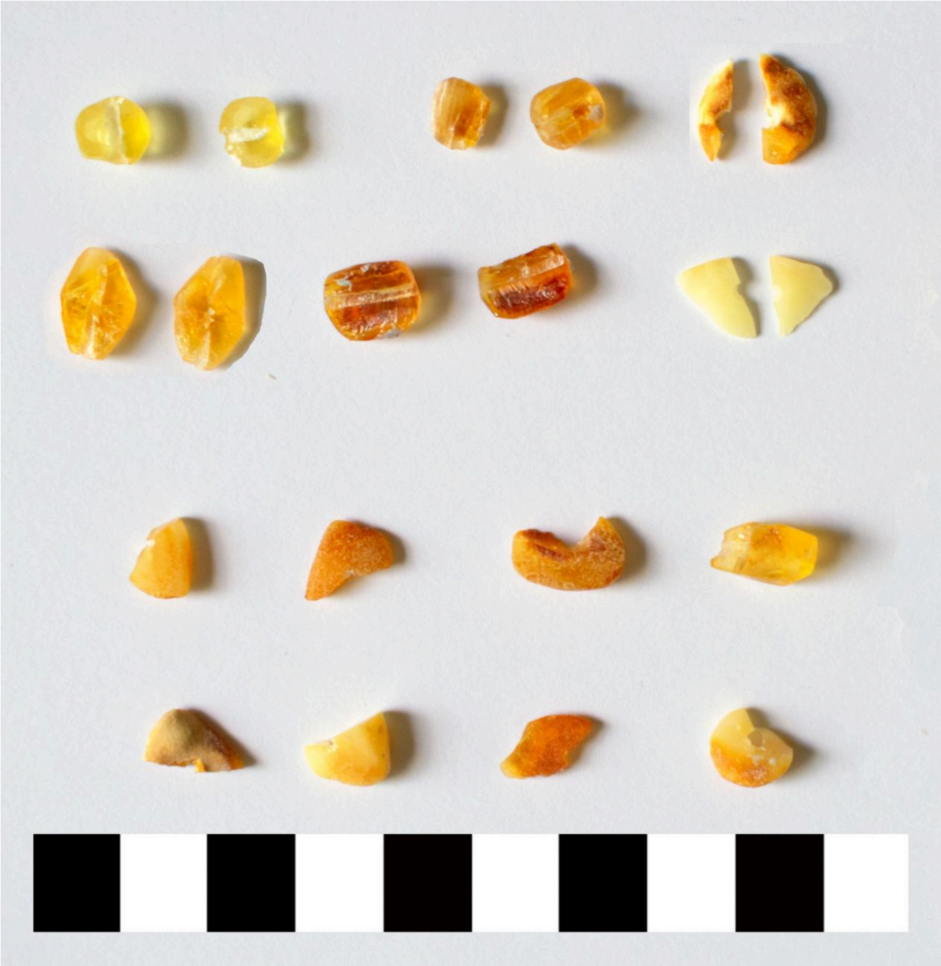
FIG 21. EXAMPLES OF BEADS THAT SPLIT DURING DRILLING. PHOTO BY KATIE HAWORTH.
