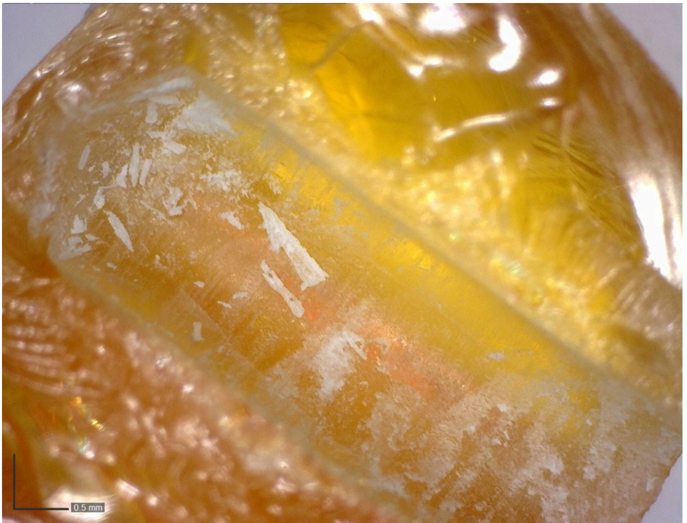
FIG 10. STRIATIONS WITHIN THE PERFORATION OF A FAILED REPLICA BEAD RESULTING FROM DRILLING USING A HANDHELD DRILL WITH A 2 MM BIT. PHOTO BY KATIE HAWORTH.
