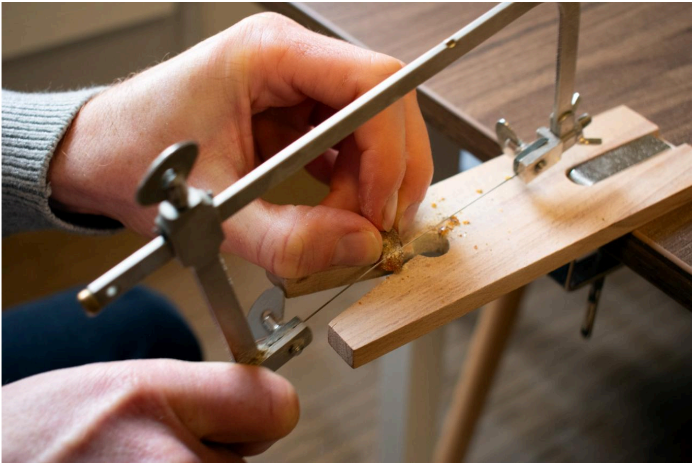
FIG 4. SAWING AMBER USING A JEWELLER'S SAW. PHOTO BY KATIE HAWORTH.
