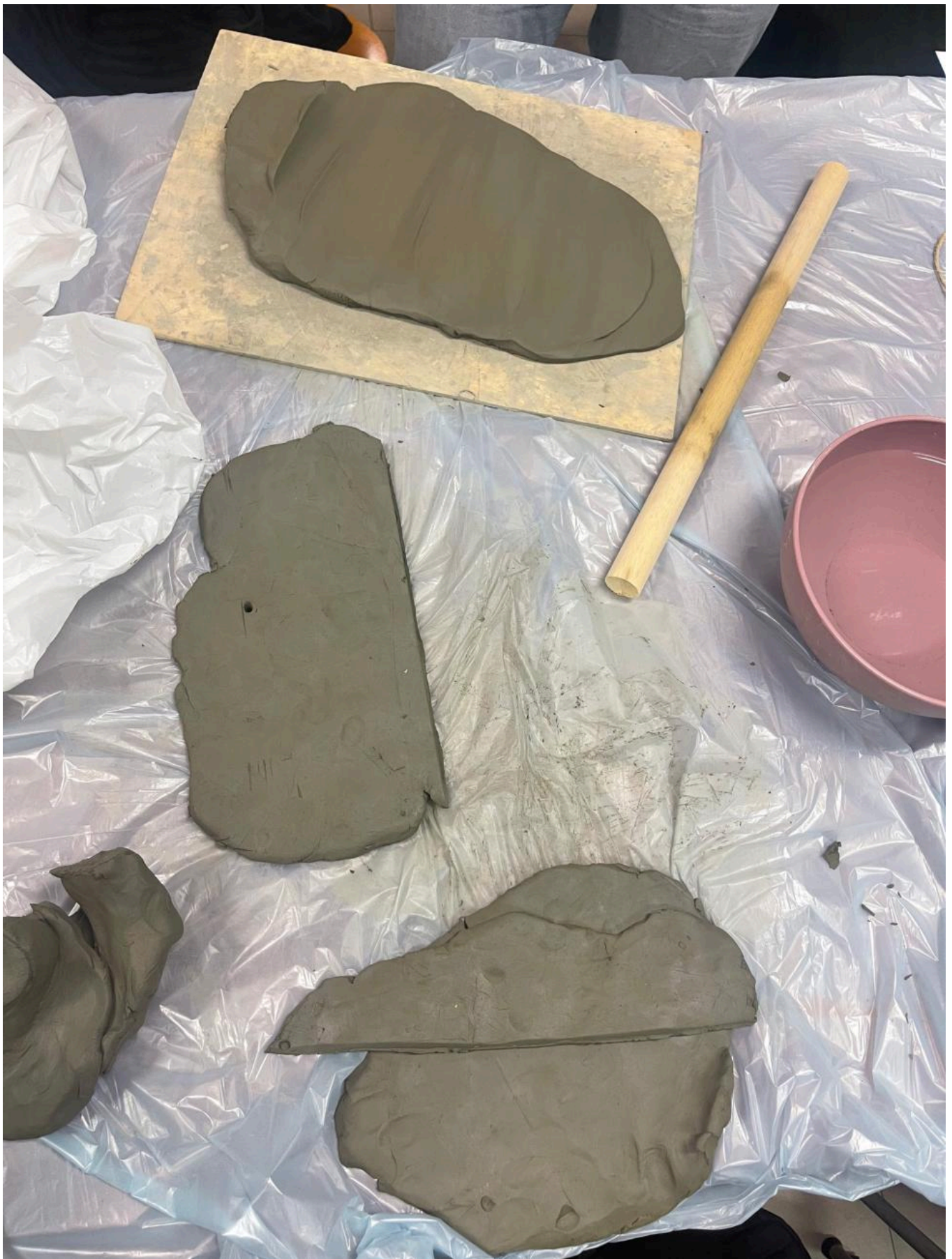
FIG 2. FIRST DAY OF EXPERIMENTATION. THE CLAY WAS PROCESSED AND ROLLED OUT WITH A ROLLING PIN TO A THICKNESS OF ABOUT 1 CM, AND FROM THIS HOMOGENEOUS PASTE THE TWELVE TABLETS WERE THEN CUT OUT. PHOTO BY AUTHORS.
