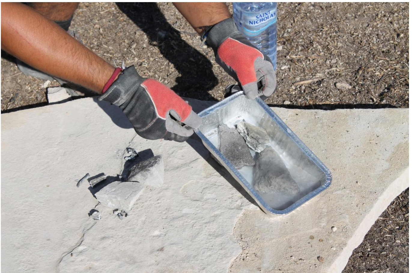
FIG 3. EXOTHERMIC REACTION OF THE LIMESTONE SAMPLES, WHICH WERE NOT FULLY CALCINATED. PHOTO BY AUTHORS.
