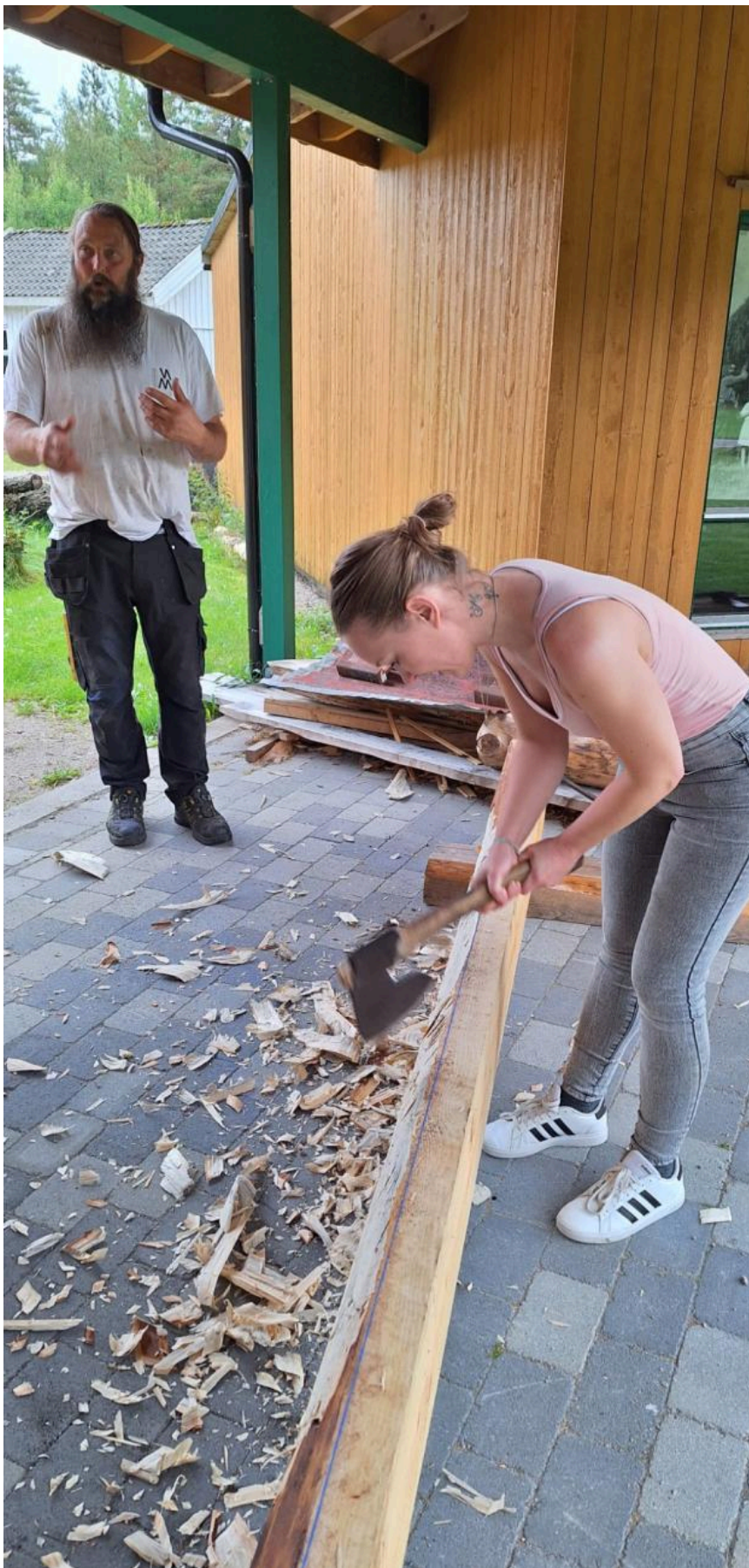
FIG 14. ØYVIND MAUREN IS INSTRUCTING AS A BEAM IS SHAPED USING AXES. PHOTO BY FREDRIK BJØNNES VESTFOLDMUSEENE
