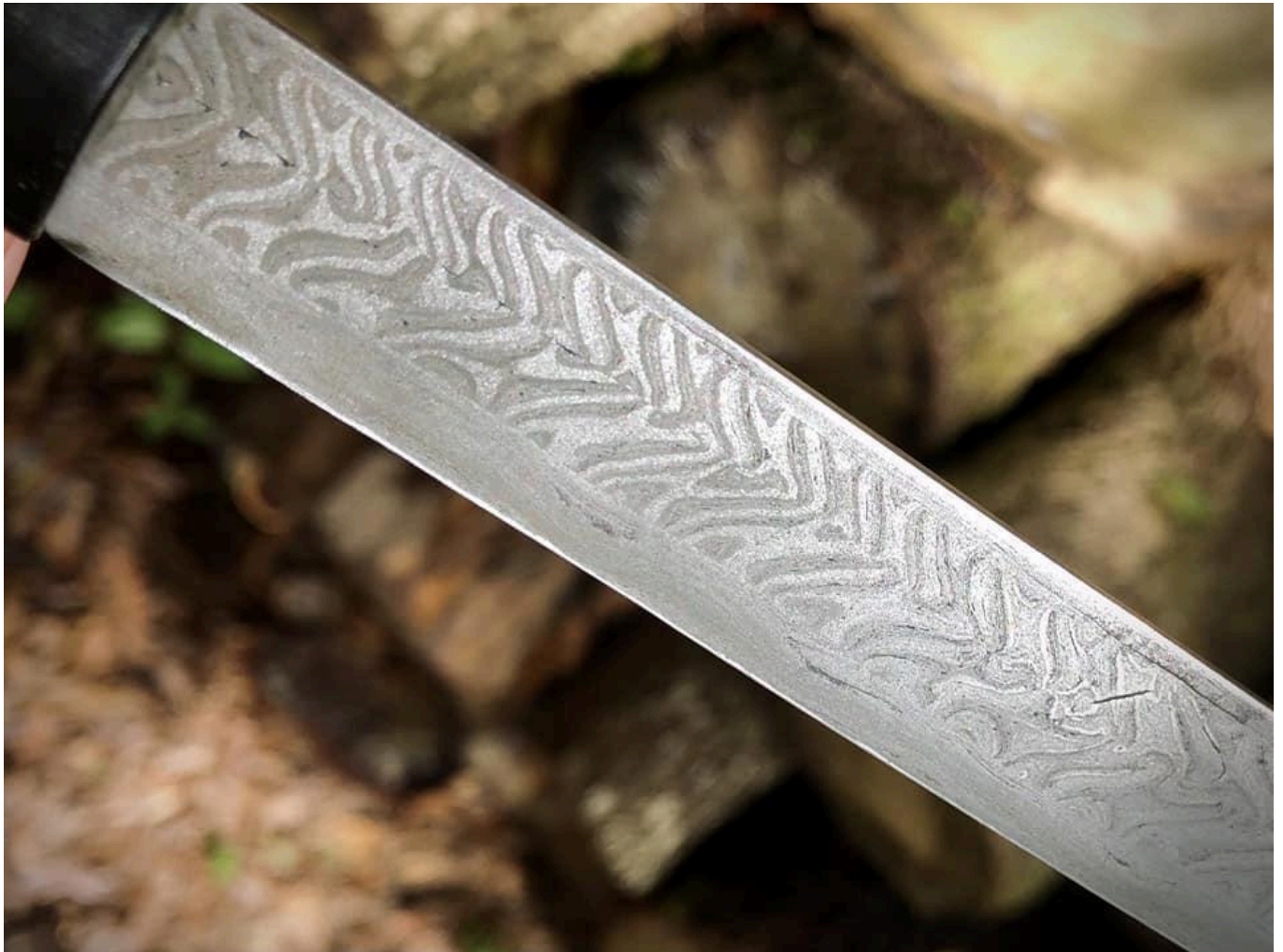
FIG 17. CONTEMPORARY PATTERN WELDED BLADE BY ANDREW WELTON, SHOWING CONTRAST BETWEEN LOW P BLOOMERY IRON AND HIGH P ANTIQUE WROUGHT IRON. (IMAGE USED WITH PERMISSION)
