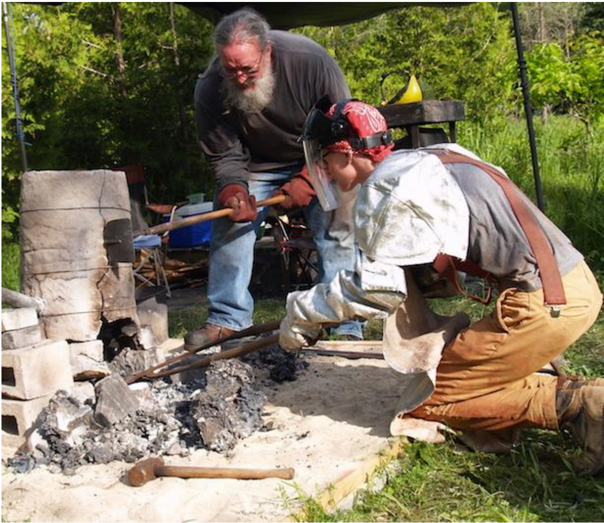
FIG 10. REY COGSWELL IN THE PROCESS OF BREAKING FREE THE BLOOM, NEIL PETERSON ASSISTING. PHOTO BY DARRELL MARKEWITZ
