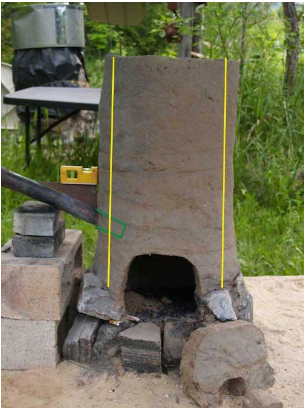
FIG 5. COMPLETED FURNACE SHOWING MOUNTING THE TUYERE, EXTRACTION AND TAPPING ARCHES. PHOTO BY DARRELL MARKEWITZ
