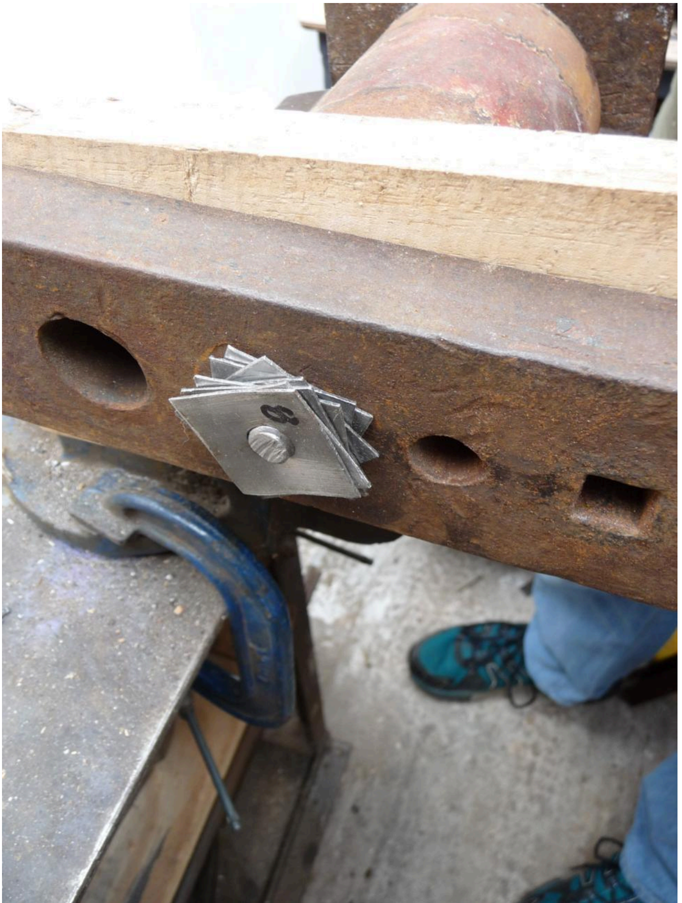
FIG 27. NUT MADE FROM THIN SHEETS OF IRON. PHOTO BY DAVID SIM
