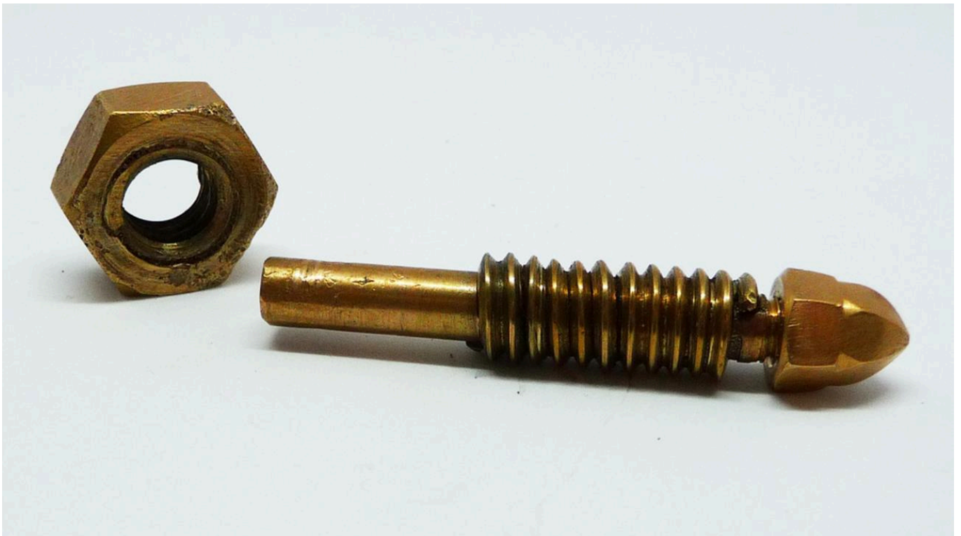
FIG 40. FABRICATED V-THREAD NUT AND BOLT. PHOTO BY DAVID SIM.
