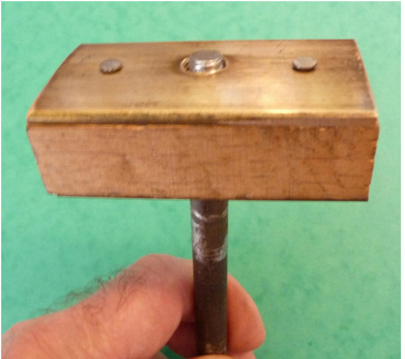
FIG 26. OAK NUT WITH BRASS PLATE REINFORCEMENT. PHOTO BY DAVID SIM.
