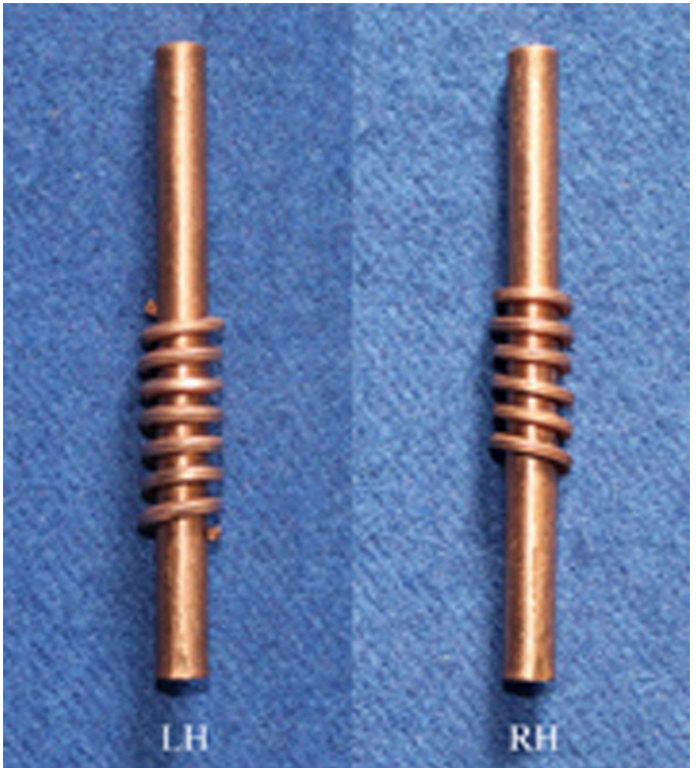
FIG 14. SHOWING LEFT AND RIGHT HAND THREADS. PHOTO BY DAVID SIM.
