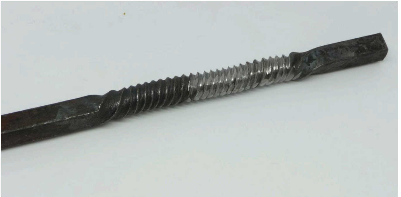
FIG 19. THREAD MADE BY TWISTING AND FILING. PHOTO BY DAVID SIM.
