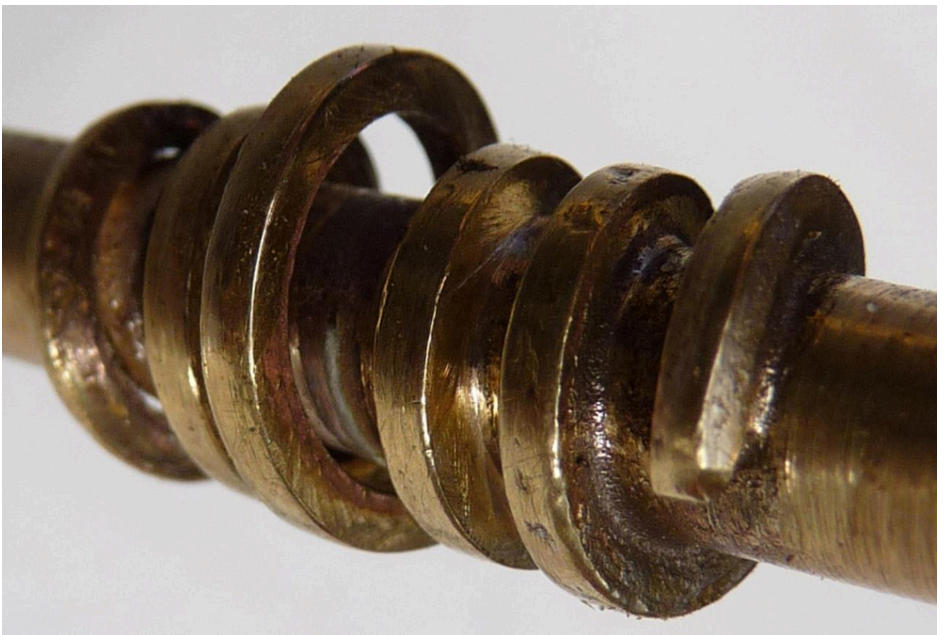
FIG 38. BROKEN BRASS THREAD. PHOTO BY DAVID SIM
