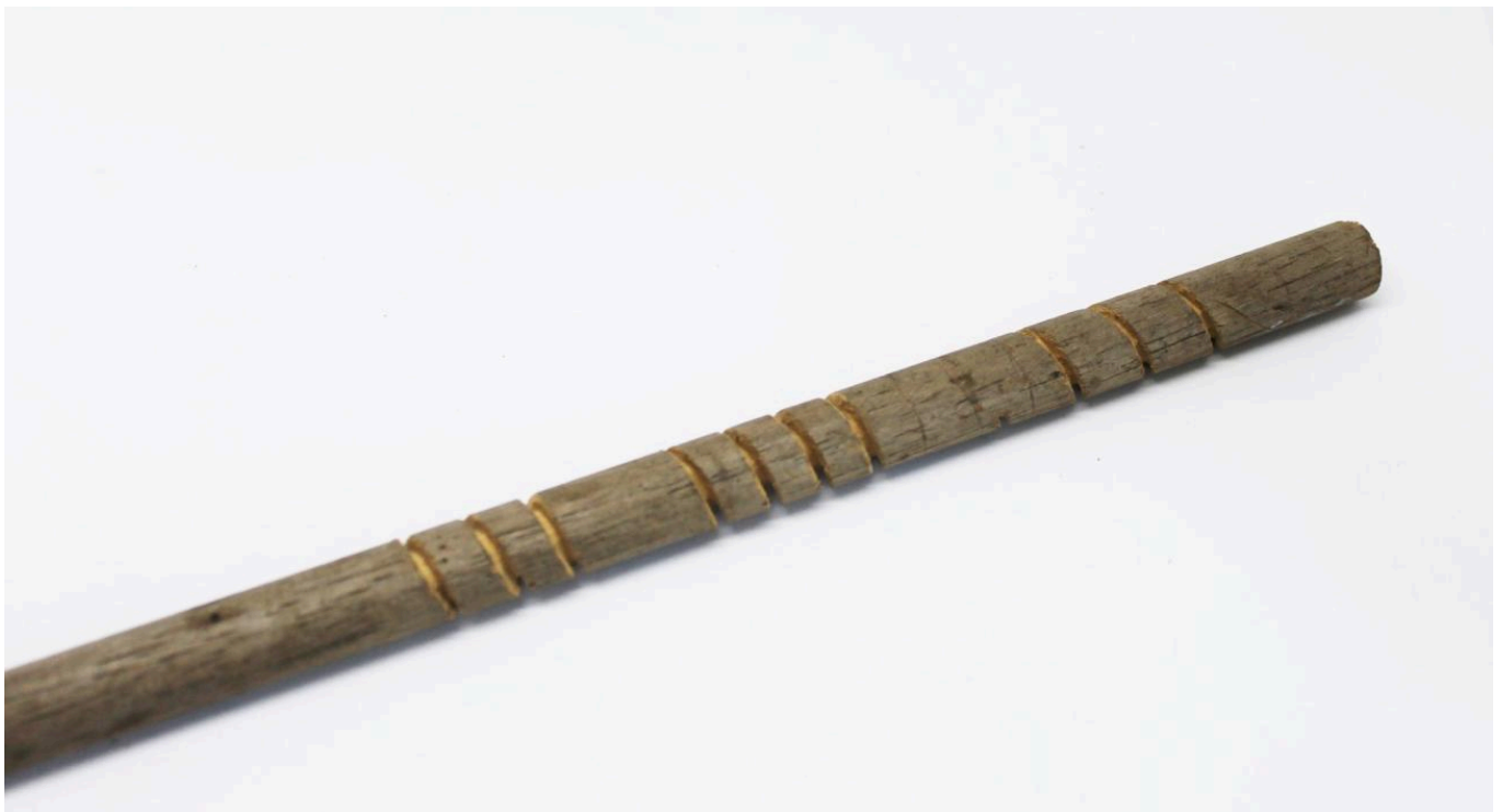
FIG 16. SQUARE THREADS CUT USING A MITER BLOCK. PHOTO BY DAVID SIM.
