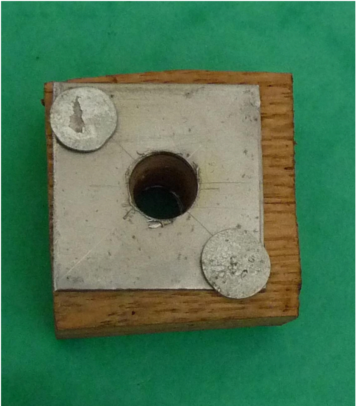
FIG 25. OAK NUT WITH IRON PLATE ENFORCEMENT. PHOTO BY DAVID SIM.
