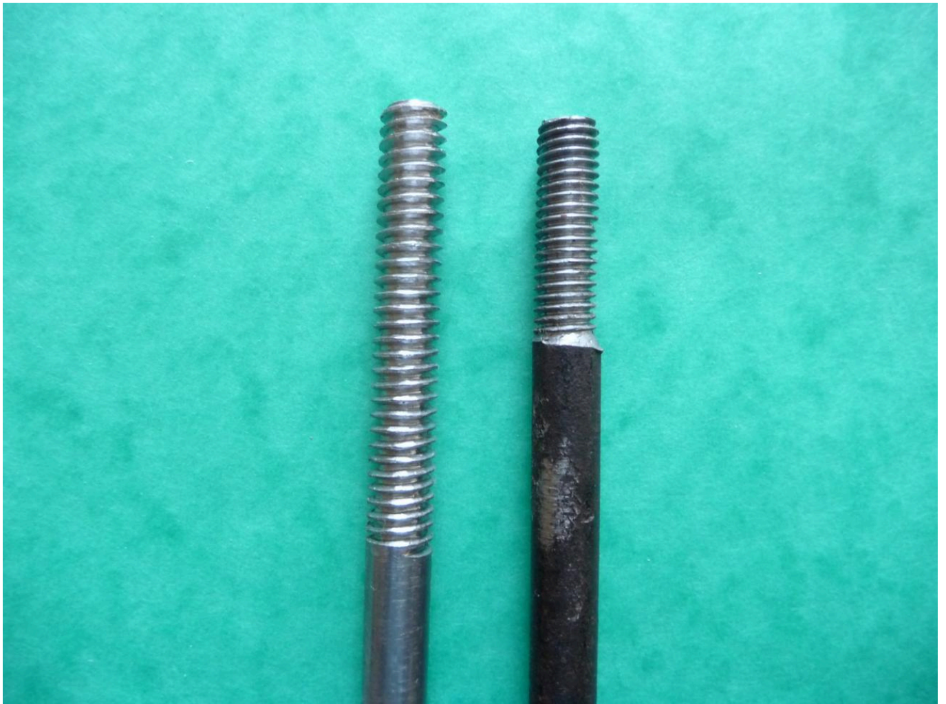
FIG 21. THREAD CUT BY HAND (LEFT) AND THREAD CUT USING A DIE (RIGHT). PHOTO BY DAVID SIM.
