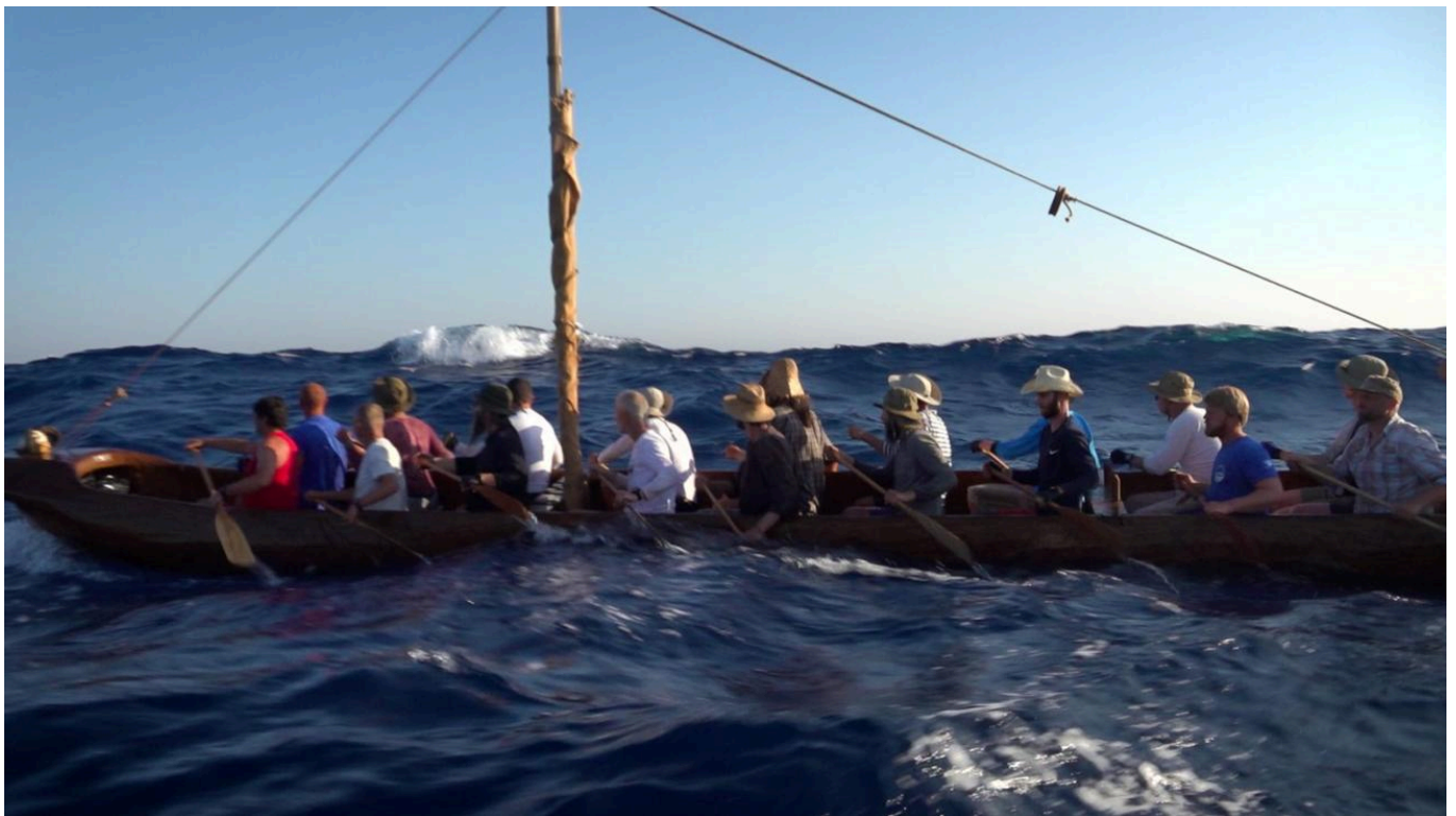
FIG 7B. TYPE 2 HIGH AND LONG SIDE WAVES: THEY ALLOW FOR EASIER NAVIGATION THAN HEADWAVES. IT IS POSSIBLE TO DELIBERATELY 'SURF' THE WAVES. PHOTO BY EXPEDITION MONOXYLON ARCHIVE.
