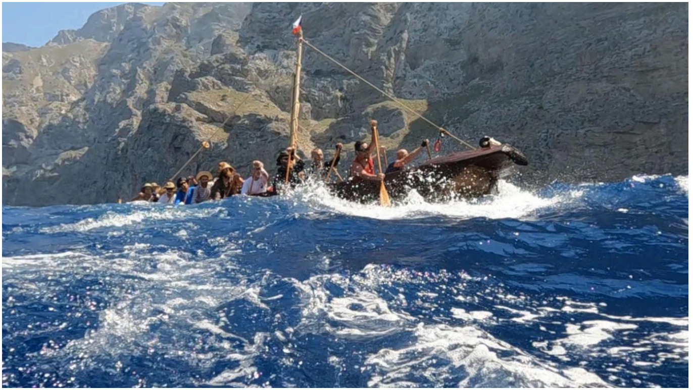
FIG 9B. TYPE 4 SIDE-HEAD WAVES: THEY CONSIDERABLE SLOW THE VESSEL BUT LESS THAN HEADWAVES. PHOTO BY EXPEDITION MONOXYLON ARCHIVE.
