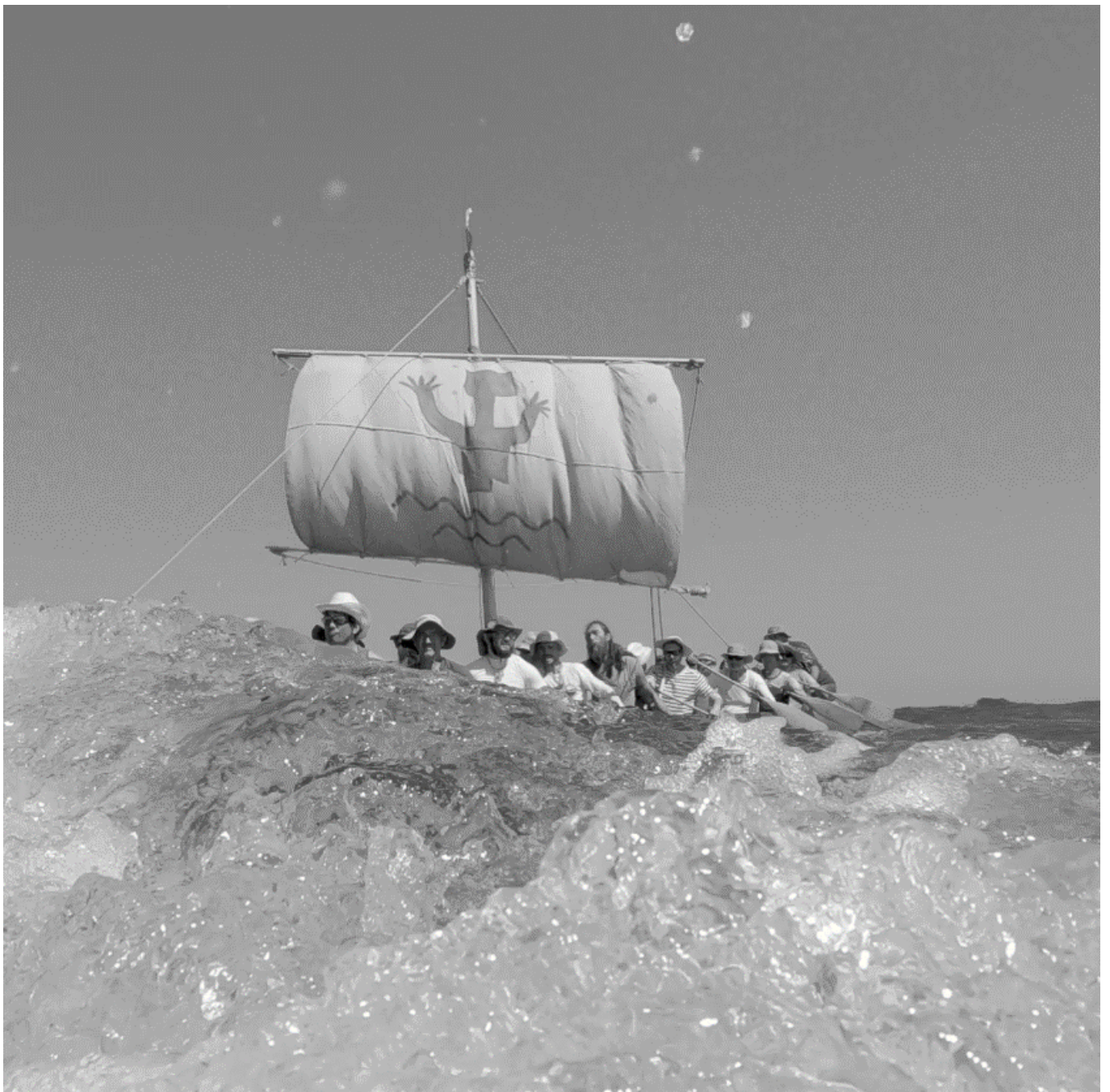
FIG 10B. TYPE 5 BACK HIGH WAVES: THEY CREATE AN IMPRESSION THAT THEY PROPEL THE VESSEL BUT THEY CAN MAKE THE VESSEL UNCONTROLLABLE. PHOTO BY EXPEDITION MONOXYLON ARCHIVE.
