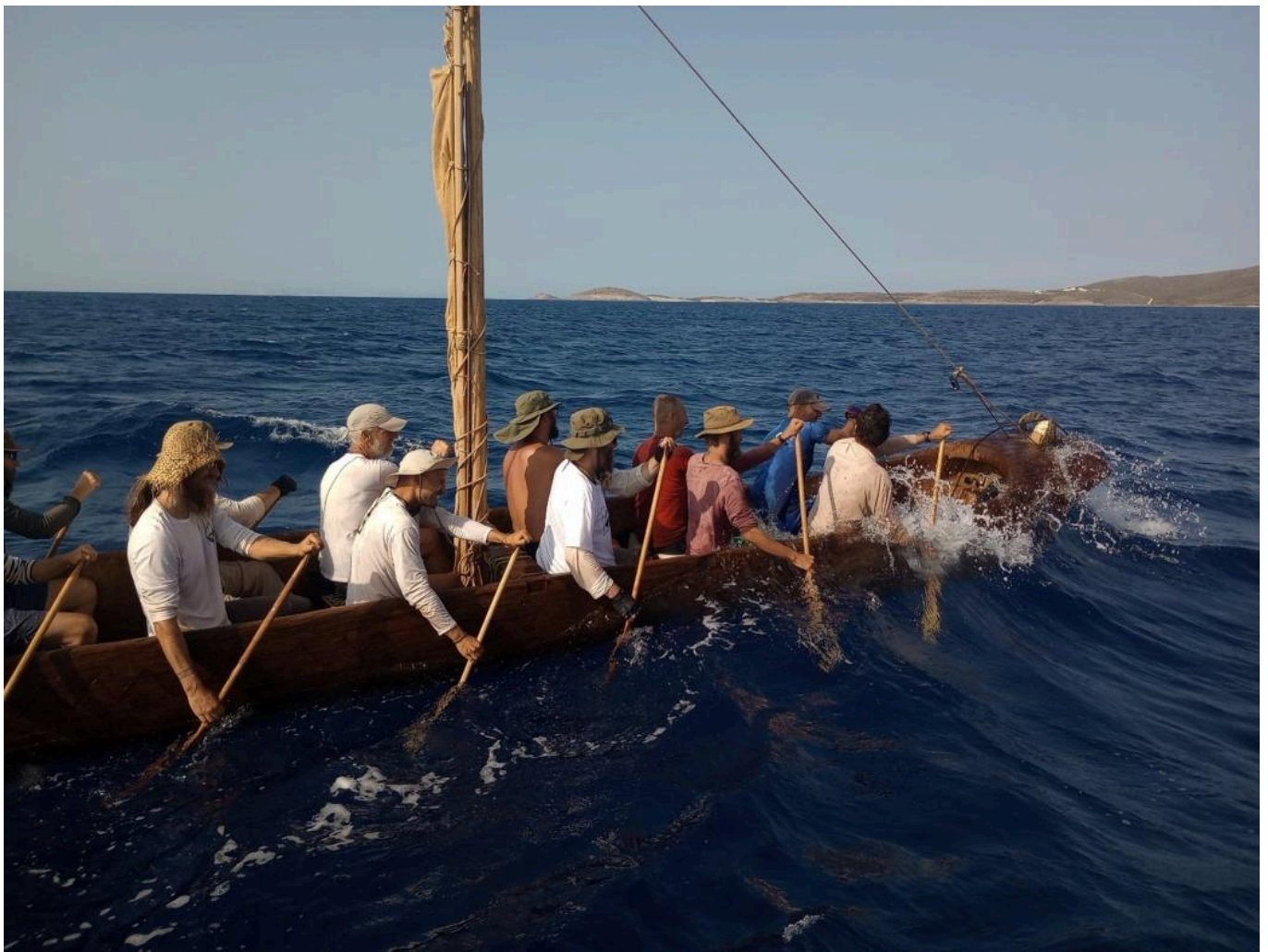
FIG 6B. TYPE 1 SHORT SIDE WAVES: THERE IS A DANGER OF OCCASIONAL FLOODING OF THE BOAT BUT THE VESSEL DOES NOT LOSE SPEED. PHOTO BY EXPEDITION MONOXYLON ARCHIVE.
