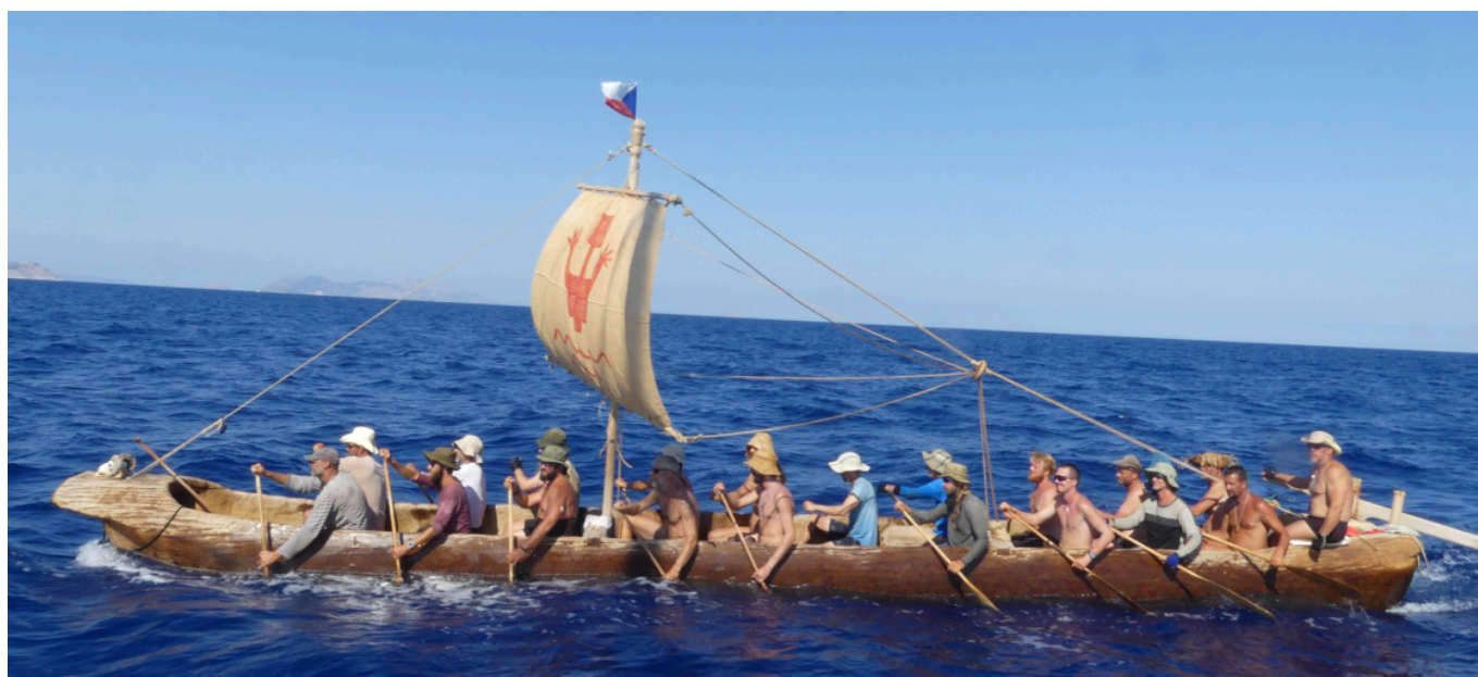
FIG 12B. TYPE 7 SIDE AND FOLLOWING WIND ON OPEN SEA: IF THE WIND IS NOT TOO STRONG, THE WAVES DO NOT FLOOD THE VESSEL AND THE WIND MIGHT BE USED FOR SAILING. PHOTO BY EXPEDITION MONOXYLON ARCHIVE.
