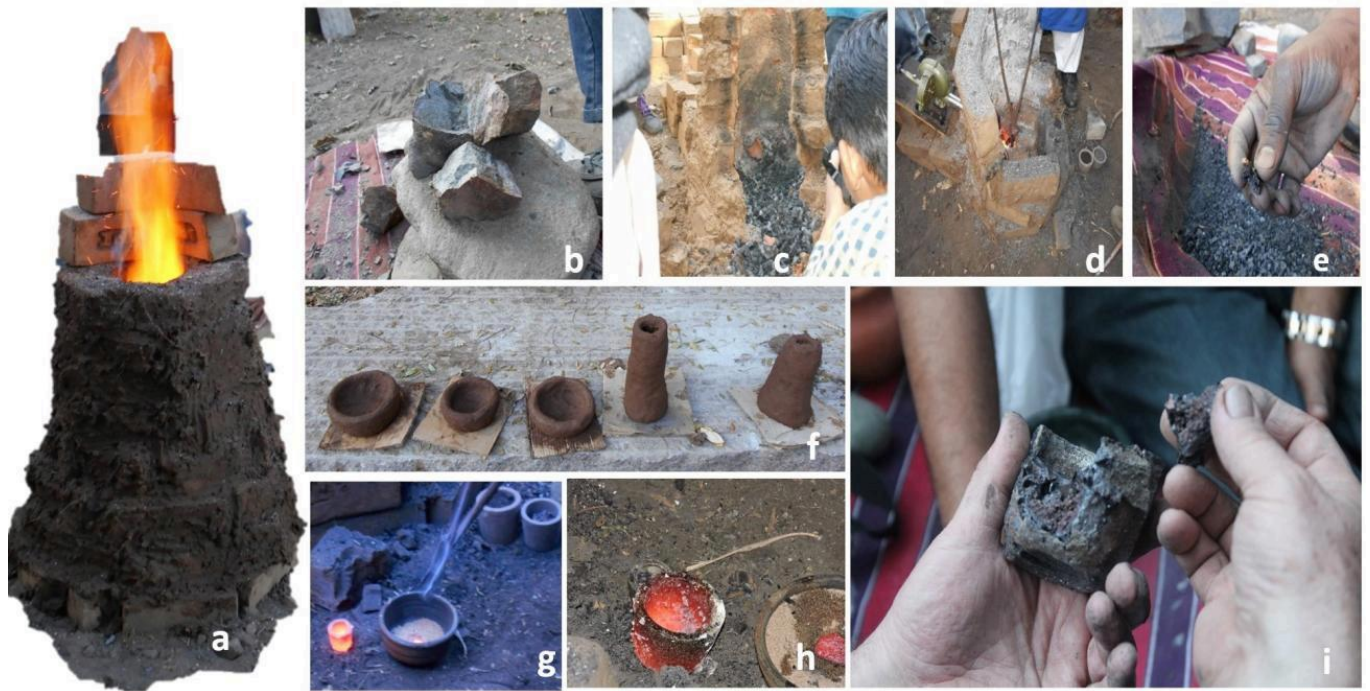
FIG 7. A COPPER SMELTING FURNACE. B. COPPER ORE C. DISMANTLED FURNACE FOR COLLECTING MOLTEN METAL FROM ORE. D. COLLECTION OF METALLIC FRAGMENTS FROM CRUCIBLE. E. OXIDIZED ORE F. CLAY TYERS FOR FURNACE G. POURED MOLTEN COPPER OVER SAND. H. CRUCIBLES. I. BROKEN CRUCIBLE AFTER MELTING THE COPPER. PHOTO BY GARIMA SINGH
