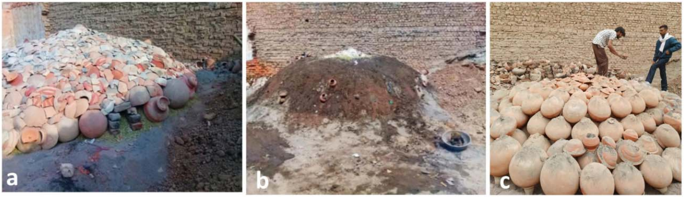
FIG 10-1. A. POTTERY KILN COVERED WITH BROKEN POTSHERD. B. KILN AFTER PLASTERED WITH CLAY C. POTS AFTER FIRING. PHOTO BY GARIMA SINGH
