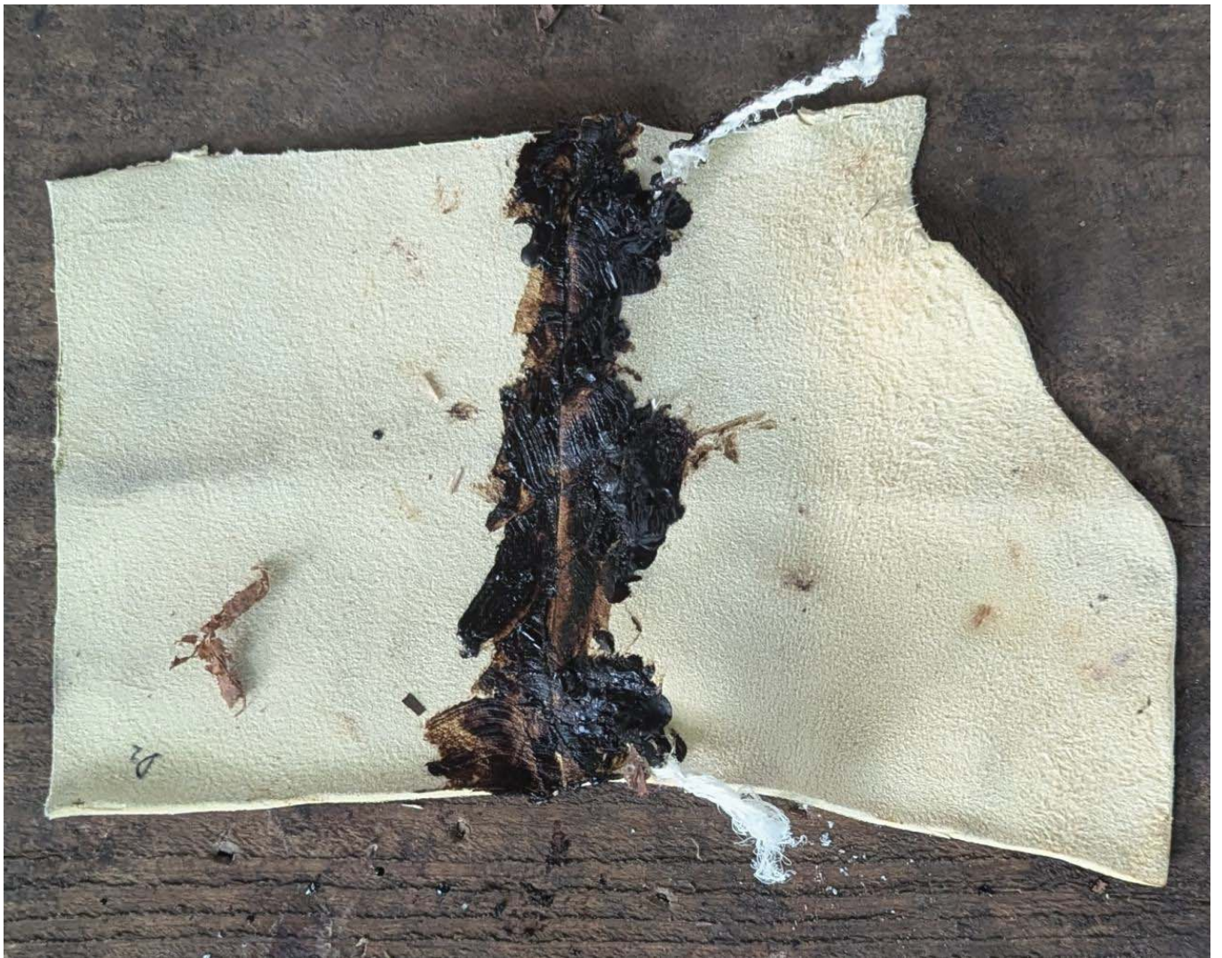
FIG 12D. THE 8 SAMPLES USED IN THE EXPERIMENT (EXCEPT CONTROLS) RIGHT AFTER ADHESIVES' APPLICATION (1 SIDE ONLY). PHOTO BY ELEONORA SCANDOLA.
