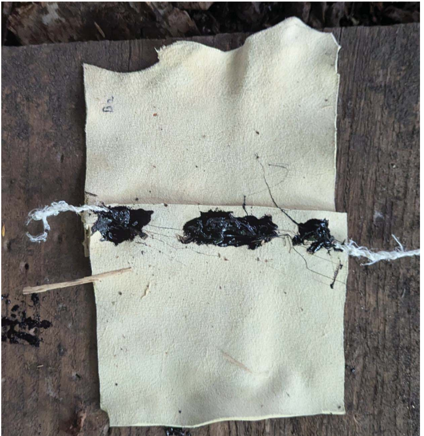
FIG 12B. THE 8 SAMPLES USED IN THE EXPERIMENT (EXCEPT CONTROLS) RIGHT AFTER ADHESIVES' APPLICATION (1 SIDE ONLY). PHOTO BY ELEONORA SCANDOLA.
