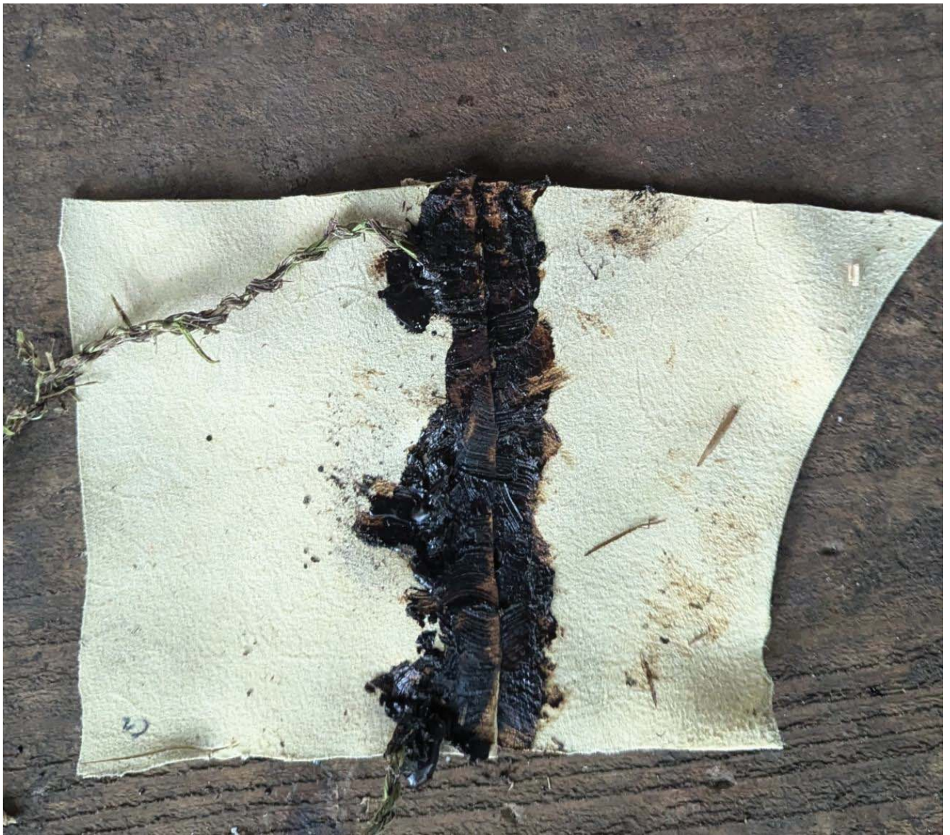
FIG 12C. THE 8 SAMPLES USED IN THE EXPERIMENT (EXCEPT CONTROLS) RIGHT AFTER ADHESIVES' APPLICATION (1 SIDE ONLY). PHOTO BY ELEONORA SCANDOLA.
