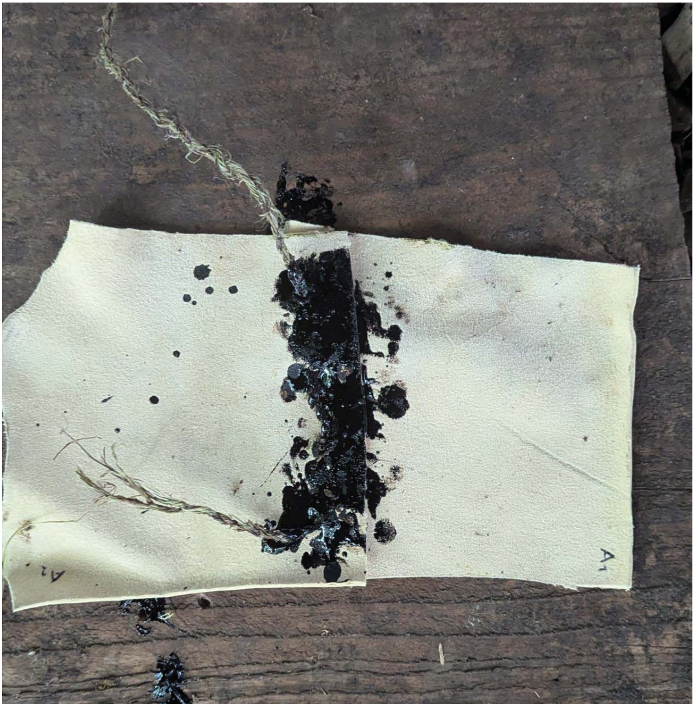
FIG 12A. THE 8 SAMPLES USED IN THE EXPERIMENT (EXCEPT CONTROLS) RIGHT AFTER ADHESIVES' APPLICATION (1 SIDE ONLY). PHOTO BY ELEONORA SCANDOLA.
