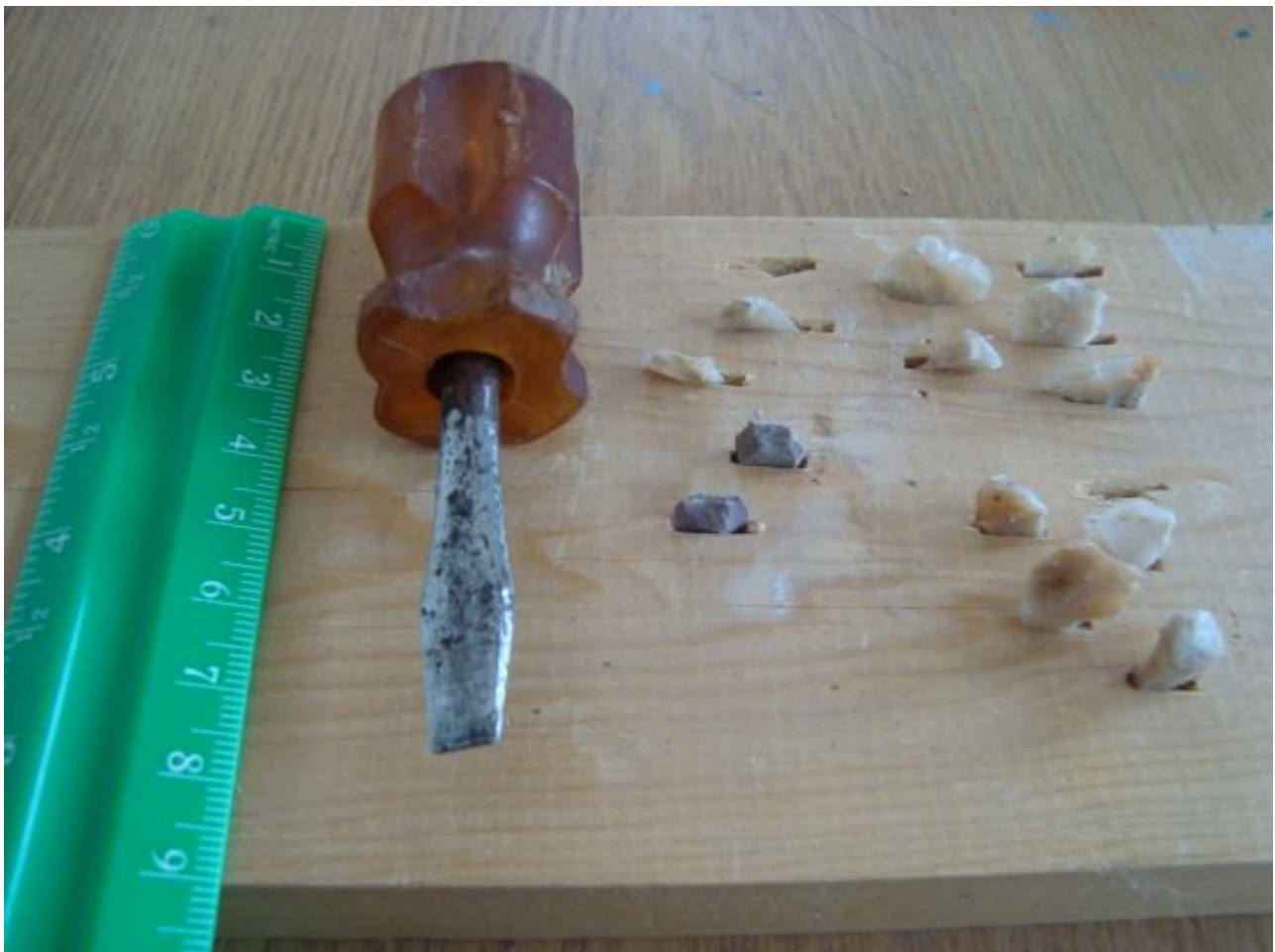
FIG 7. FIRST ATTEMPTS TO INSERT FLAKES IN MY EXPERIMENTAL BOARD. THOSE ON THE RIGHT ARE TOO BIG AND POORLY FITTED; THOSE ON THE LEFT ARE APPROACHING A SATISFACTORY STANDARD. PHOTO J. WHITTAKER
