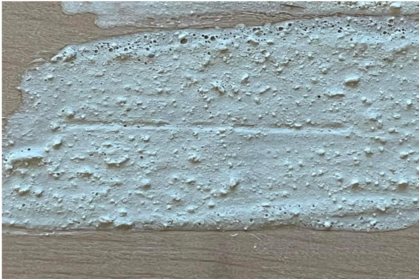
FIG 12. WHITE GROUND OVER INCISION WITH A WIDTH OF 1 MM. PHOTO: A.V. GELSKOV
