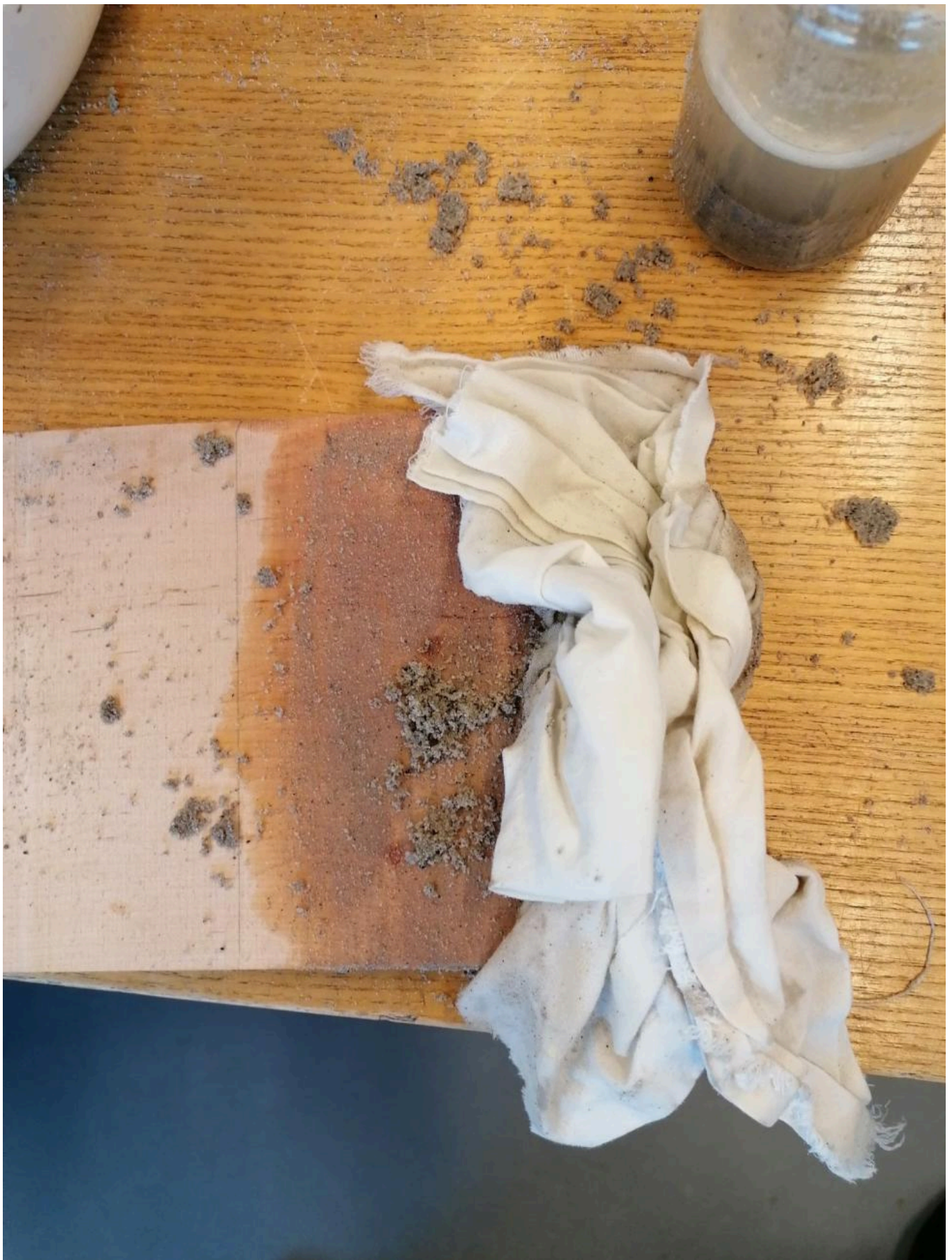
FIG 7. THE WOOD GETS WET BY THIS METHOD AND NEEDS TO DRY BEFORE FURTHER PROCESSING, AS THE WET SANDING CLEARLY RUINS THE SURF. PHOTO: C. RELAND
