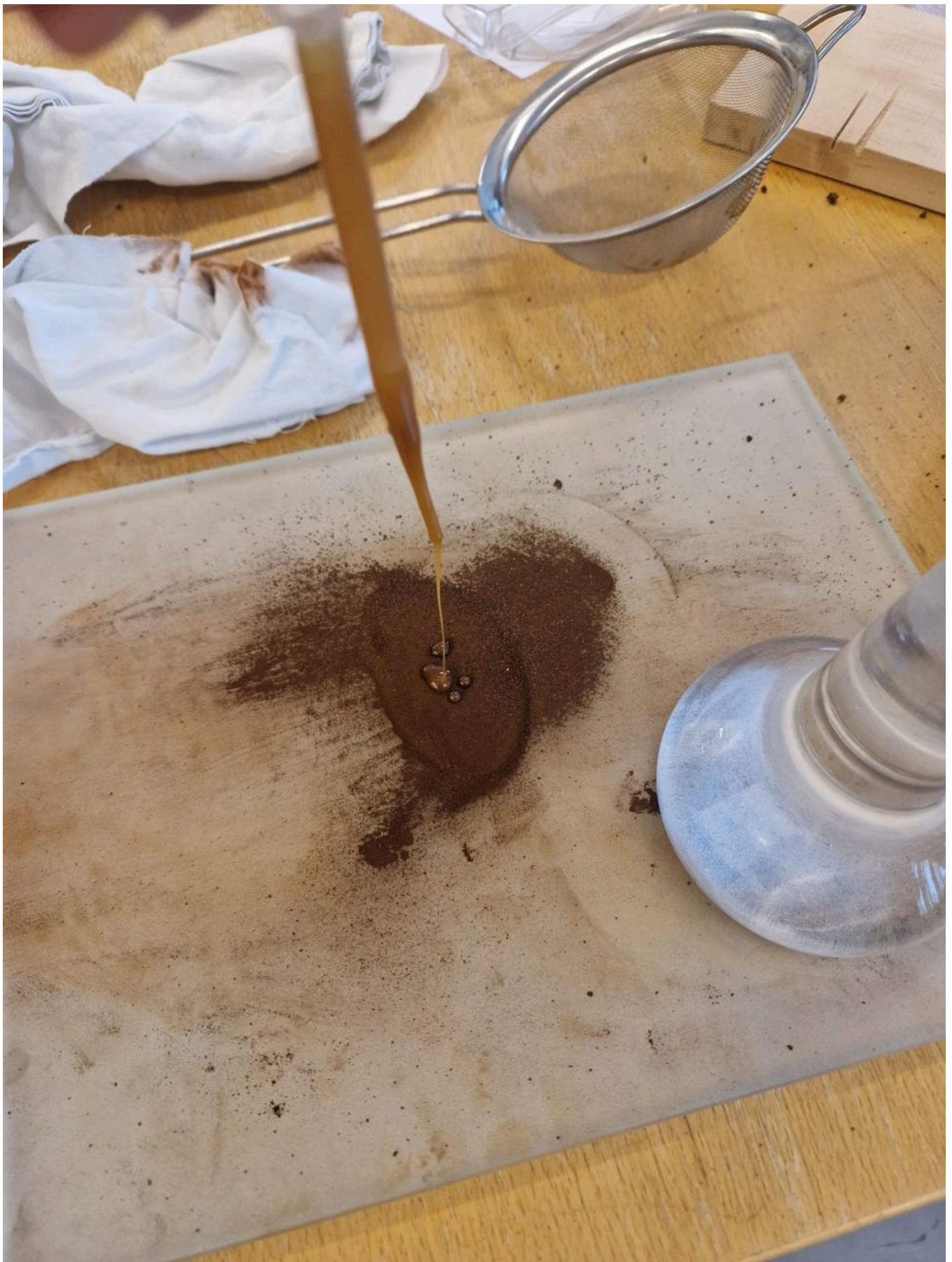
FIG 15. LINSEED OIL MIXED INTO POWDER MADE FROM FRESHLY GRINDED IRON ORE. PHOTO: S.L. ANDERSEN.
