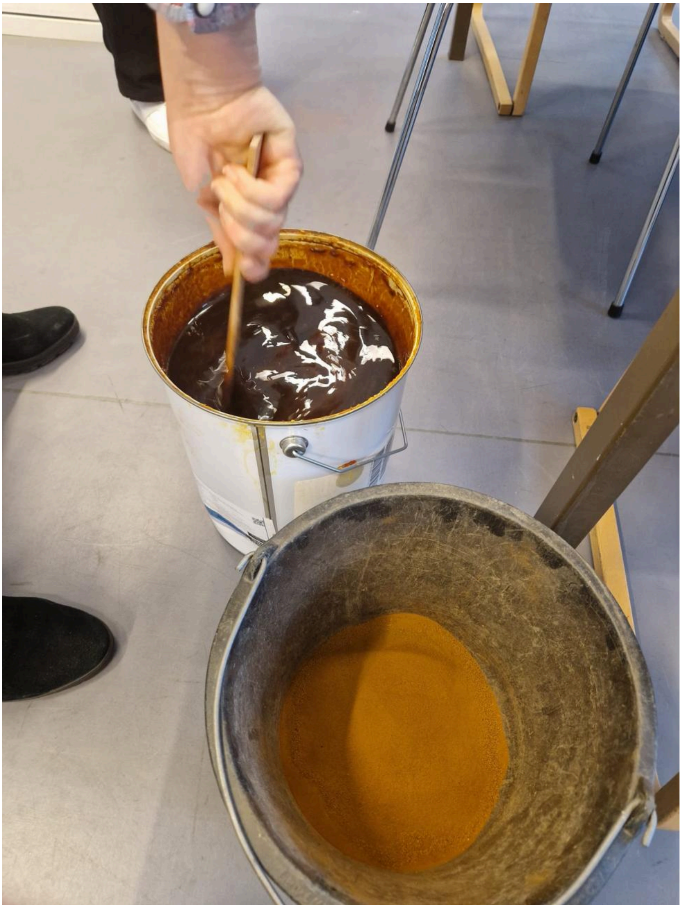
FIG 14. LINSEED OIL AND IRON ORE FOR PIGMENTATION. PHOTO: S.L. ANDERSEN
