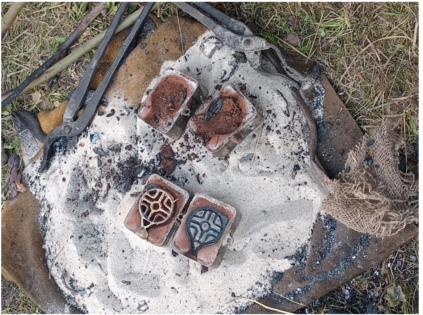
FIG 4. PENDANT CAST IN SAND. PHOTO BY E. GIOVANNA FREGNI
