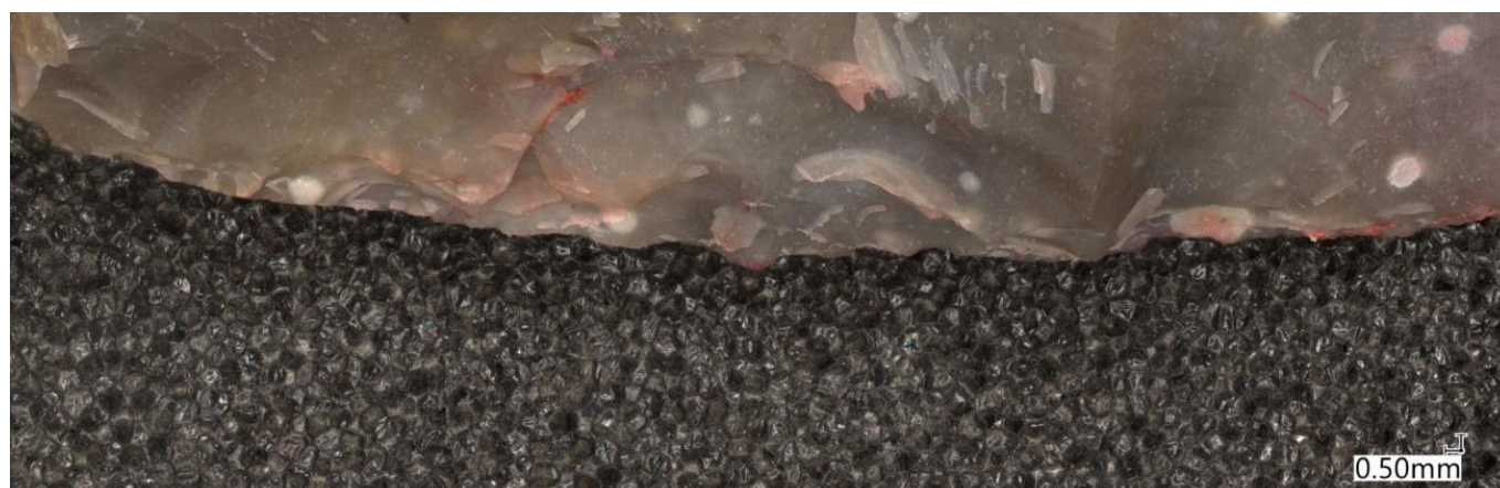
FIG 1. EDGE OF EXPERIMENTAL TOOL SHOWING HIGH DENSITY OF 'MICRO-NICHES' TERMINATIONS (20X). SOURCE: WHITEHEAD
