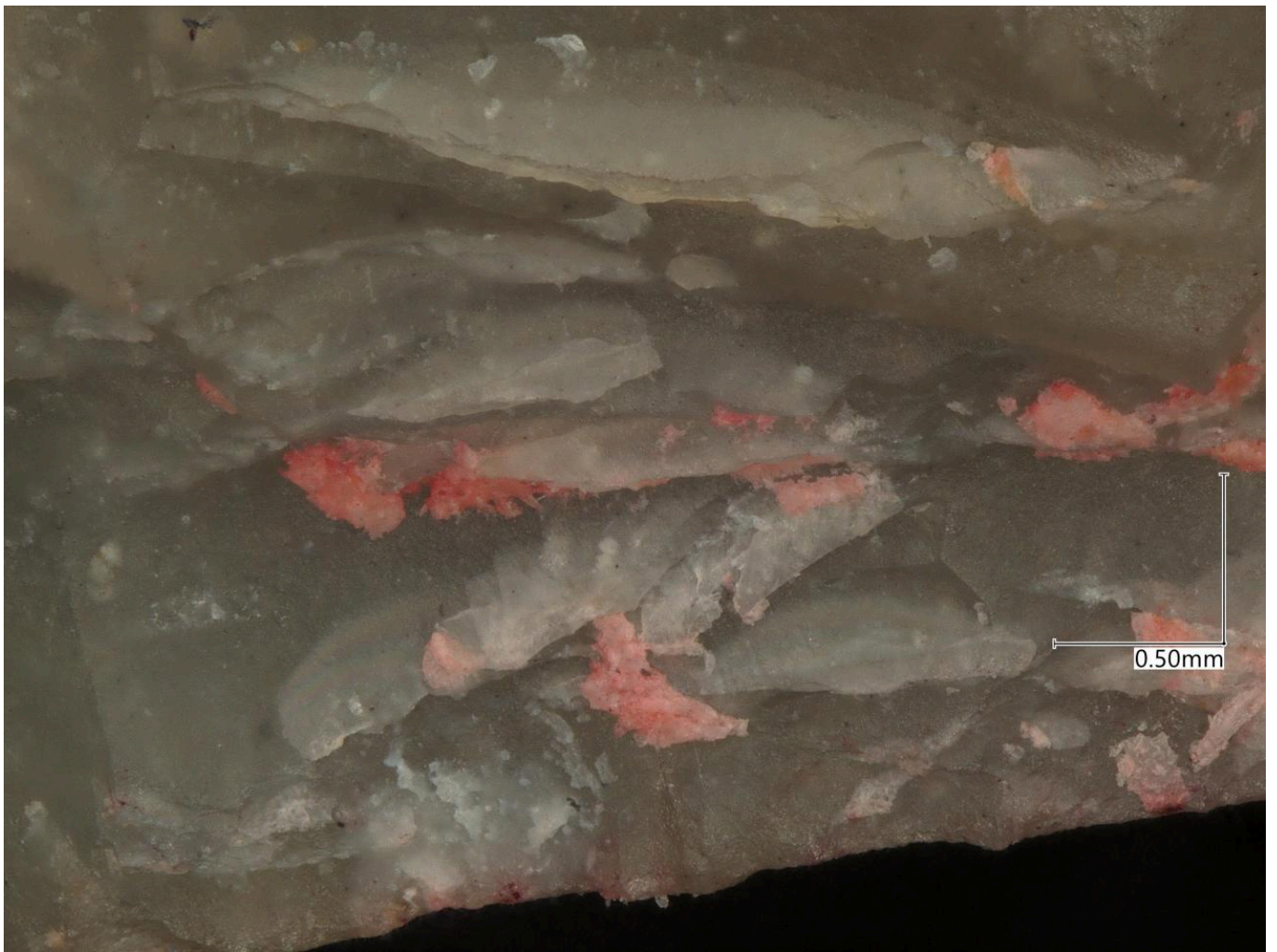
FIG 2C. CLOSE-UP VIEW OF EDGE WITH HIGH AMOUNTS OF FISSURATED FLAKES AND ADHERENT BIOLOGICAL MATTER (80X). SOURCE: WHITEHEAD
