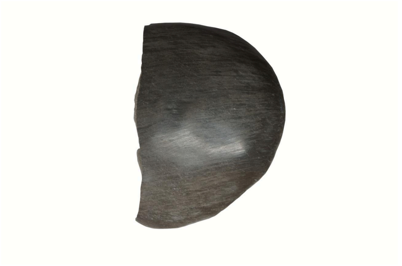
FIG 6B. LINEAR BURNISHING MARKS ON THE SURFACE OF THE UNFIRED TEST SHERD FROM THE CRETAN CLAY. PHOTO BY NIKOS GERAKAKIS
