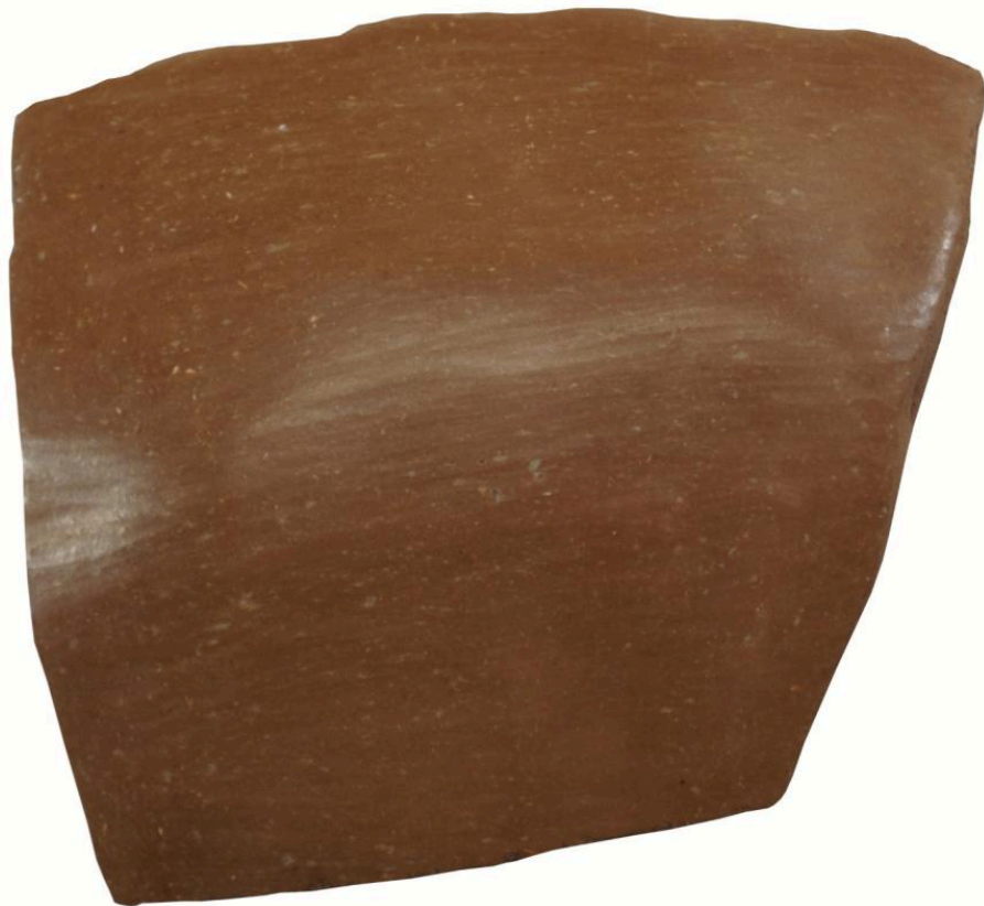
FIG 17A. TEST SHERD FROM THE CRETAN CLAY FIRED AT 700° C/3 MIN IN A FHR CONTROLLED FIRING. PHOTO BY NIKOS GERAKAKIS
