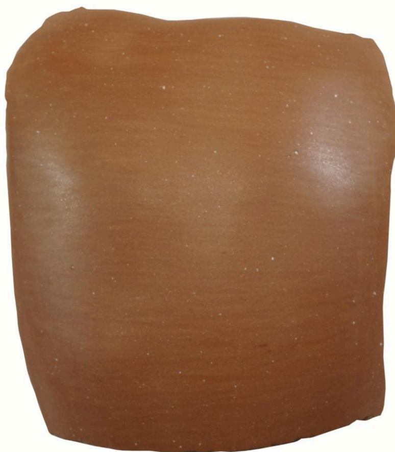
FIG 16C. TEST SHERD FROM THE EUBOEAN CLAY FIRED AT 900° C/3 MIN IN A FHR CONTROLLED FIRING. PHOTO BY NIKOS GERAKAKIS
