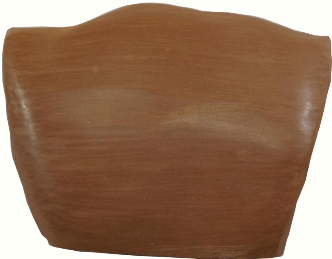
FIG 16A. TEST SHERD FROM THE EUBOEAN CLAY FIRED AT 700° C/3 MIN IN A FHR CONTROLLED FIRING. PHOTO BY NIKOS GERAKAKIS
