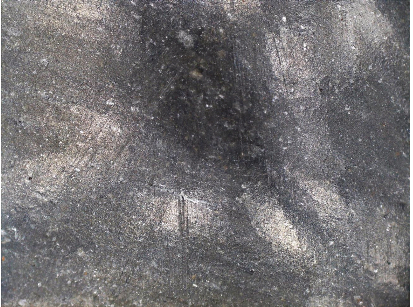
FIG 7B. CHARACTERISTIC BURNISHING STRIATIONS, AS OBSERVED UNDER A DIGITAL HANDHELD MICROSCOPE: FIELD OF VIEW 1.1 CM. PHOTO BY GEORGIA KORDATZAKI
