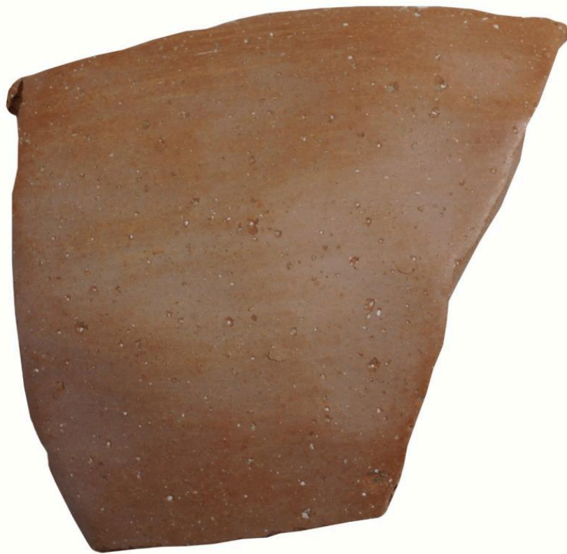
FIG 21C. TEST SHERD FROM THE CRETAN CLAY FIRED AT 1000° C/3 MIN IN A VSHR CONTROLLED FIRING. THE SHERD SHOWED EARLY LIME SPALLING. PHOTO BY NIKOS GERAKAKIS
