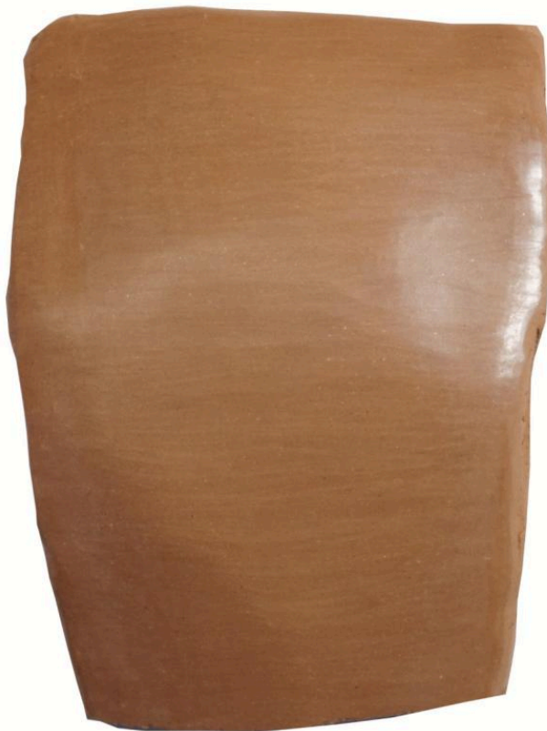
FIG 20A. TEST SHERD FROM THE EUBOEAN CLAY FIRED AT 700° C/3 MIN IN A VSHR CONTROLLED FIRING. PHOTO BY NIKOS GERAKAKIS
