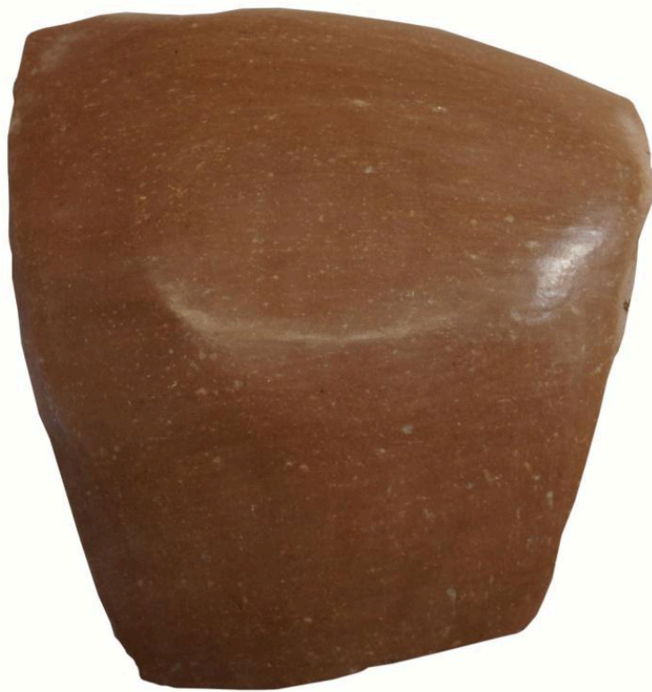
FIG 21A. TEST SHERD FROM THE CRETAN CLAY FIRED AT 700° C/3 MIN IN A VSHR CONTROLLED FIRING. PHOTO BY NIKOS GERAKAKIS
