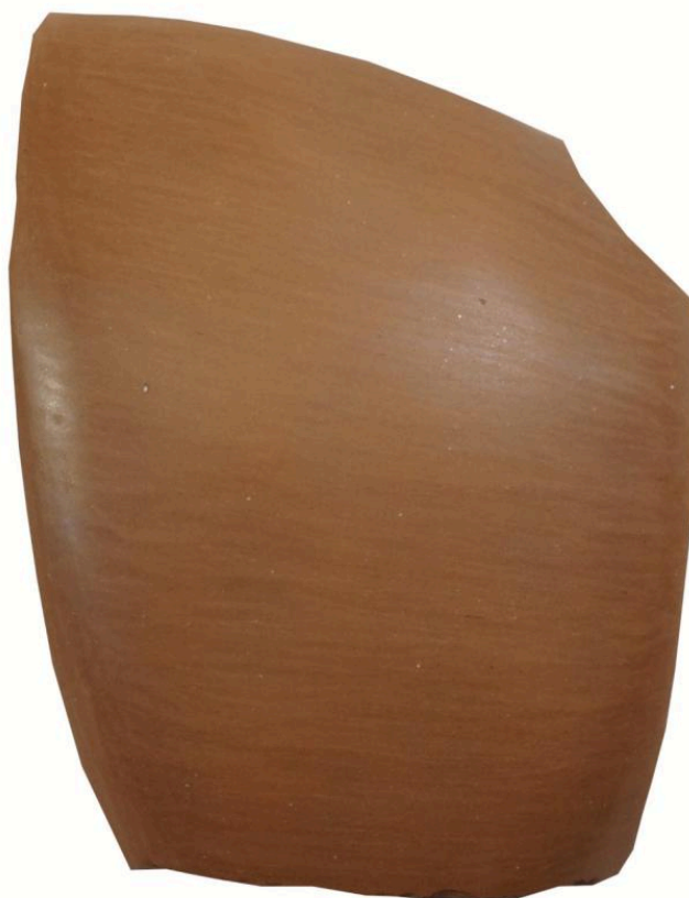
FIG 18B. TEST SHERD FROM THE EUBOEAN CLAY FIRED AT 800° C/1 H IN A FHR CONTROLLED FIRING. PHOTO BY NIKOS GERAKAKIS
