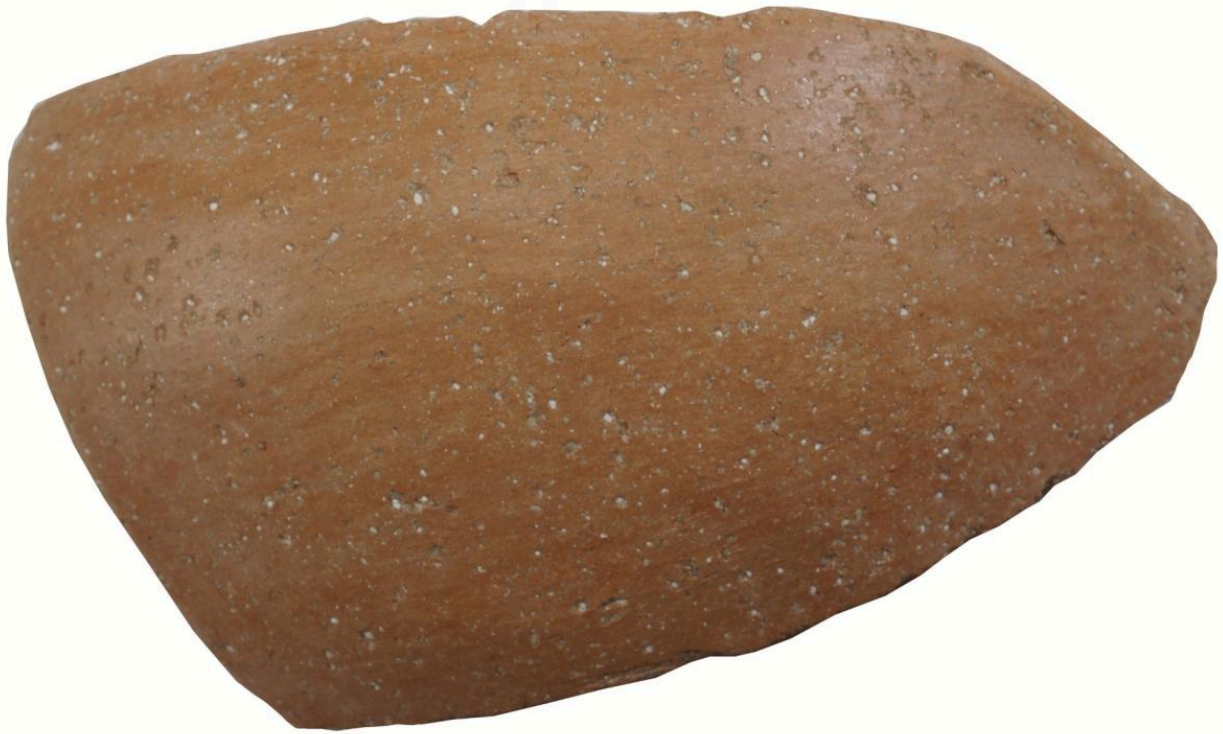
FIG 17D. TEST SHERD FROM THE CRETAN CLAY FIRED AT 1000° C/3 MIN IN A FHR CONTROLLED FIRING. THE SHERD SHOWED ADVANCED LIME SPALLING. PHOTO BY NIKOS GERAKAKIS
