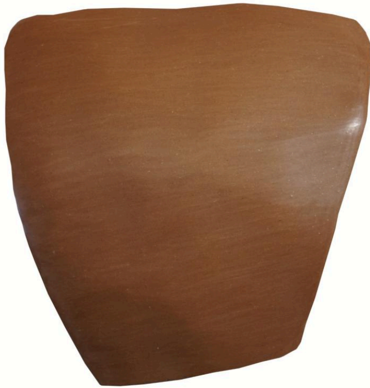
FIG 20B. TEST SHERD FROM THE EUBOEAN CLAY FIRED AT 800° C/3 MIN IN A VSHR CONTROLLED FIRING. PHOTO BY NIKOS GERAKAKIS
