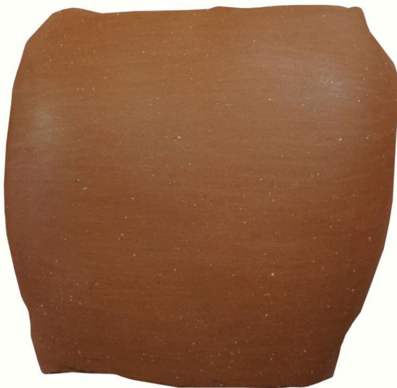
FIG 18D. TEST SHERD FROM THE EUBOEAN CLAY FIRED AT 1000° C/1 H IN A FHR CONTROLLED FIRING. PHOTO BY NIKOS GERAKAKIS
