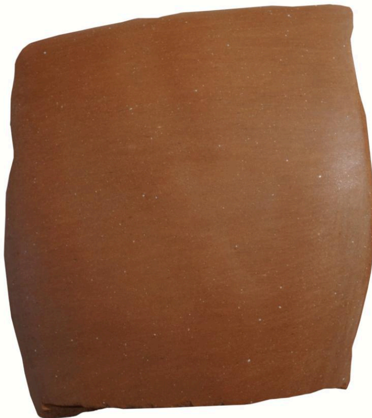
FIG 20C. TEST SHERD FROM THE EUBOEAN CLAY FIRED AT 1000° C/3 MIN IN A VSHR CONTROLLED FIRING. PHOTO BY NIKOS GERAKAKIS
