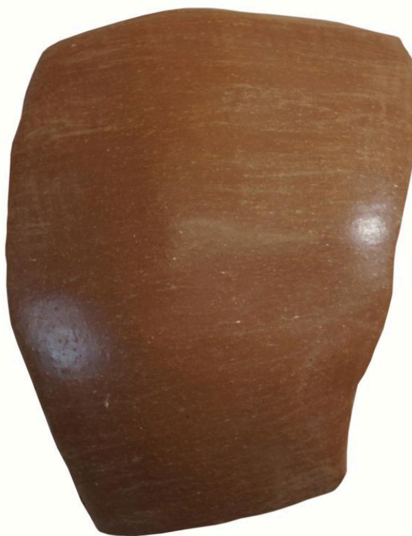
FIG 21B. TEST SHERD FROM THE CRETAN CLAY FIRED AT 800° C/3 MIN IN A VSHR CONTROLLED FIRING. PHOTO BY NIKOS GERAKAKIS
