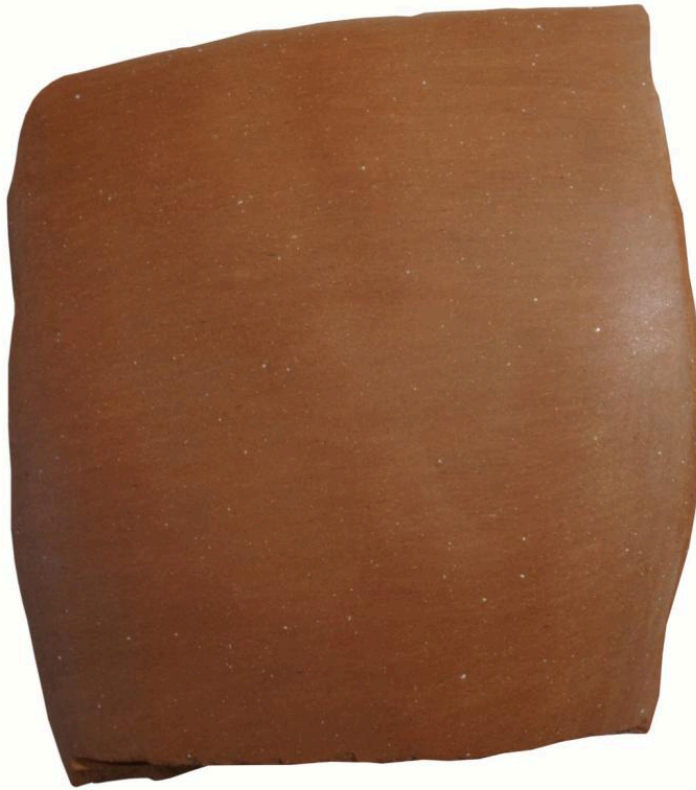
FIG 22B. TEST SHERD FROM THE EUBOEAN CLAY FIRED AT 1000° C/3 MIN IN A VSHR CONTROLLED FIRING. PHOTO BY NIKOS GERAKAKIS
