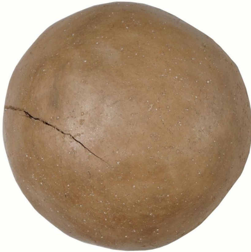
FIG 15B. POT FROM THE CRETAN CLAY THAT WAS FIRED IN THE UPDRAFT, WOOD-FIRING KILN (FOURTH FIRING). THE POT SHOWED ADVANCED LIME SPALLING. PHOTO BY NIKOS GERAKAKIS
