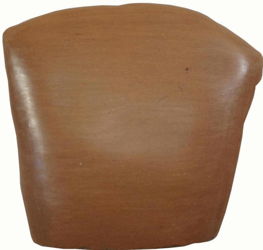
FIG 16B. TEST SHERD FROM THE EUBOEAN CLAY FIRED AT 800° C/3 MIN IN A FHR CONTROLLED FIRING. PHOTO BY NIKOS GERAKAKIS
