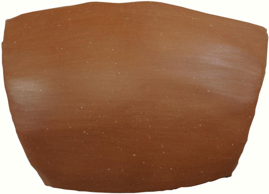
FIG 16D. TEST SHERD FROM THE EUBOEAN CLAY FIRED AT 1000° C/3 MIN IN A FHR CONTROLLED FIRING. PHOTO BY NIKOS GERAKAKIS
