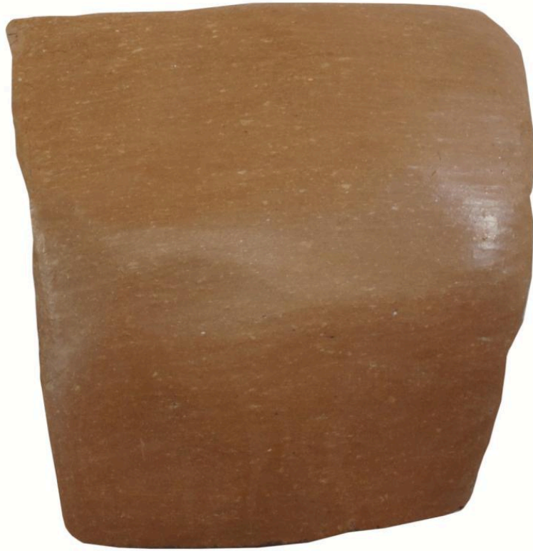
FIG 19B. TEST SHERD FROM THE CRETAN CLAY FIRED AT 800° C/1 H IN A FHR CONTROLLED FIRING. PHOTO BY NIKOS GERAKAKIS
