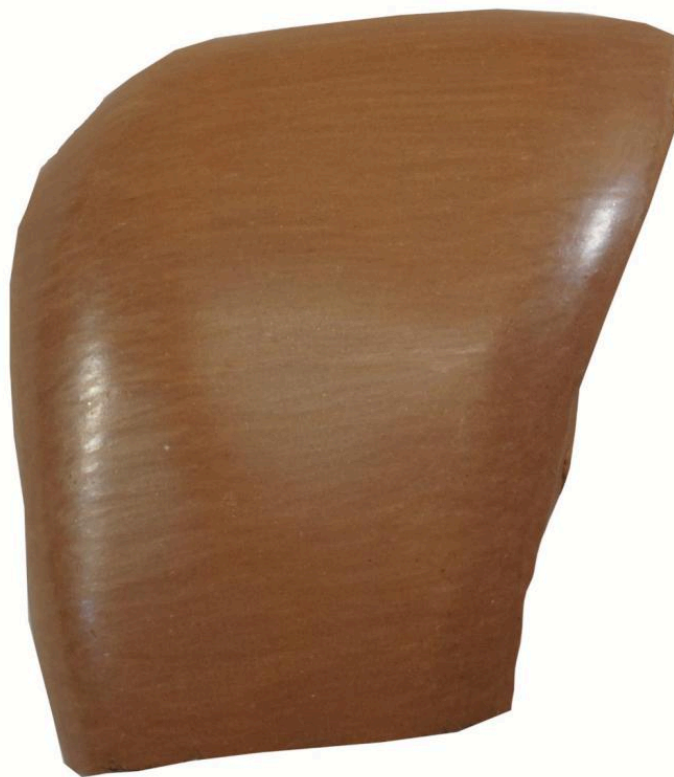
FIG 18A. TEST SHERD FROM THE EUBOEAN CLAY FIRED AT 700° C/1 H IN A FHR CONTROLLED FIRING. PHOTO BY NIKOS GERAKAKIS
